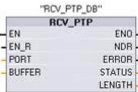
Input EN\_R controls the copy of a received message to the BUFFER.
