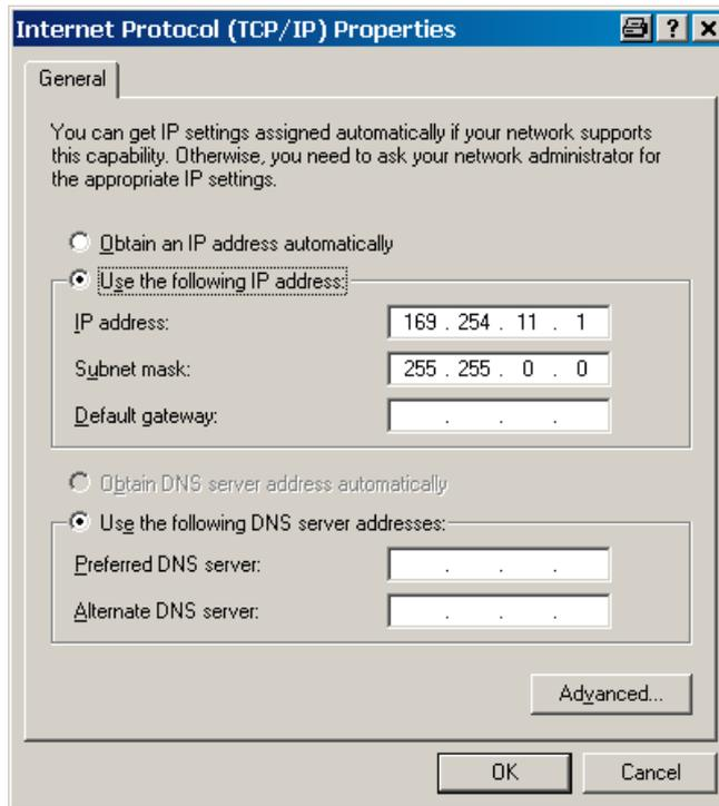
Figure 5-1 Example: IPv4 address of the PG/PC
