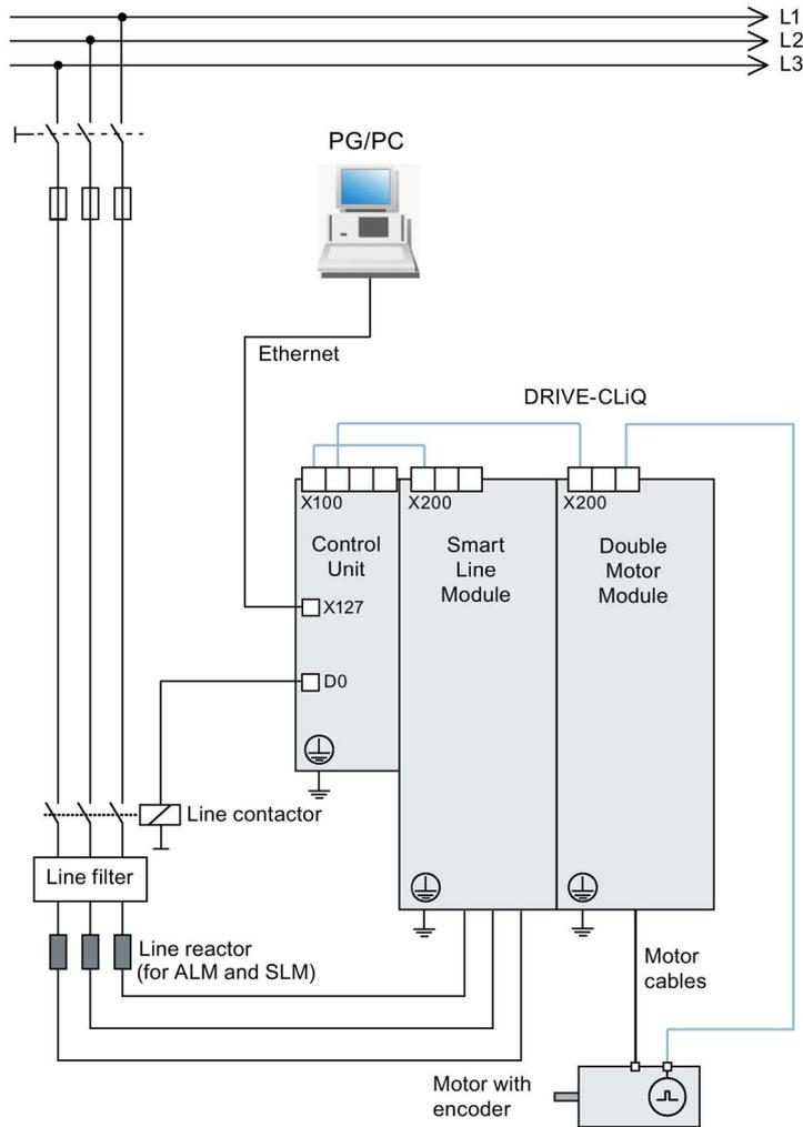
Figure 4-2 Wiring principle
