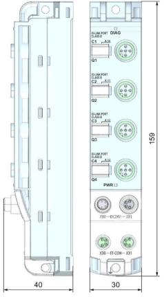
The following figure shows the dimension drawing of the CM 4xIO-Link 4xM12 communication module in front and side view.
