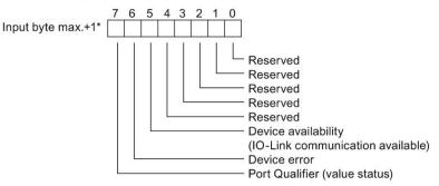
\* The PQI byte is always located after the last input byte of the port.
