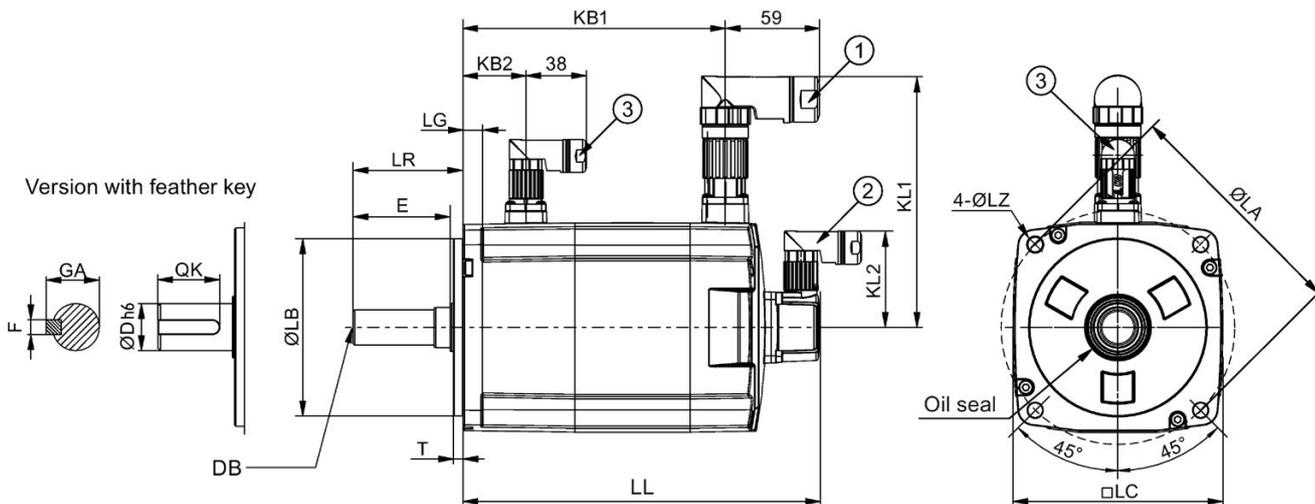
**High inertia servo motor with angular connectors, with the absolute encoder**
