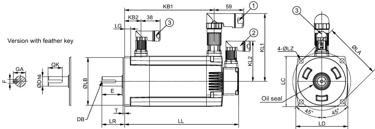
Low inertia servo motor, shaft height: 50 mm, with angular connectors
