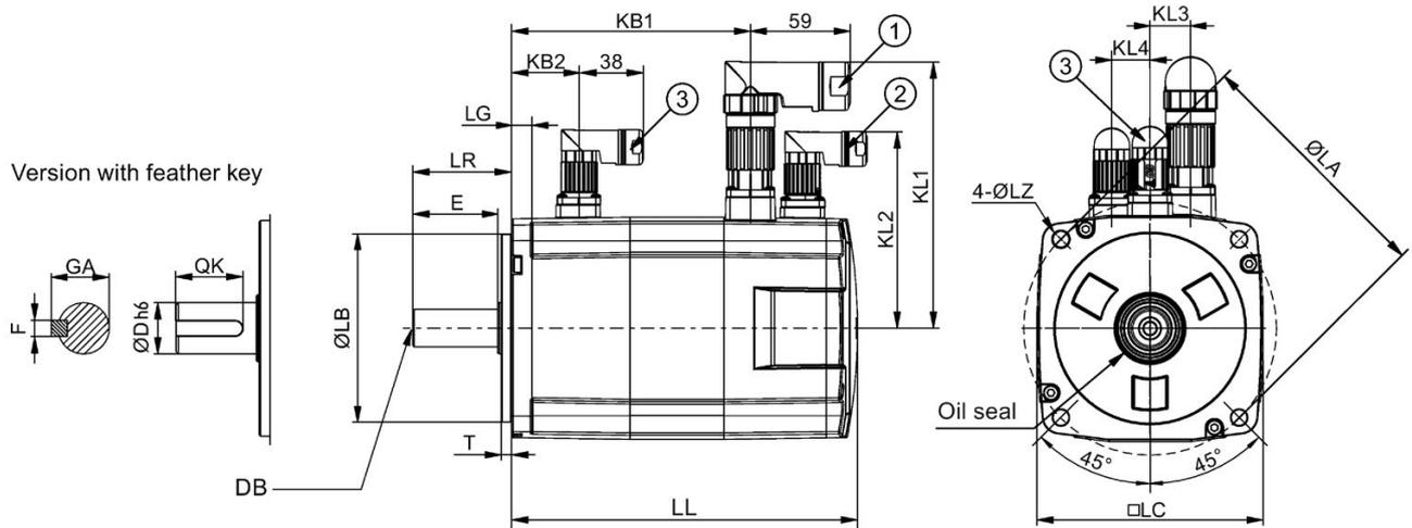
High inertia servo motor with angular connectors, with the incremental encoder
