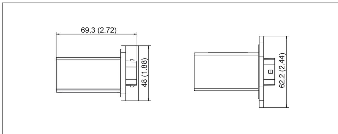
Figure 13-11 Dimension drawing, DRIVE-CLiQ cabinet gland
