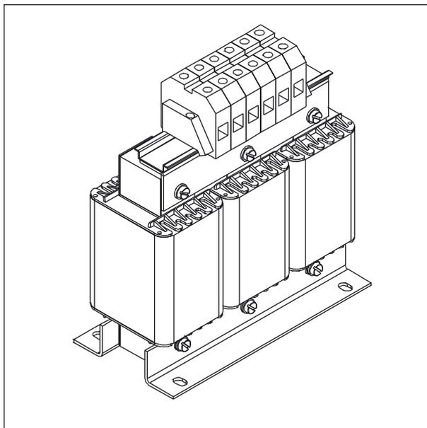
Figure 4-35 Line reactor for Basic Line Module (40 kW)
