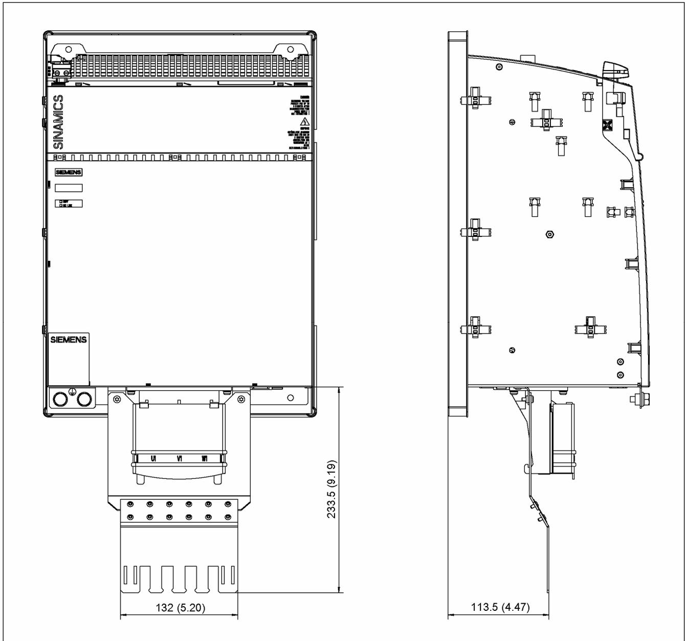
Dimension drawing, shield connecting plate on a 300 mm component with cold plate
