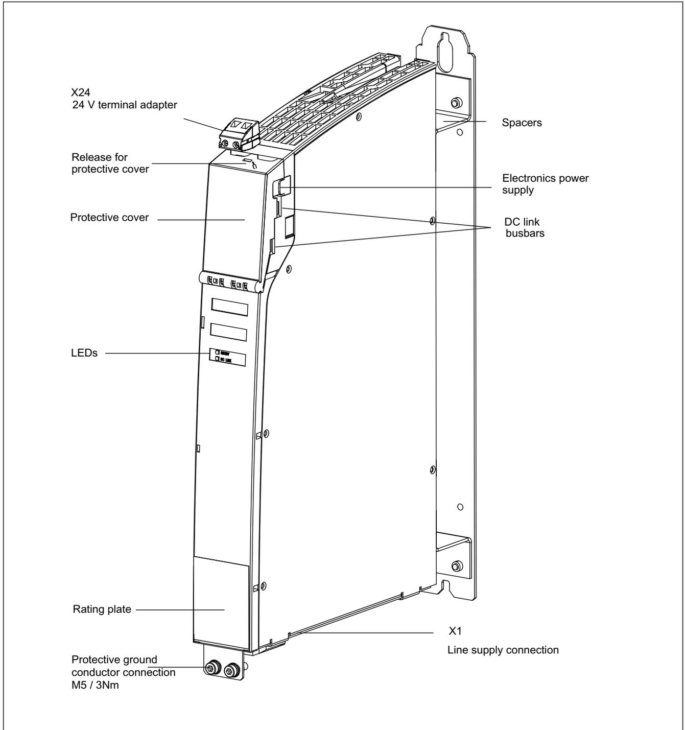
Figure 11-11 Interface description: control supply module
