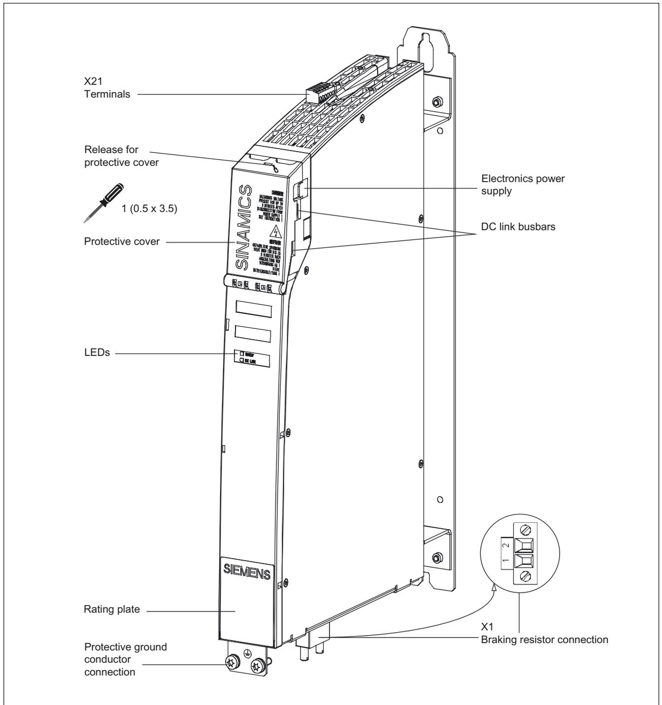
Figure 11-1 Interface description of braking module
