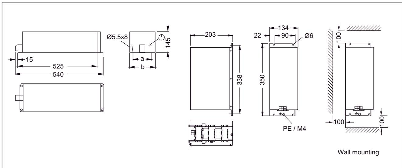
Figure 6-19 Dimension drawing: Braking resistor 7.5 kW and 15 kW
