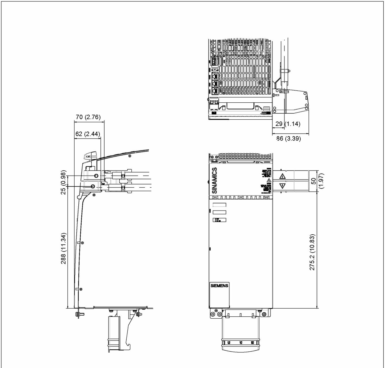
Figure 13-9 Dimension drawing, 150 mm components with DC link adapter for two-row configuration 35 mm<sup>2</sup> to 95 mm<sup>2</sup>
