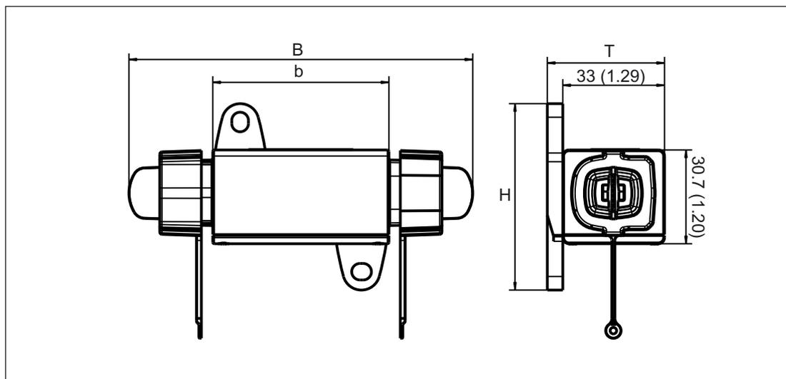
Figure 13-15 Dimension drawing, DRIVE-CLiQ coupling
