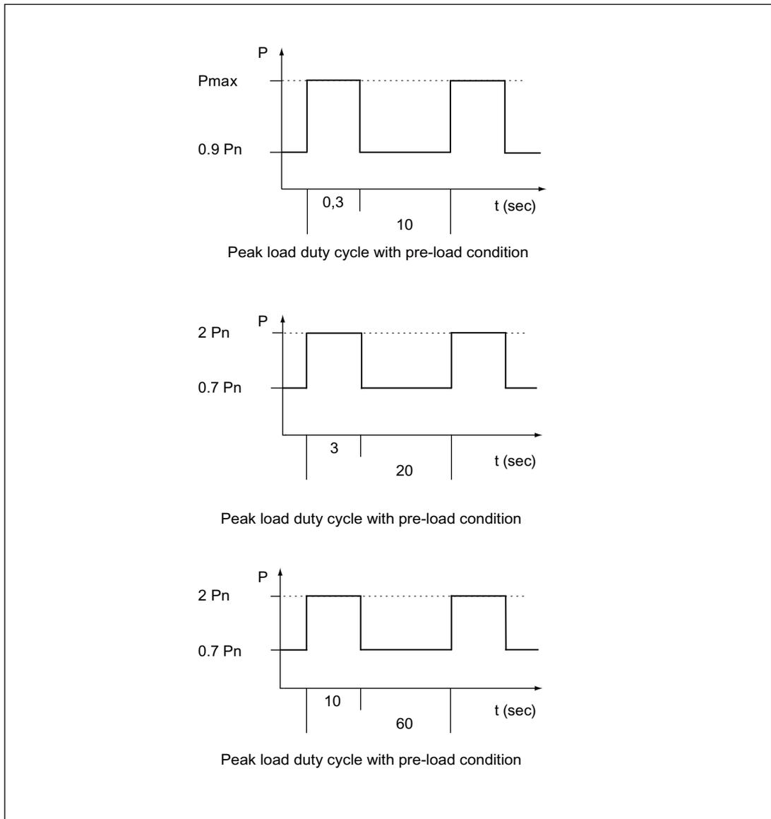
Figure 6-12 Infeed duty cycles for 20 kW and 40 kW Basic Line Modules
