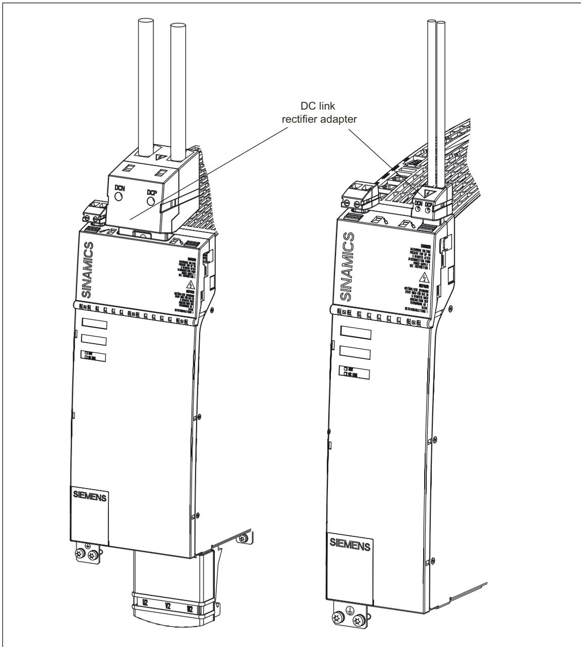
Figure 13-5 150 mm components with DC link rectifier adapter for 35 mm<sup>2</sup> to 95 mm<sup>2</sup> and 100 mm components with DC link rectifier adapter for 4 mm<sup>2</sup> to 10 mm<sup>2</sup>
