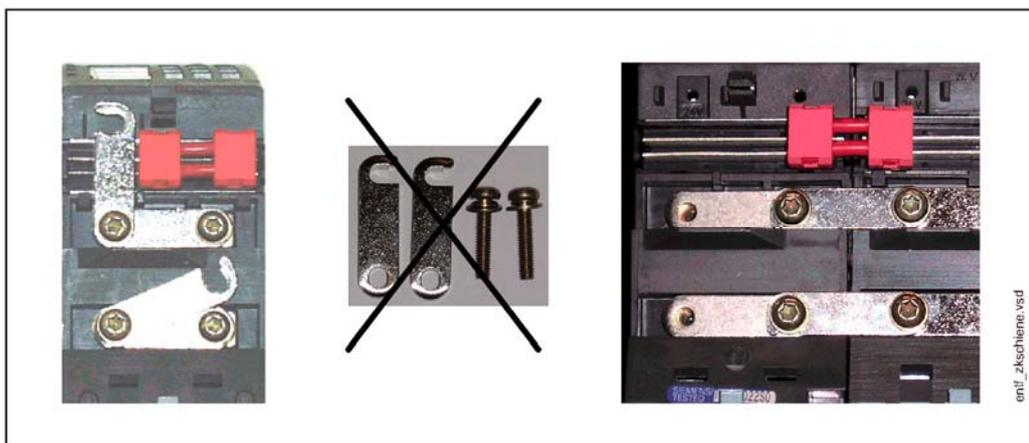
Figure 14-3 Removing the DC link bridges (multi-tier configuration)
