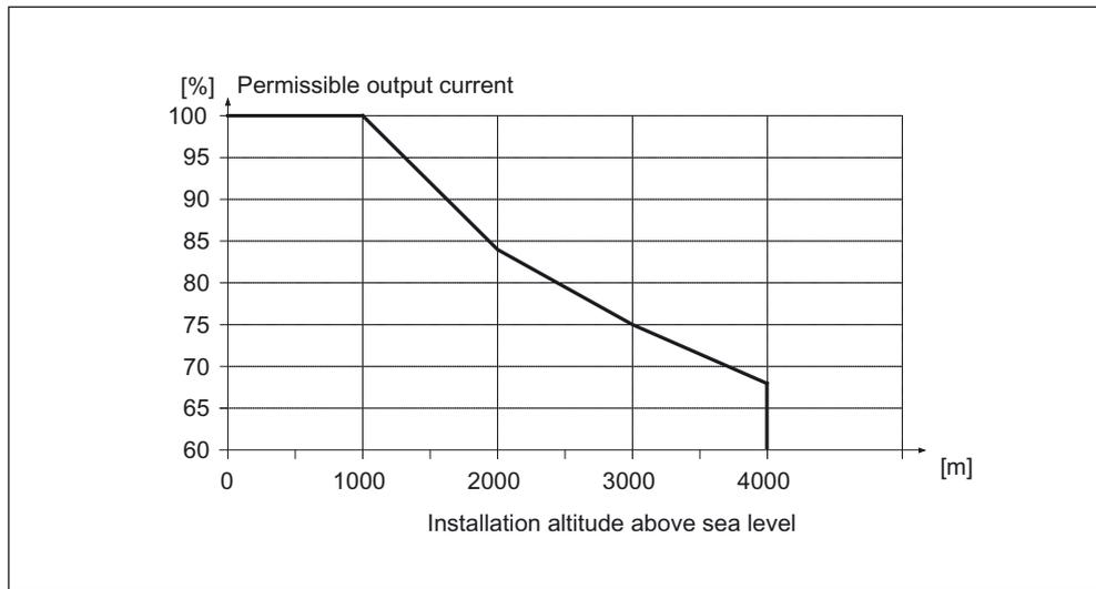
Figure 8-17 Derating as a function of the site altitude
