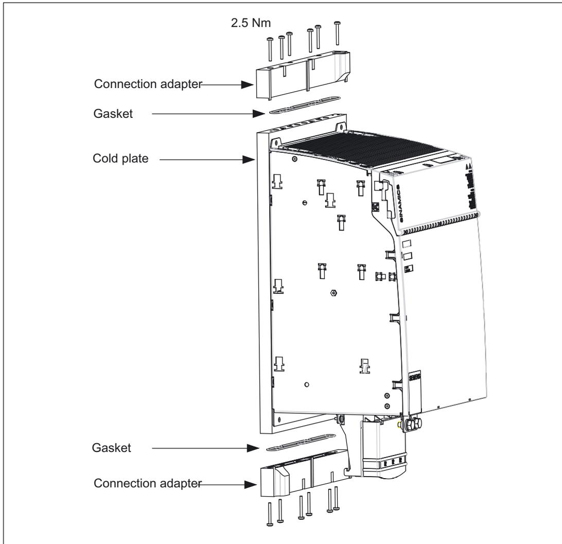
Figure 9-3 Connection method
