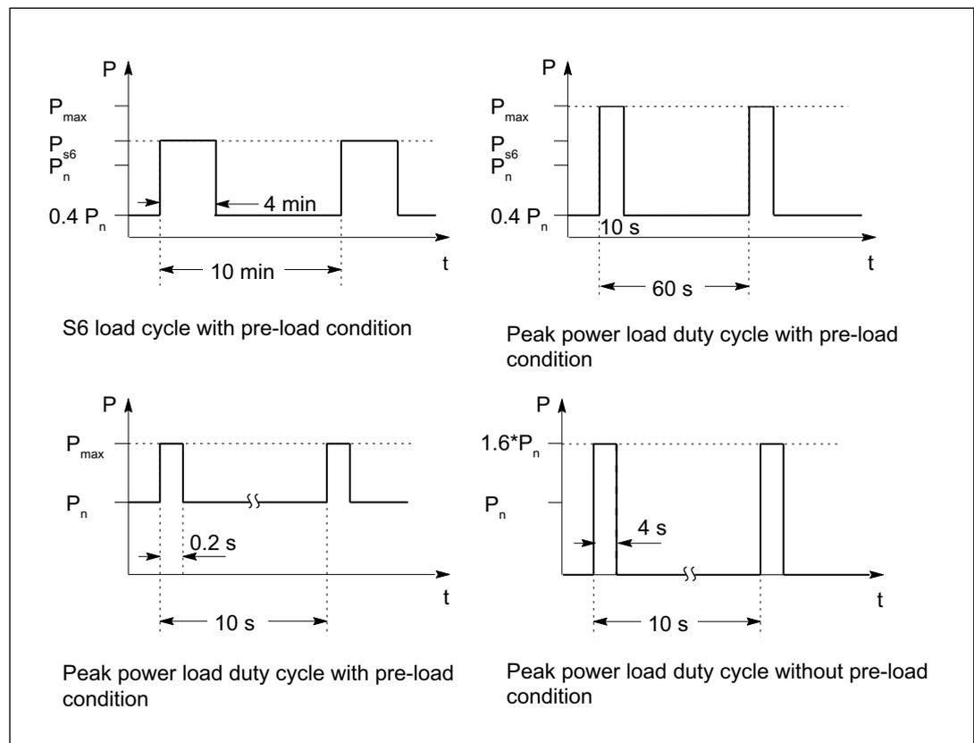
Figure 5-6 Rated duty cycles of Active Line Modules
