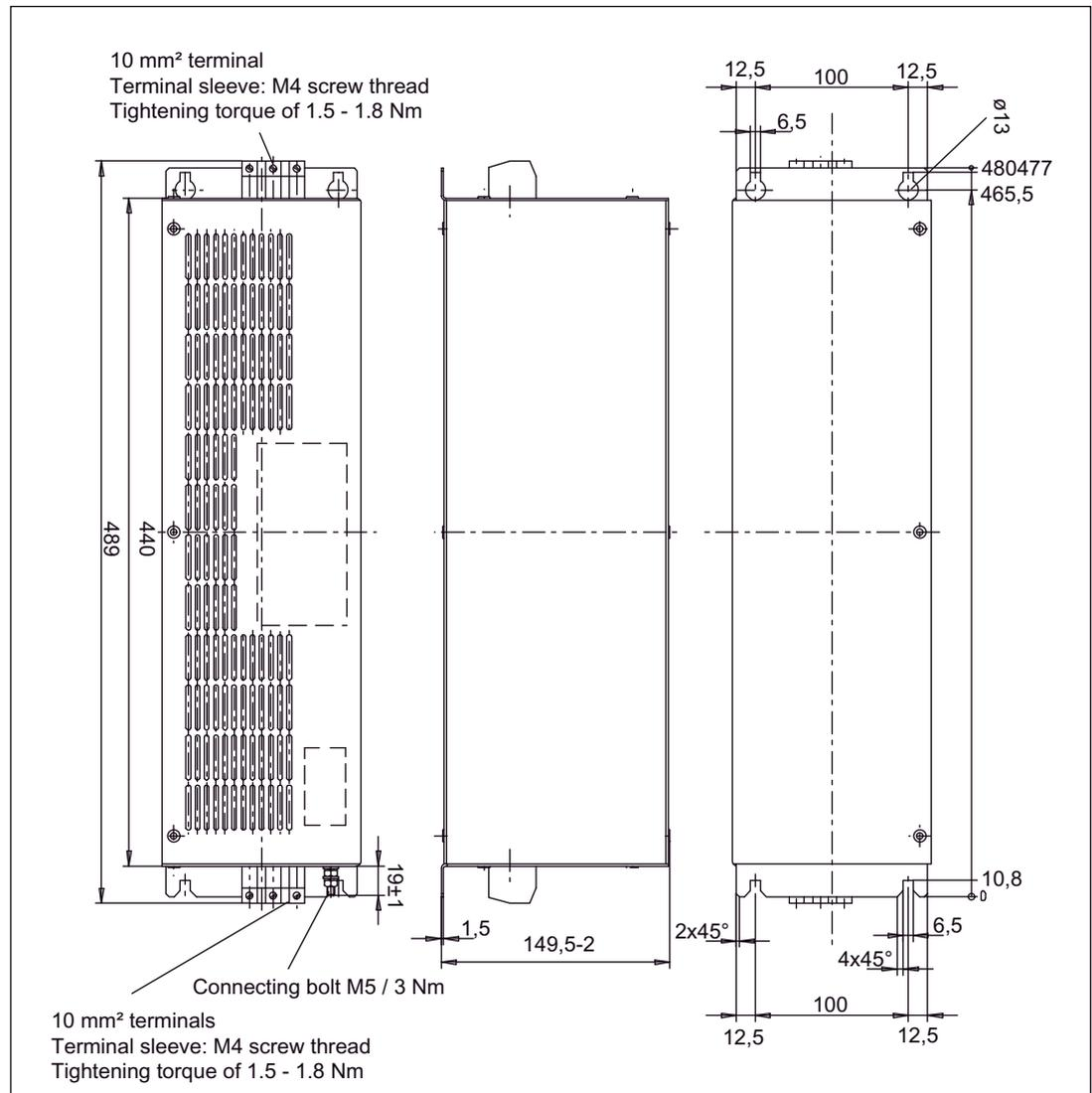
Figure 4-11 Dimension drawing: 16 kW Wideband Line Filter for Active Line Modules
