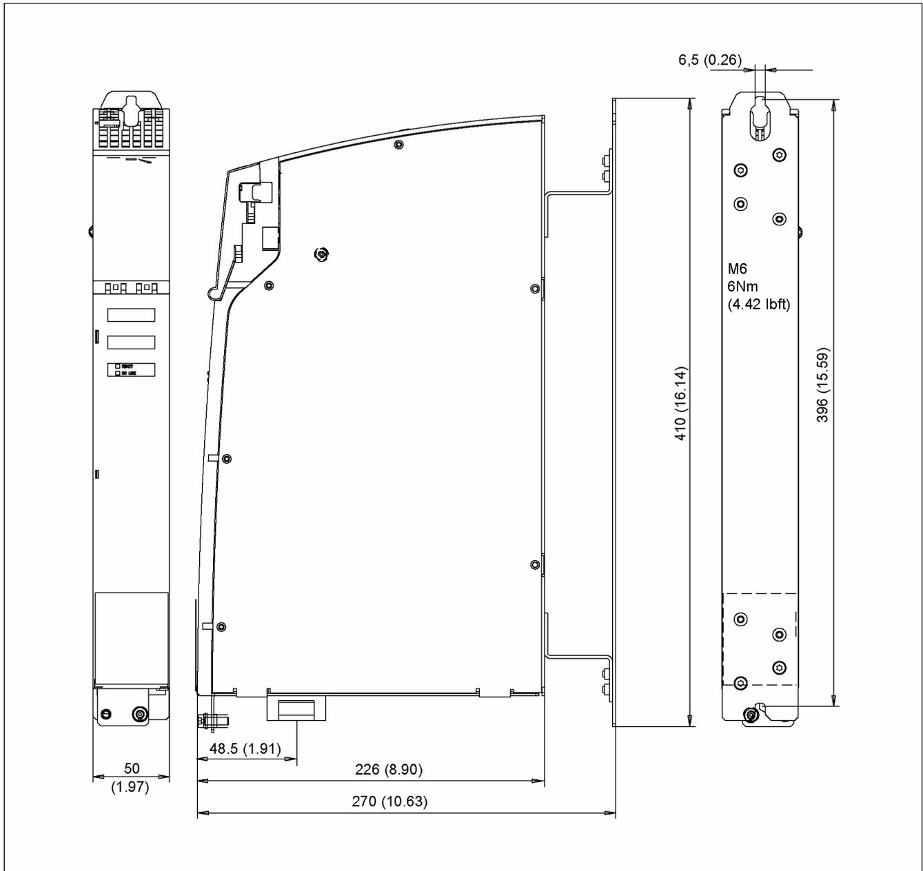
Figure 11-13 Dimension drawing of the Control Supply Module
