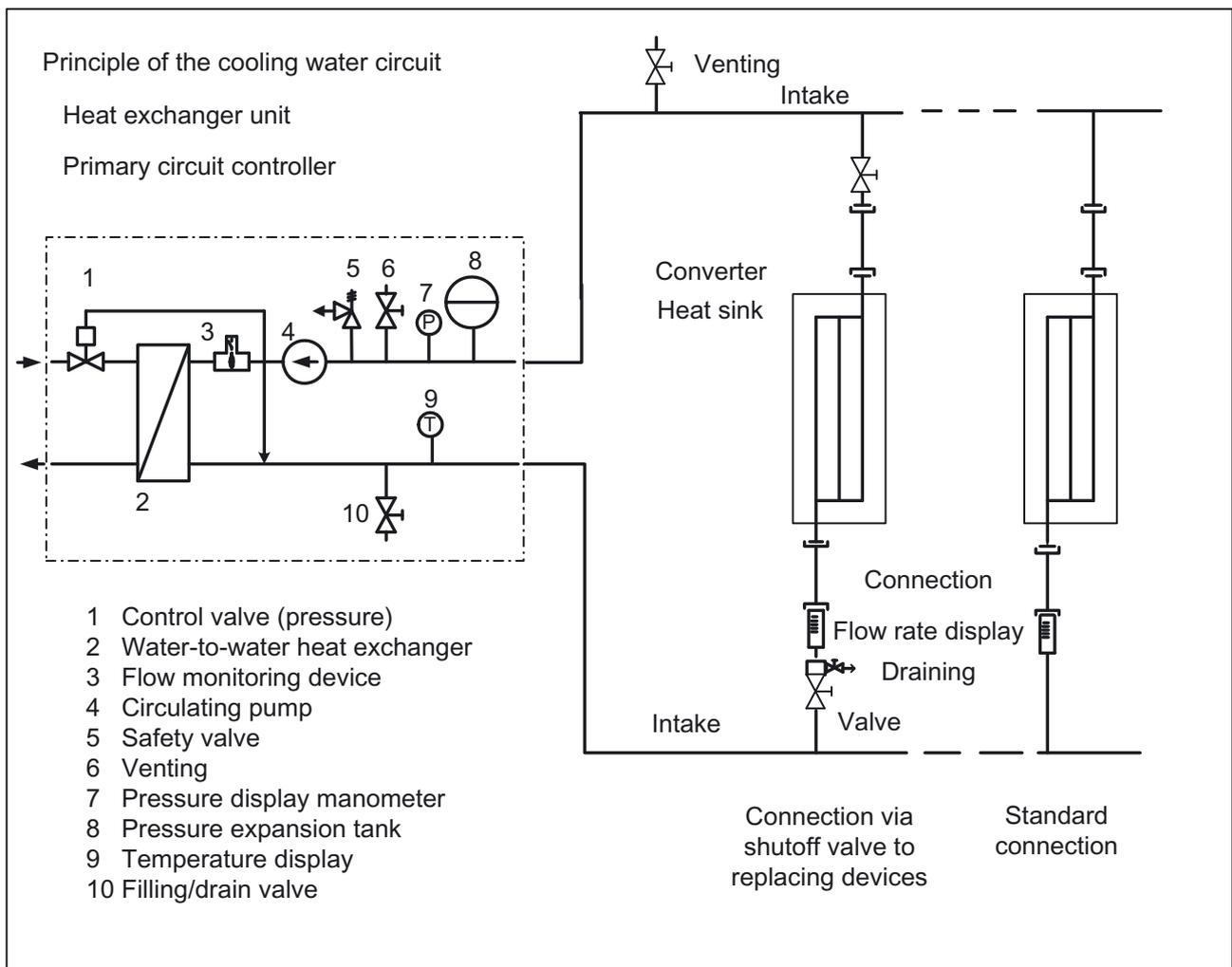
Figure 3-1 Principle of the cooling water circuit
