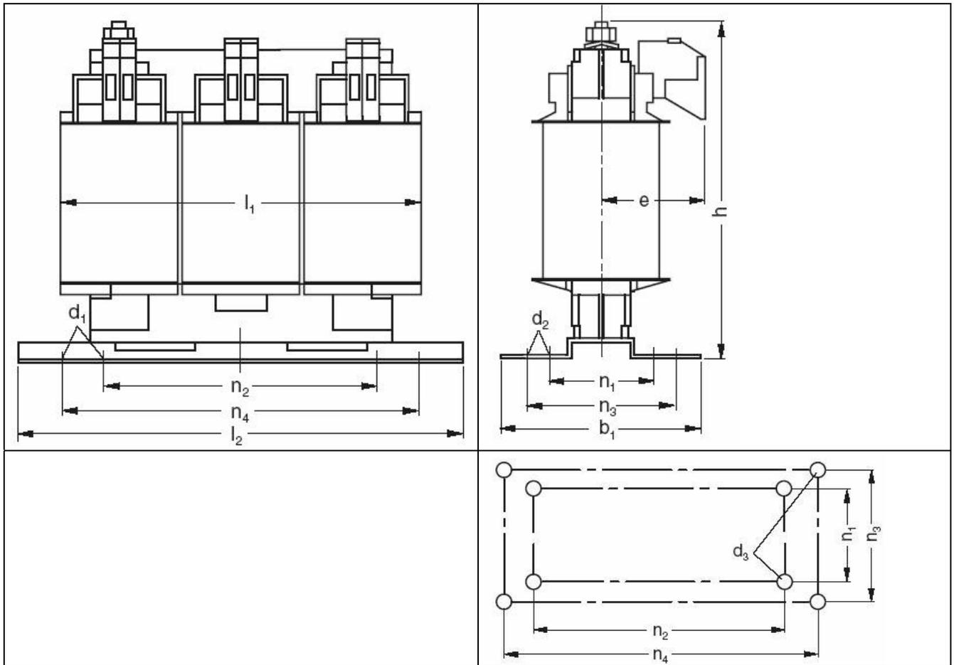
Table 12-3 Dimensions of motor reactors, all data in mm and (inches)
