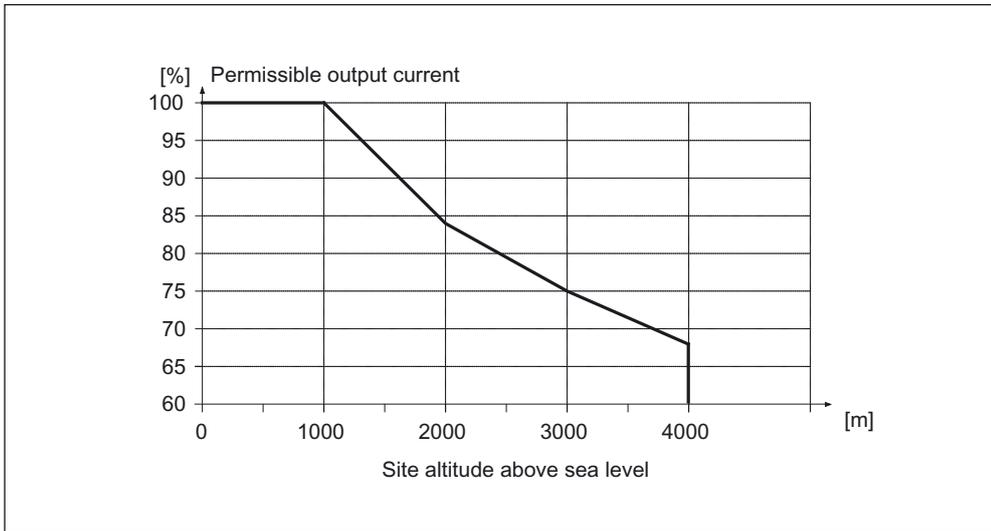
Figure 5-8 Derating as a function of the site altitude
