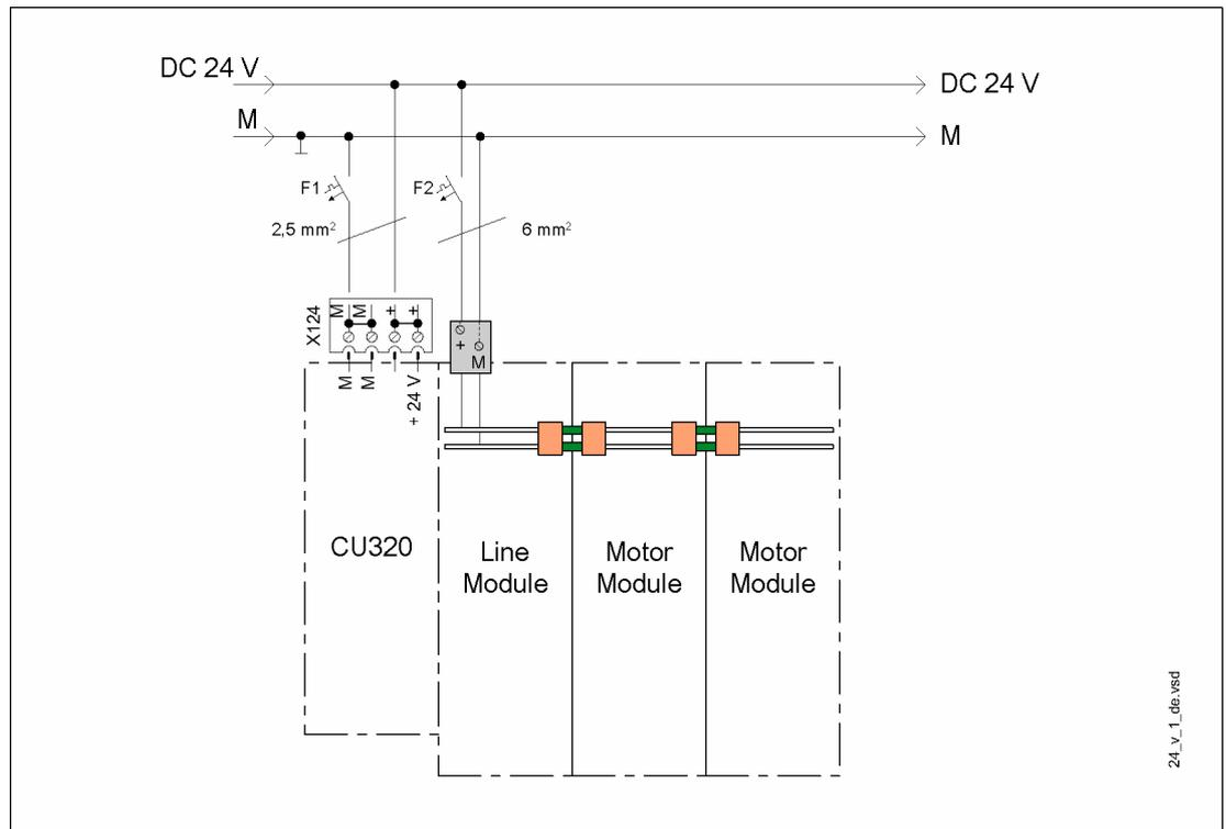
Figure 14-1 Example of 24 V DC fuse protection
