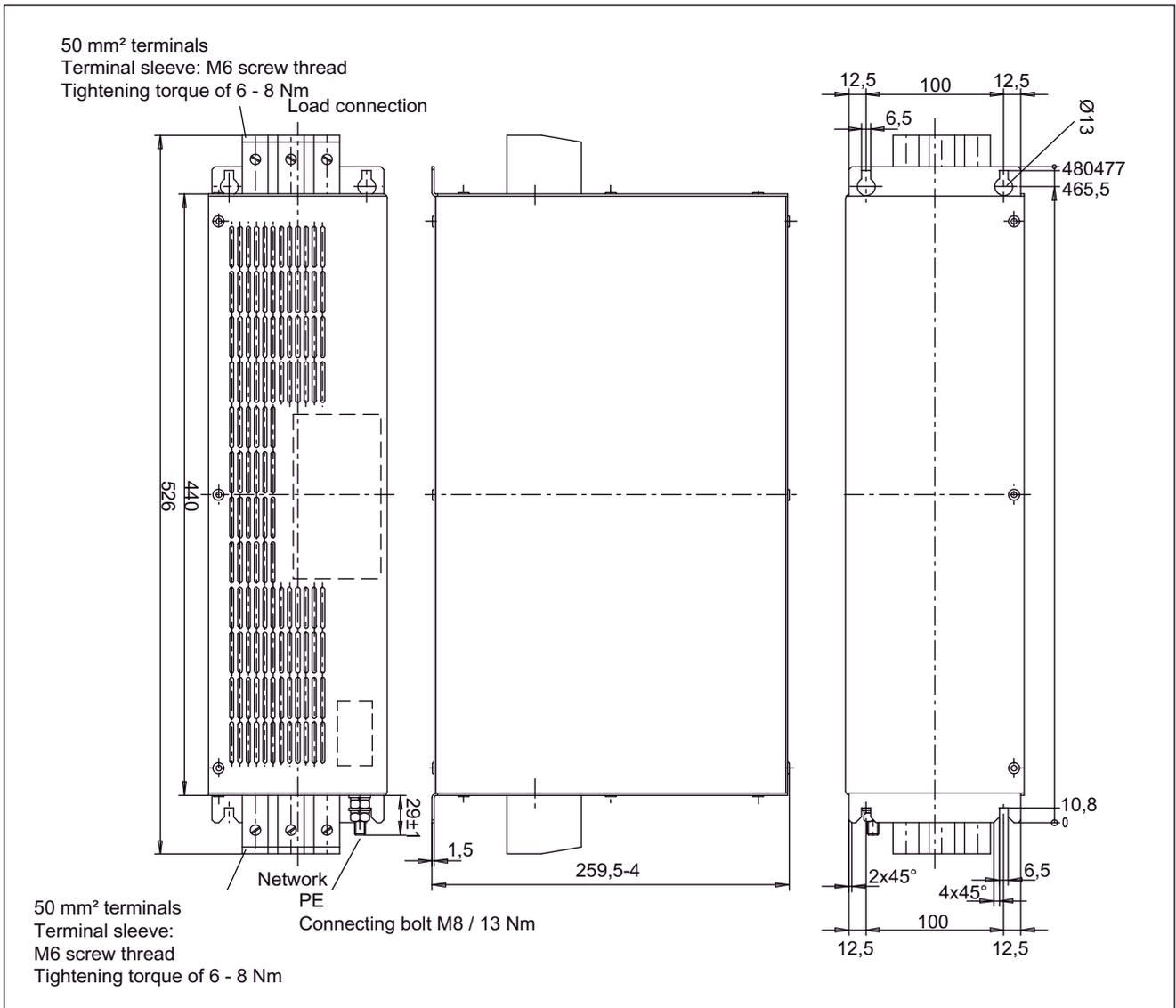
Figure 4-13 Dimension drawing: 55 kW Wideband Line Filter for Active Line Modules
