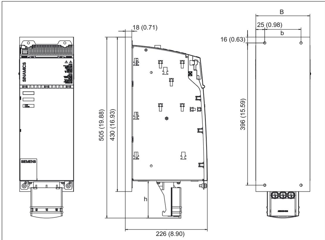
Figure 8-6 Dimension drawing, Motor Module with cold plate 45 A, 60 A and 85 A
