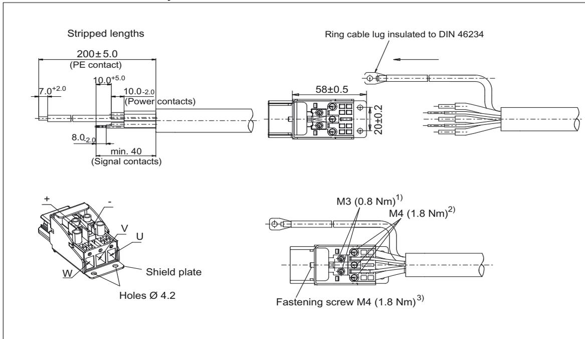
Figure 14-9 Setting up and installing the power supply connector (X1/X2)
