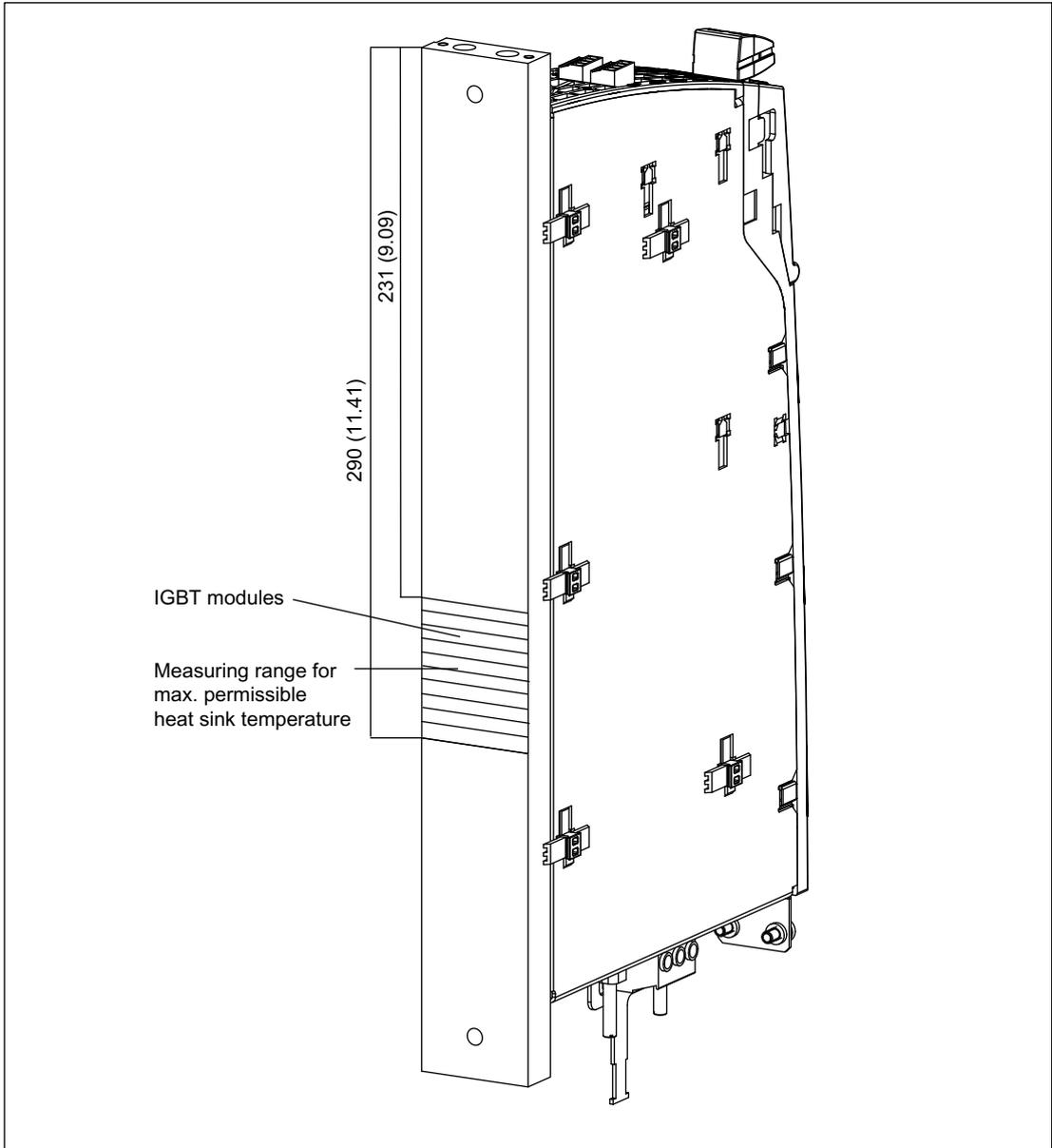
Figure 7-10 Measuring range for max. permissible heat sink temperature for a Smart Line Module
