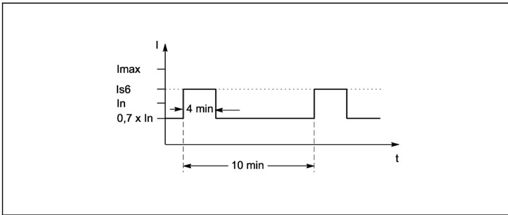
Figure 8-11 S6 current duty cycle with prior loading
