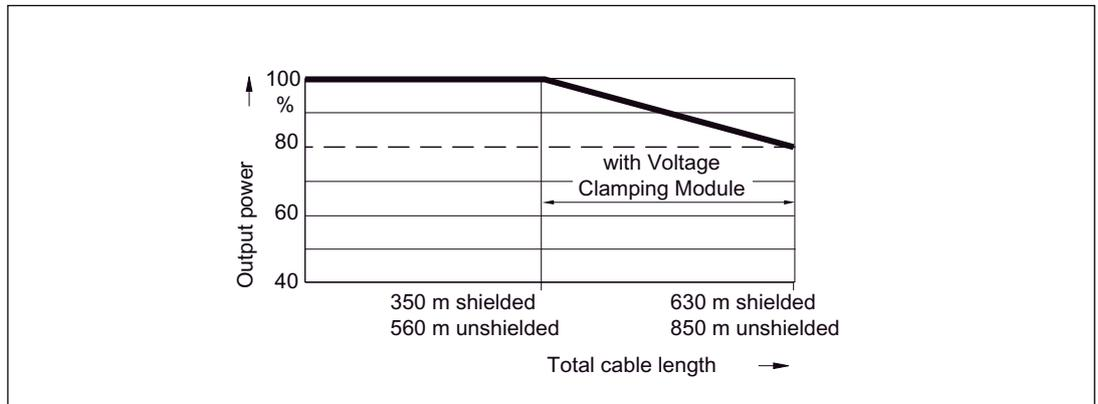
Figure 7-9 Output power as a function of total cable length
