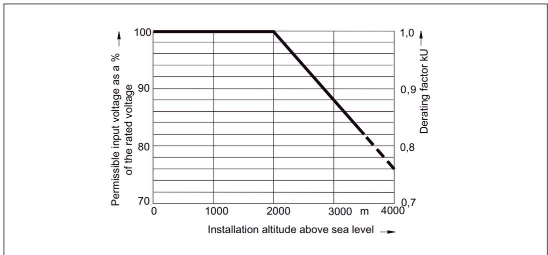
Figure 8-18 Voltage derating as a function of the installation altitude
