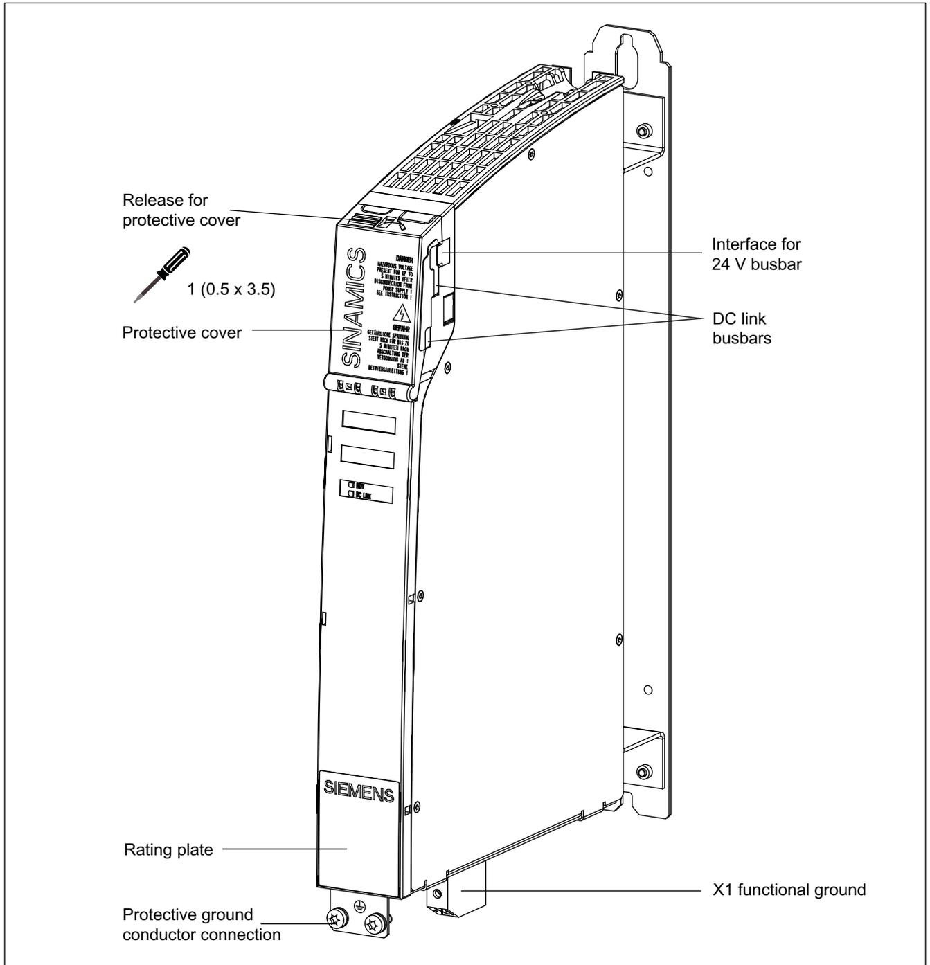
Figure 11-14 Interface description: Voltage Clamping Module
