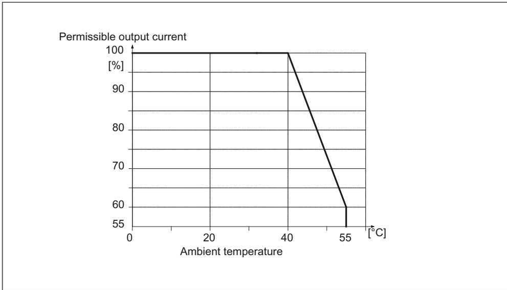
Figure 8-15 Derating as a function of the ambient temperature
