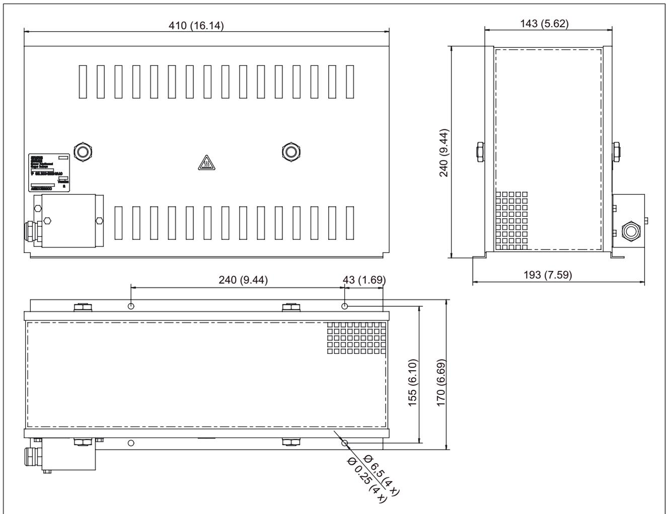
Figure 11-6 Dimension drawing: Braking resistor 1.5 kW / 100 kW
