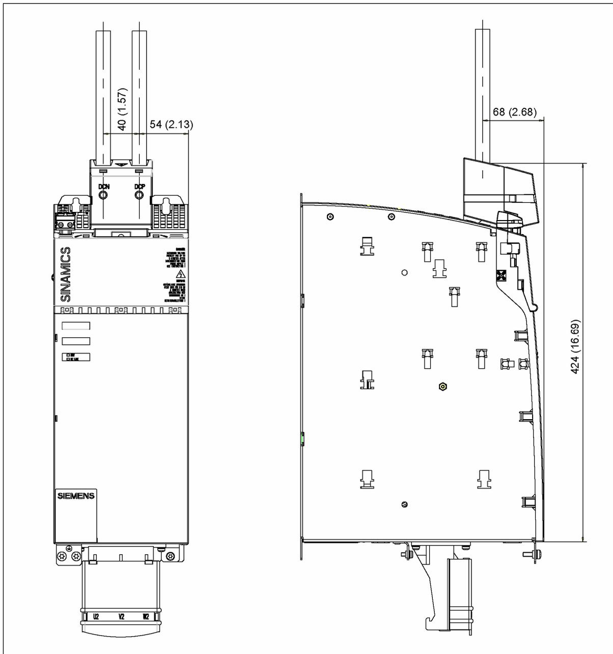
Figure 13-7 Dimension drawing, 150 mm components with DC link rectifier adapter for 35 mm<sup>2</sup> to 95 mm<sup>2</sup>
