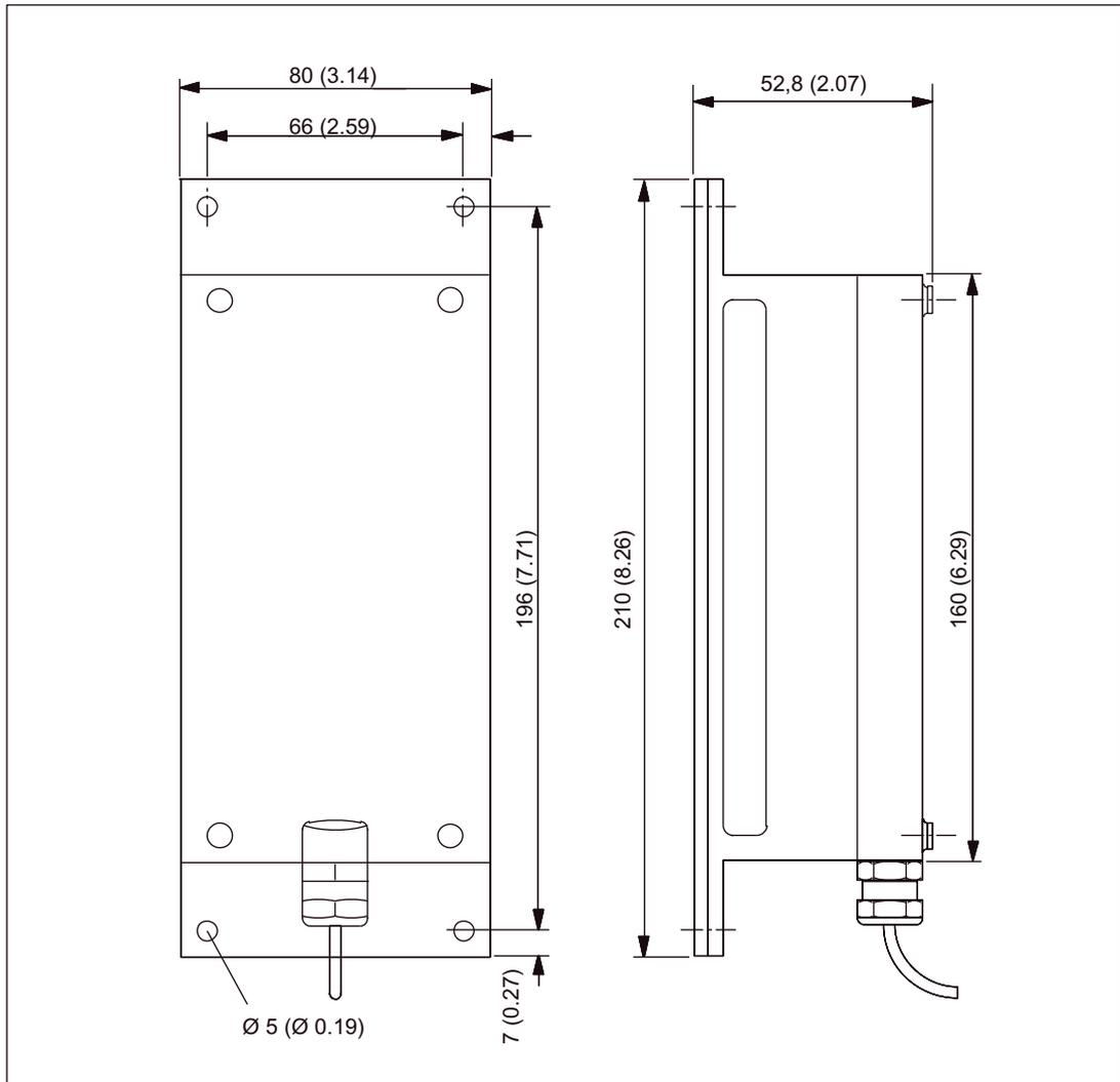
Figure 11-5 Dimension drawing: Braking resistor 0.3 kW / 25 kW
