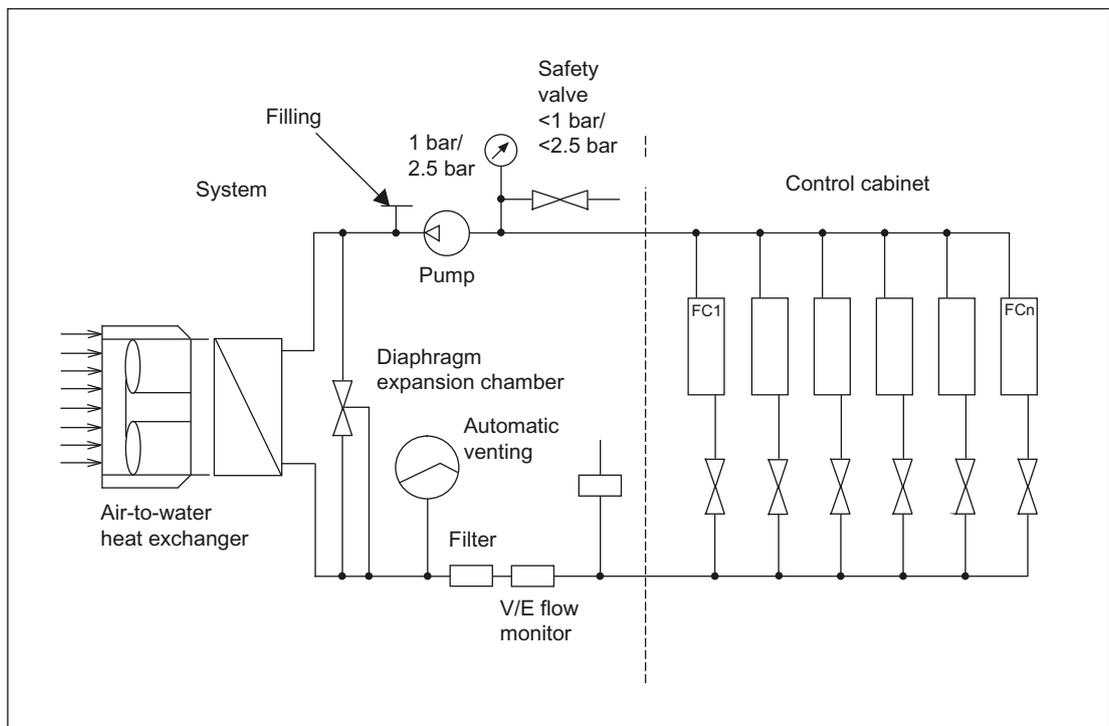
Figure 10-2 Air-to-water heat exchanger
