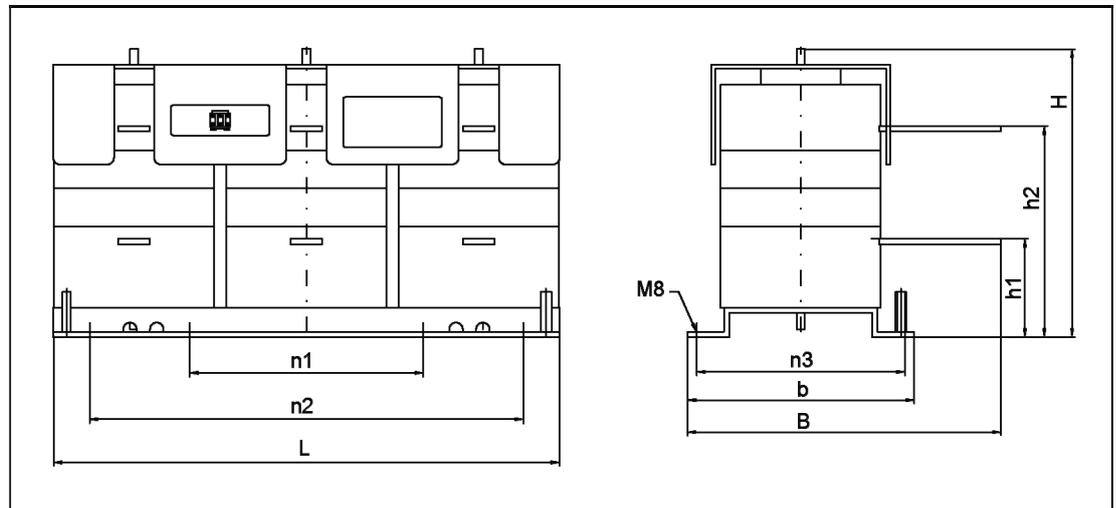
Figure 4-29 Dimension drawing: line reactor for Active Line Modules (as of 80 kW)
