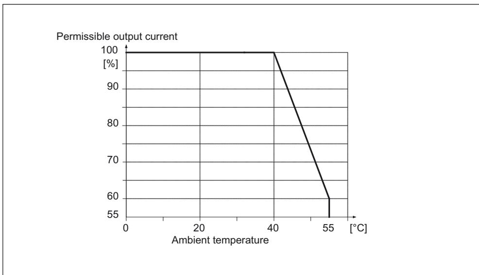
Figure 7-6 Derating as a function of the ambient temperature
