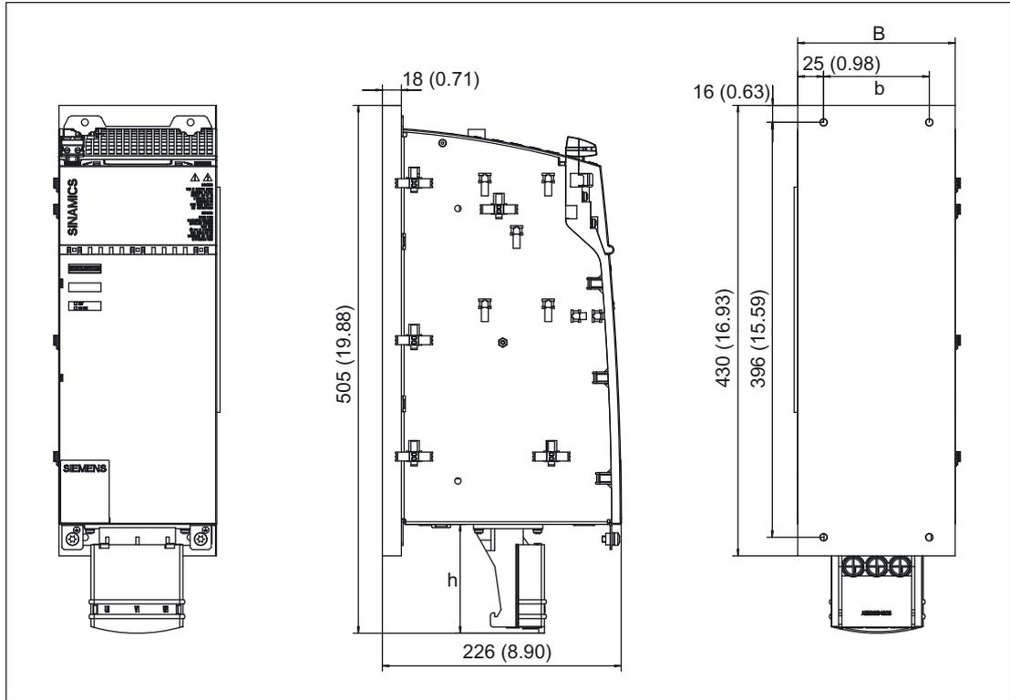
Figure 5-4 Dimension drawing, Active Line Module with cold plate (36 kW, 55 kW, 80 kW, and 120 kW)
