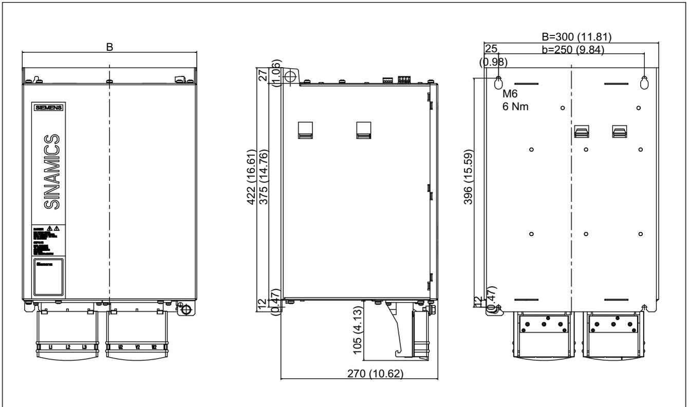
Figure 4-25 Dimension drawing: Active Interface Module (80 kW and 120 kW)
