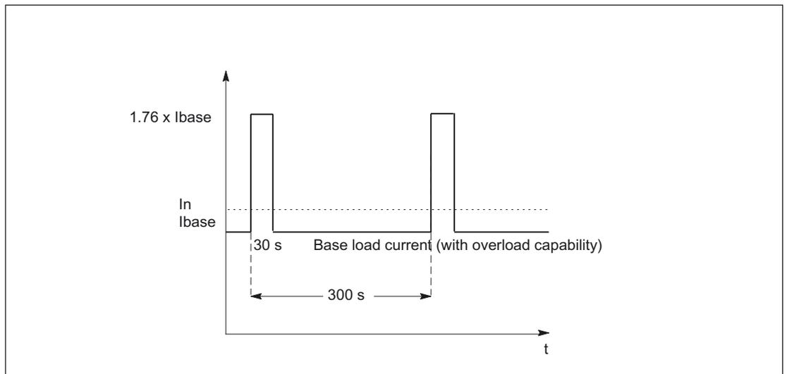
Figure 8-14 Current duty cycle with pre-loading
