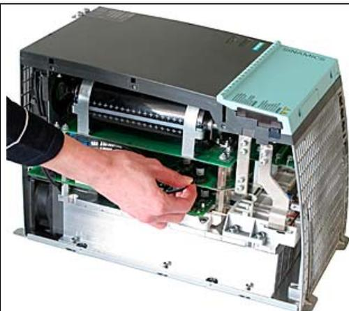
Pull the first fan cable by pressing it slightly
