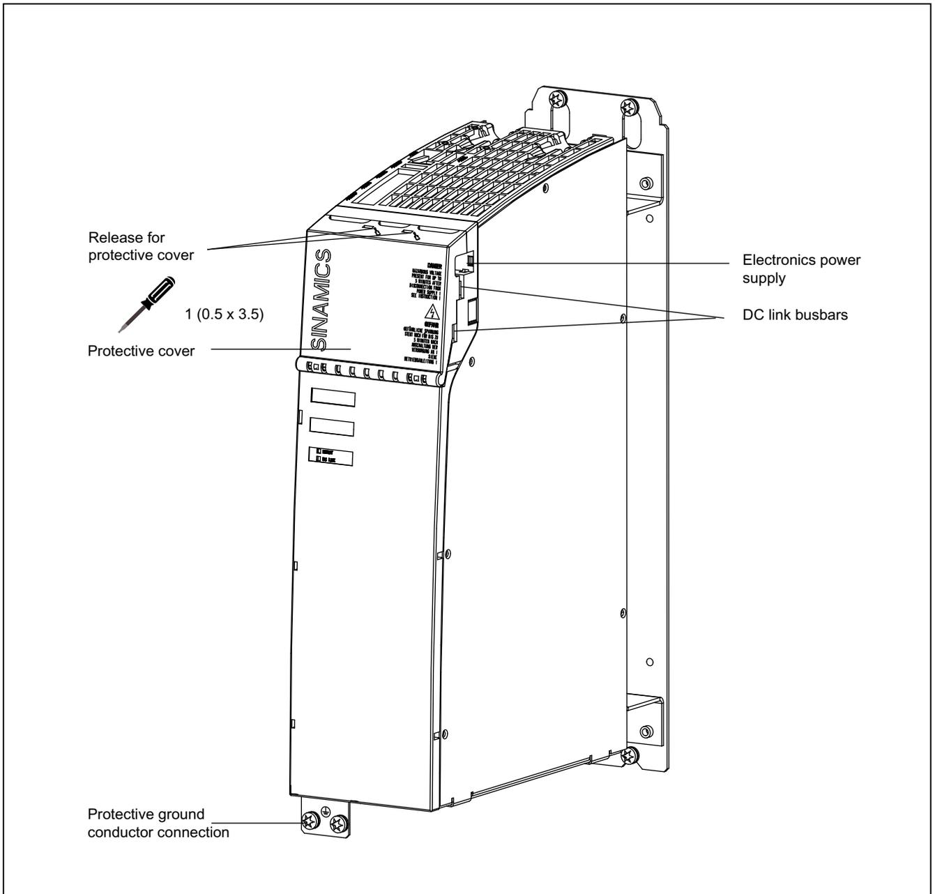
Figure 11-8 Interface description of the capacitor module
