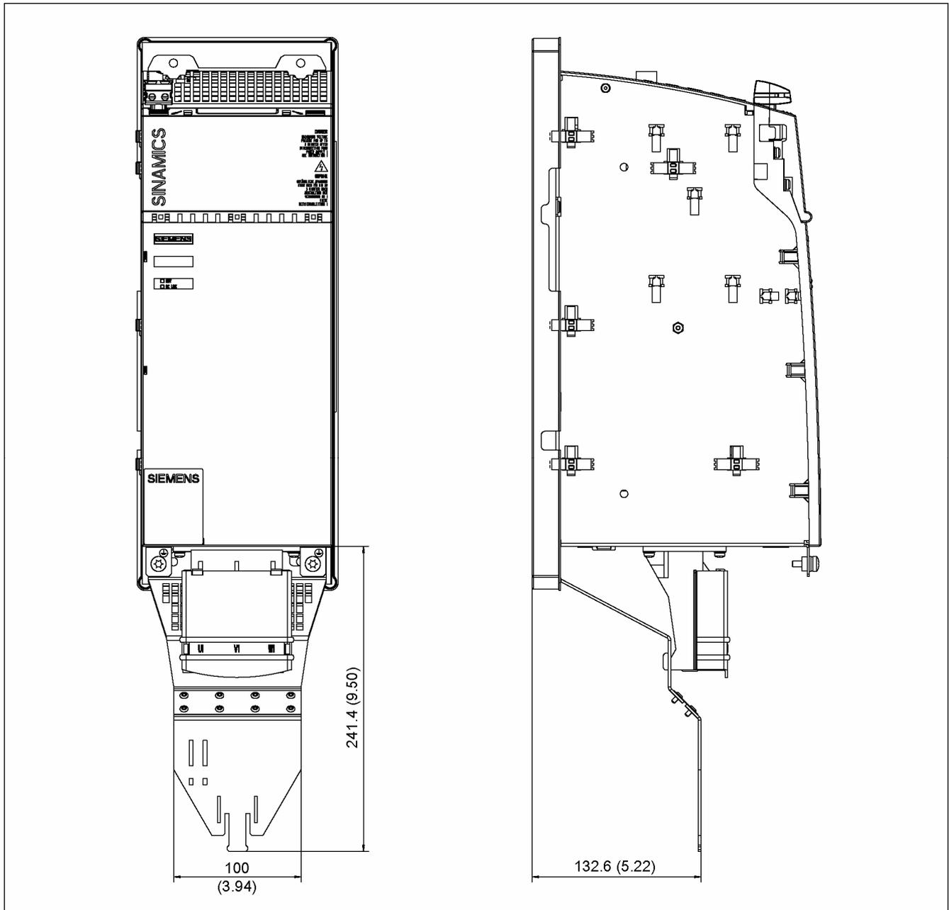
Figure 13-3 Dimension drawing, shield connecting plate on a 150 mm component with cold plate
