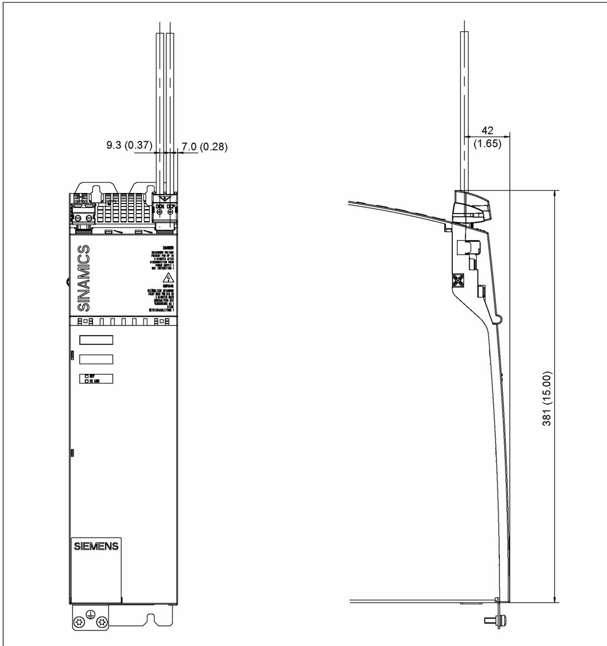
Figure 13-6 Dimension drawing, 100 mm components with DC link rectifier adapter for 0.5 mm<sup>2</sup> to 10 mm<sup>2</sup>
