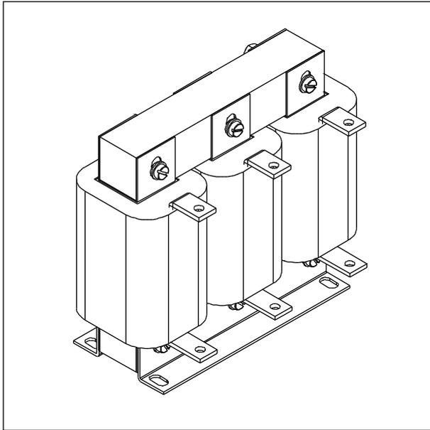
Figure 4-36 Line reactor for Basic Line Module (100 kW)
