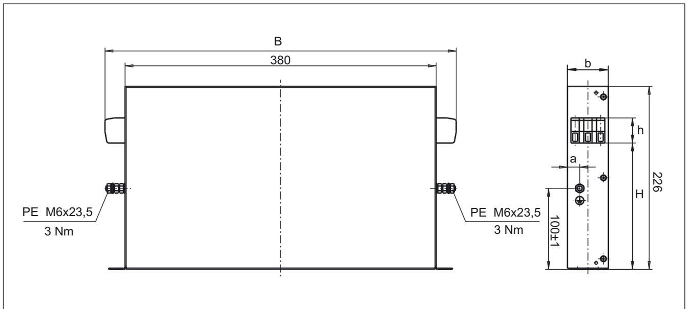
Figure 4-20 Dimension drawing: Basic Line Filter for Smart Line Modules (16 kW and 36 kW)
