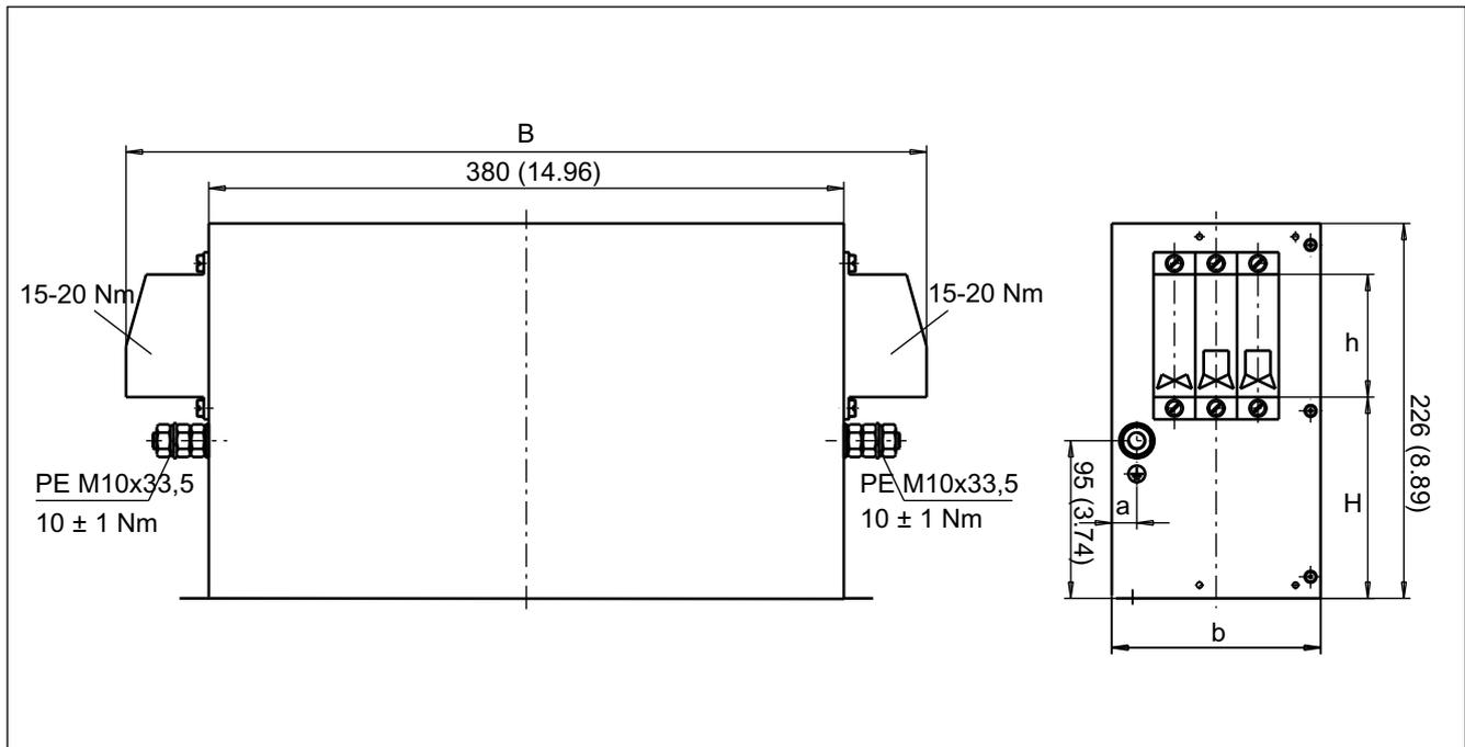
Figure 4-9 Dimension drawing: 80 kW and 120 kW Basic Line Filter
