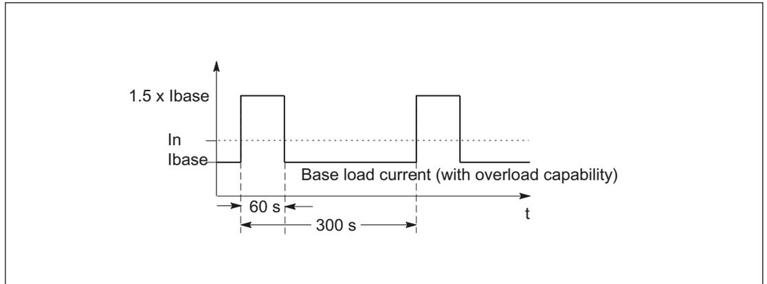
Figure 8-13 Current duty cycle with pre-loading
