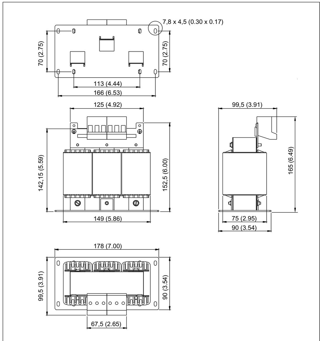
Figure 4-37 Dimension drawing: Line reactor for Basic Line Module (20 kW)
