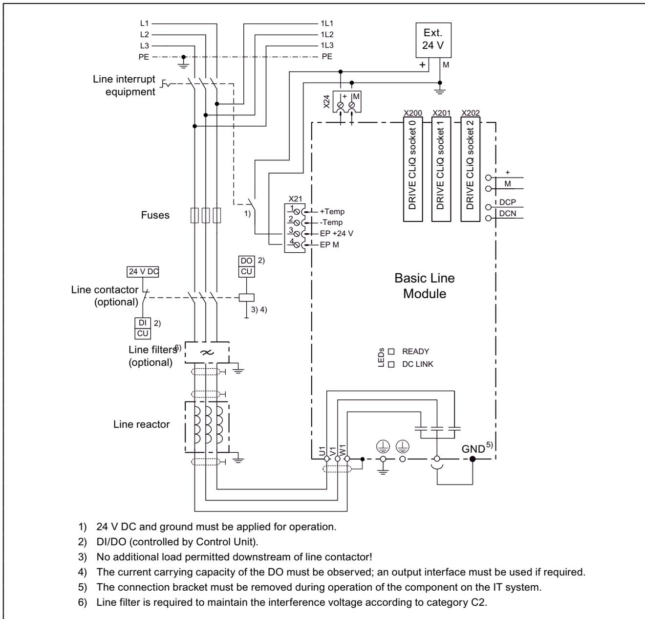
Figure 6-5 Connection example: Basic Line Module (100 kW)
