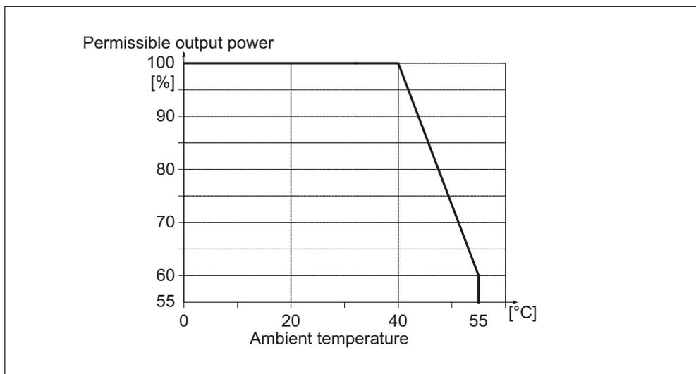
Figure 6-15 Derating as a function of the ambient temperature
