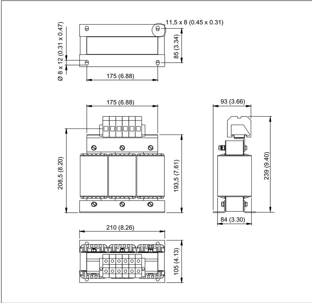
Figure 4-38 Dimension drawing: Line reactor for Basic Line Module (40 kW)
