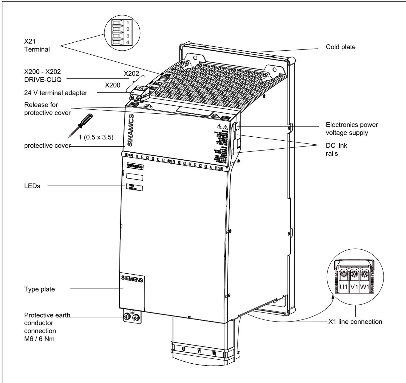
Figure 6-3 Interface description: Basic Line Module with cold-plate cooling (100 kW)
