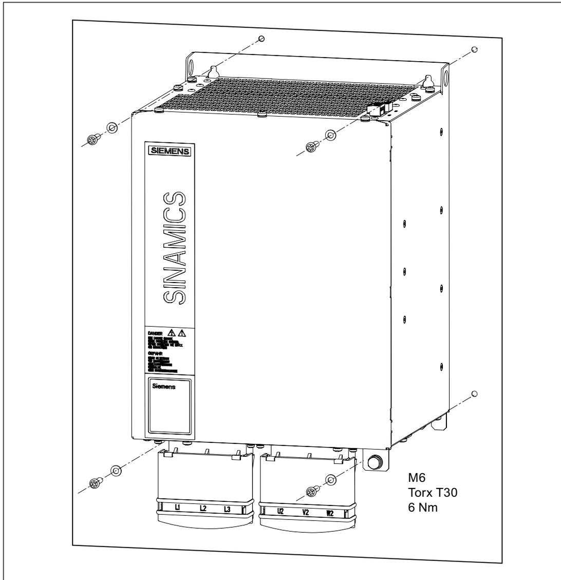
Figure 4-26 Mounting: Active Interface Module
