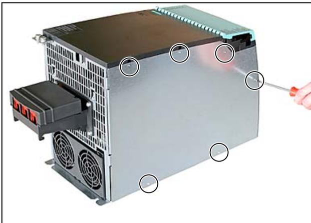
Open the right device cover by loosening the six marked screws
