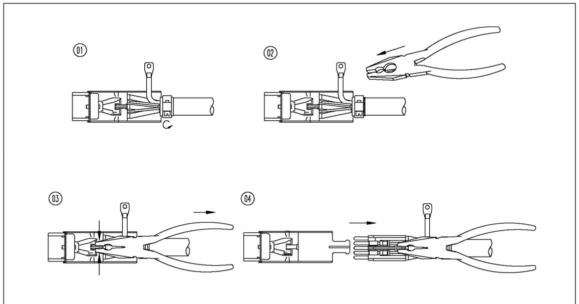
Figure 14-7 Removing the motor connector
