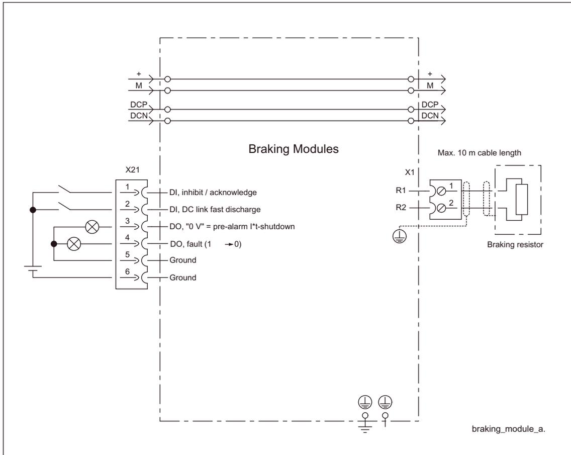
Figure 11-2 Example connection of Braking Module
