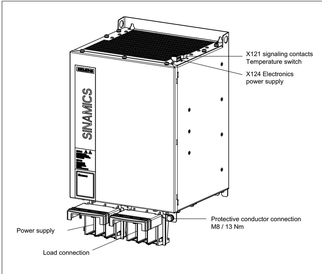
Figure 4-22 Interface description: Active Interface Module (80 kW and 120 kW)
