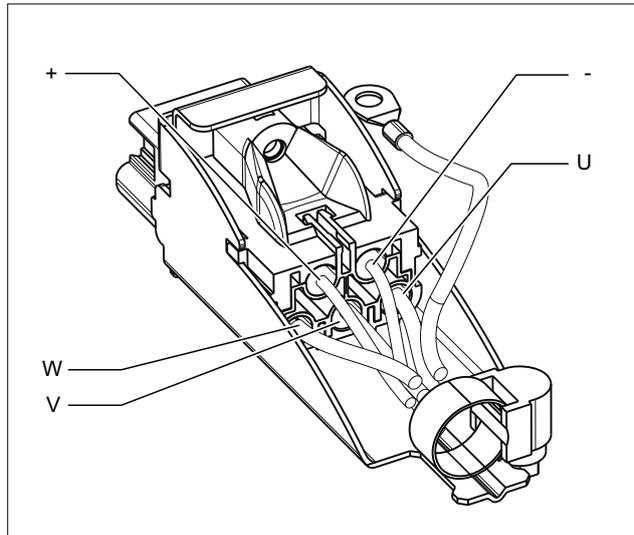
Figure 14-6 Motor connector
