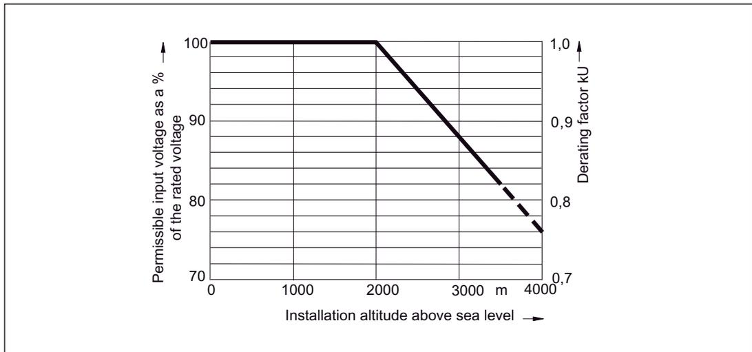
Figure 7-8 Voltage derating as a function of the installation altitude
