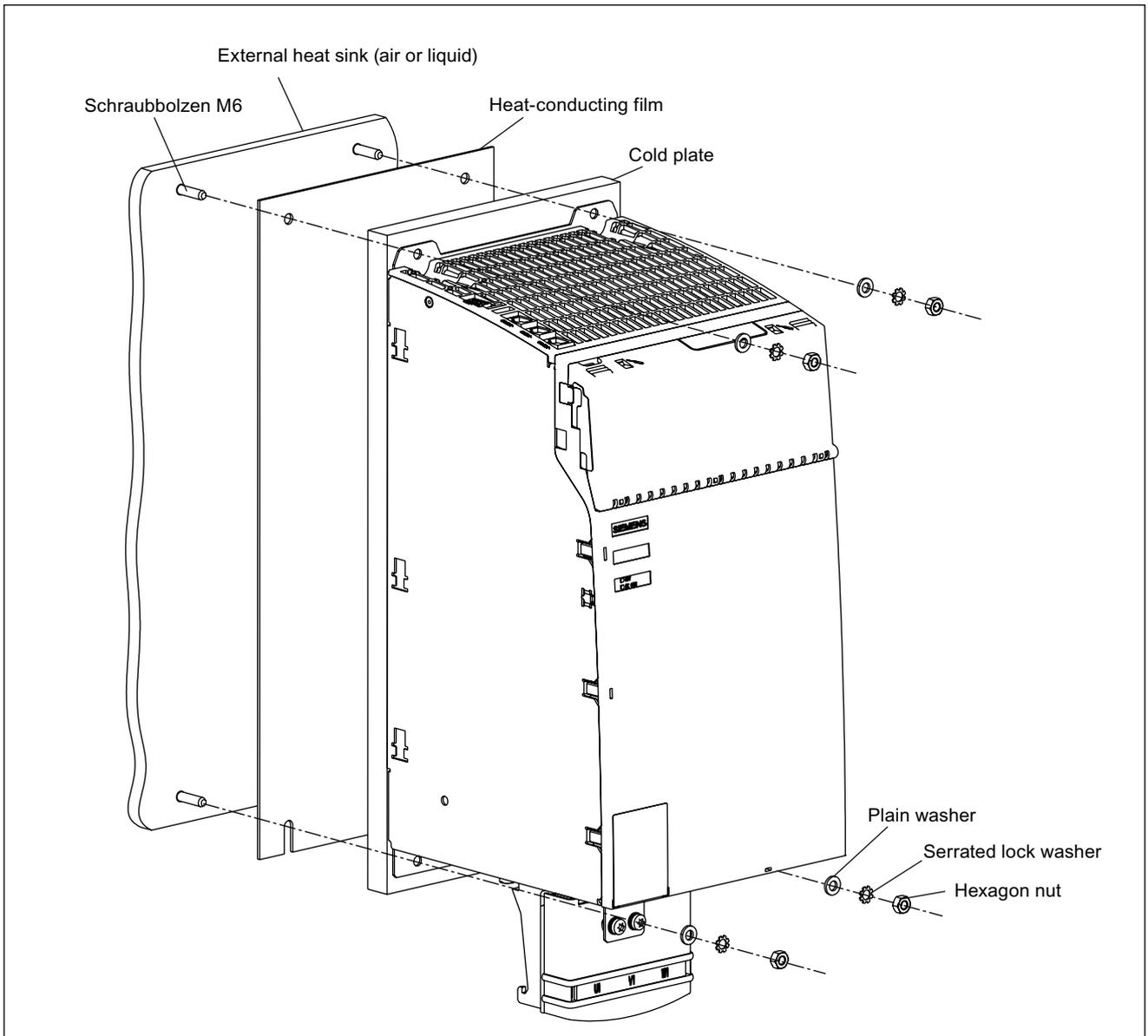
Figure 6-10 Installation of Basic Line Module 100 kW with external heat sink and heat-conducting film
