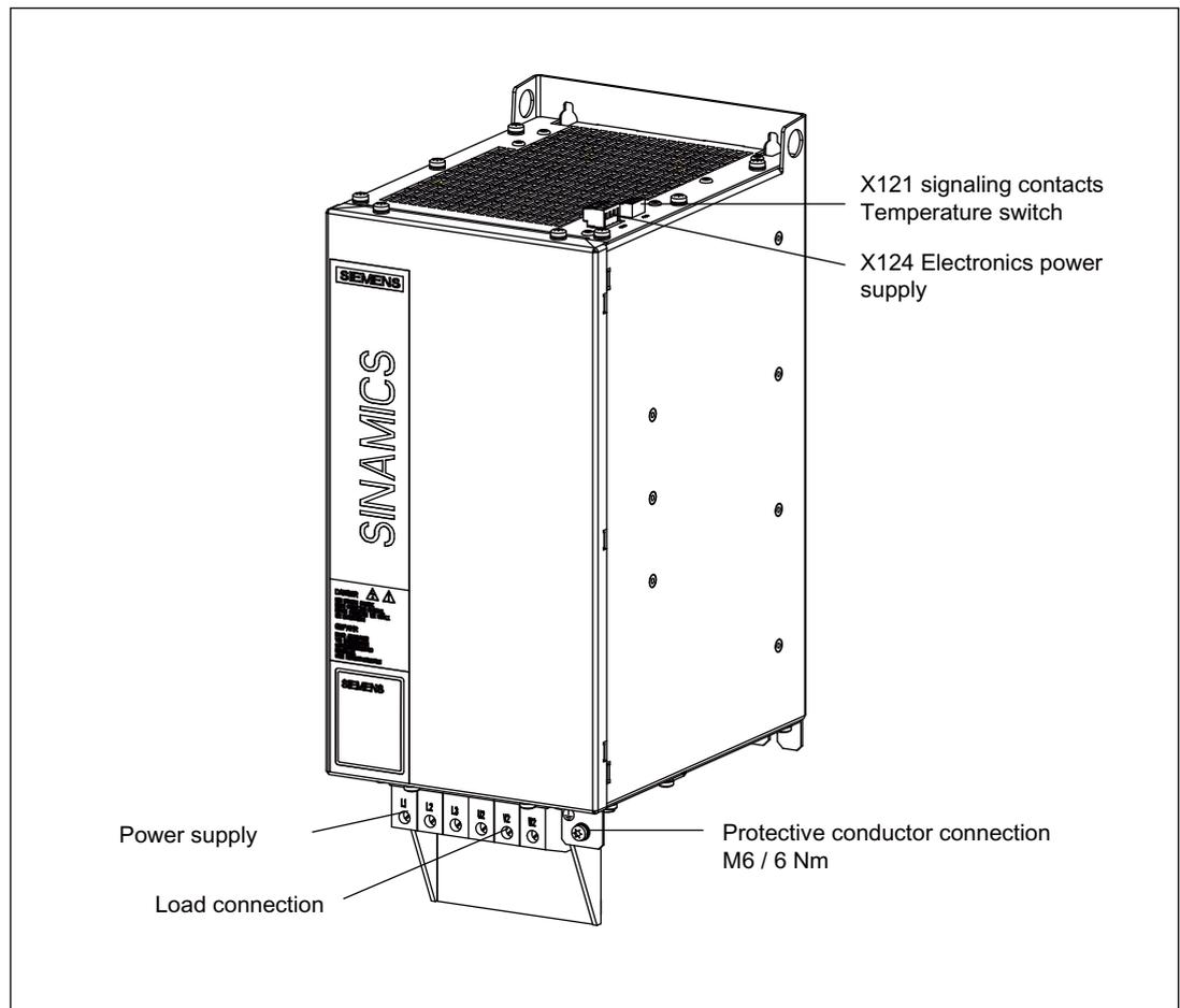
Figure 4-21 Interface description: Active Interface Module 55 kW
