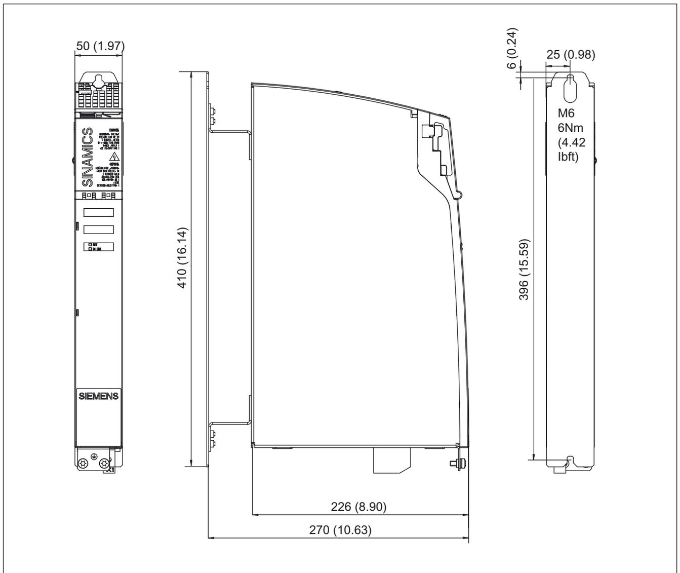
Figure 11-16 Dimension drawing of the Voltage Clamping Module
