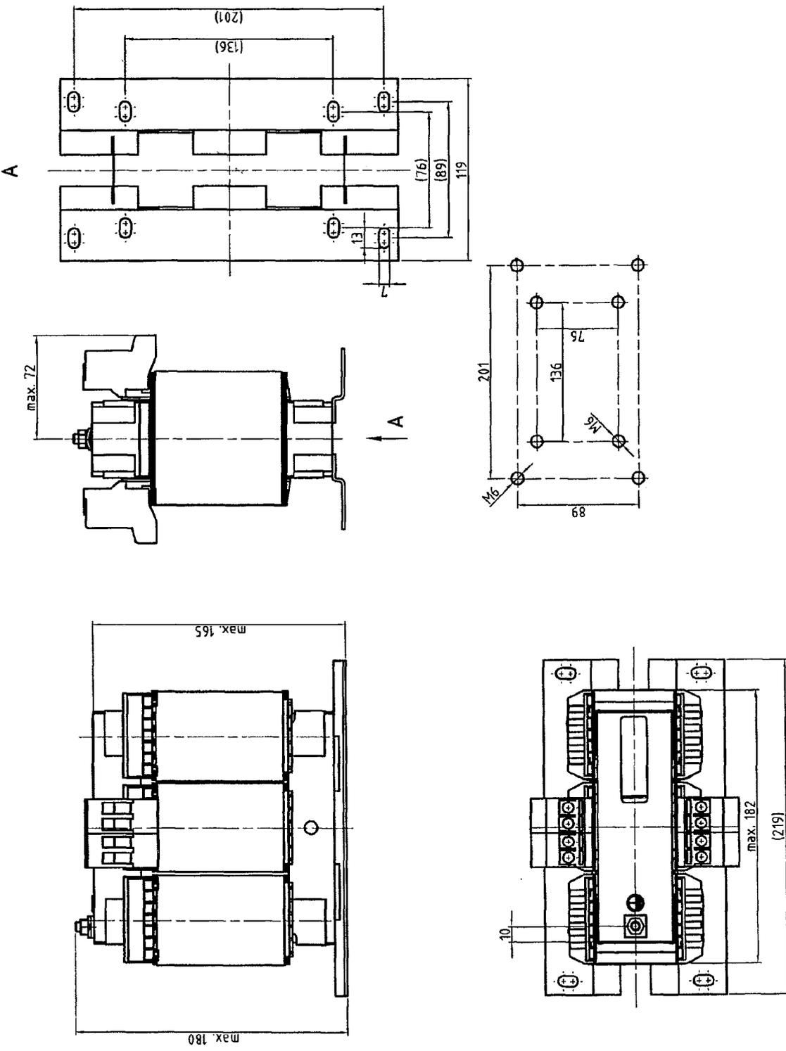
Figure 4-32 Dimension drawing of line reactor for the Smart Line Module 16 kW
