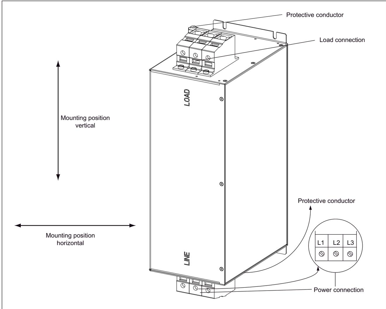
Figure 4-7 Interface description: 80 kW and 120 kW Basic Line Filter
