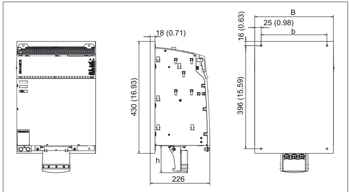
Figure 8-7 Dimension drawing of Motor Module with cold plate (132 A and 200 A)
