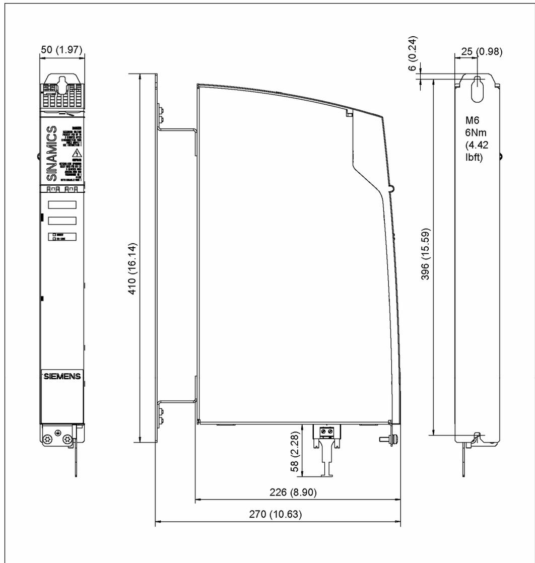
Figure 11-3 Dimension drawing of the Braking Module
