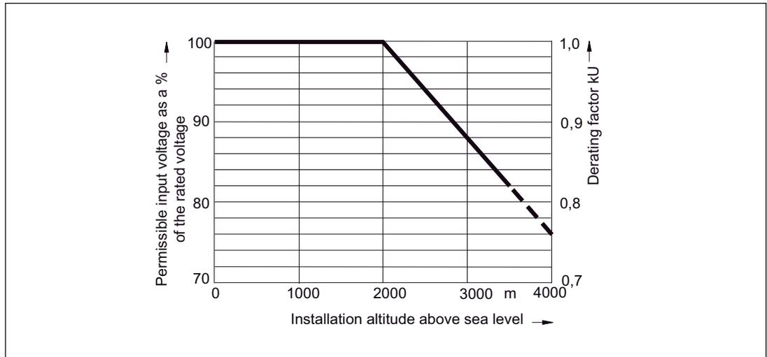
Figure 5-9 Voltage derating as a function of the installation altitude
