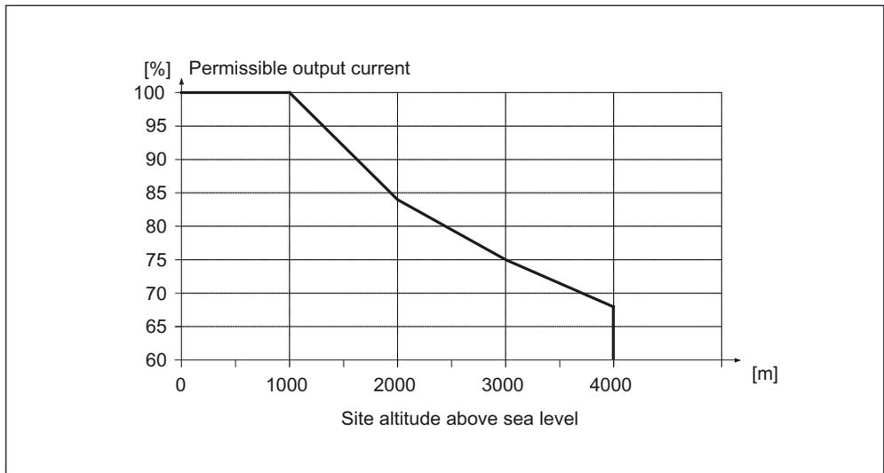
Figure 7-7 Derating as a function of the site altitude
