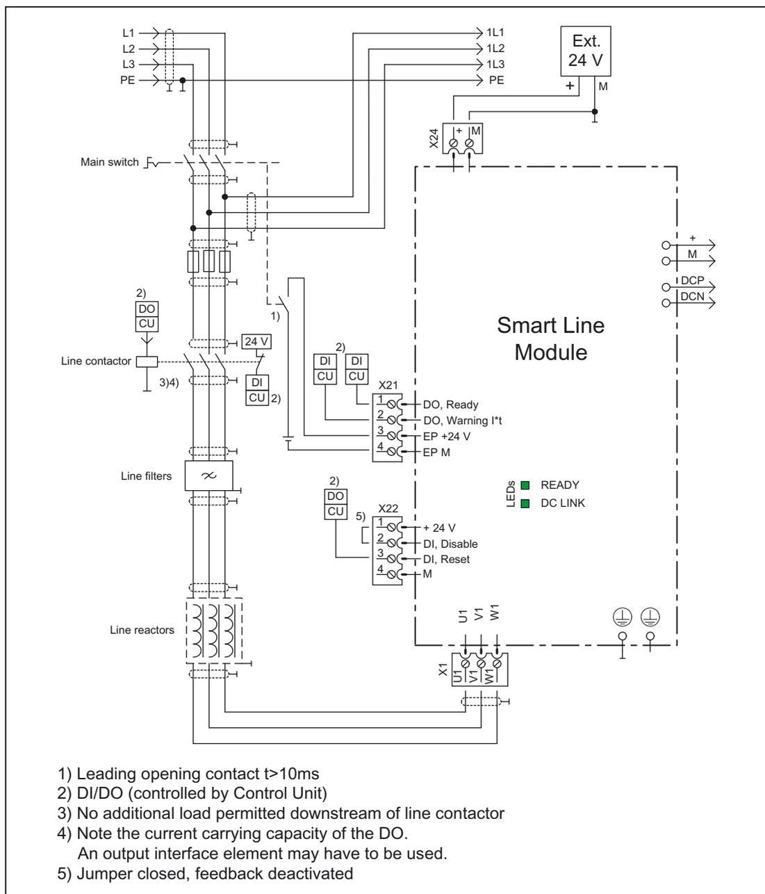
Figure 7-2 Connection example: smart line module with cold plate
