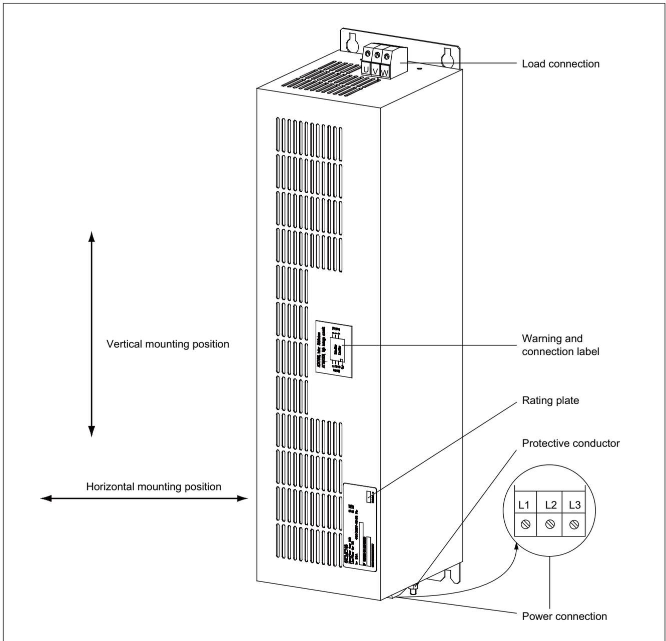
Figure 4-10 Wideband Line Filter for Active Line Module (example: 16 kW)
