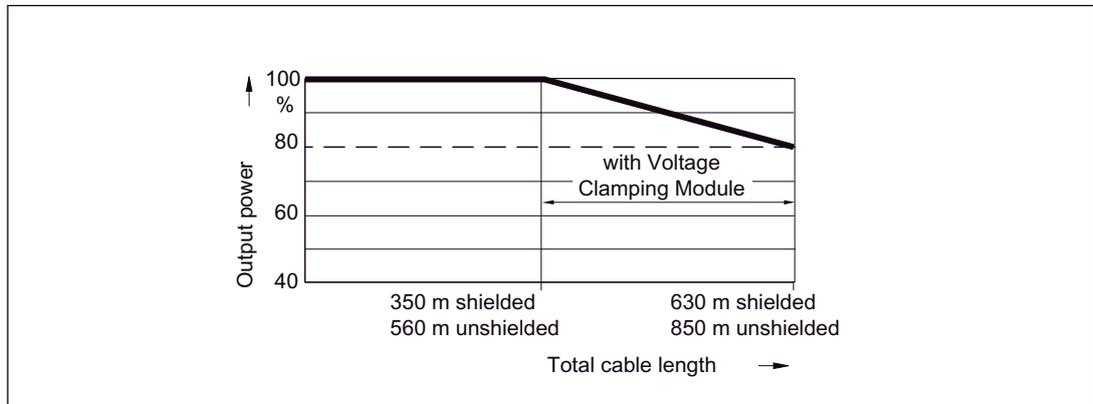
Figure 6-18 Output power as a function of total cable length
