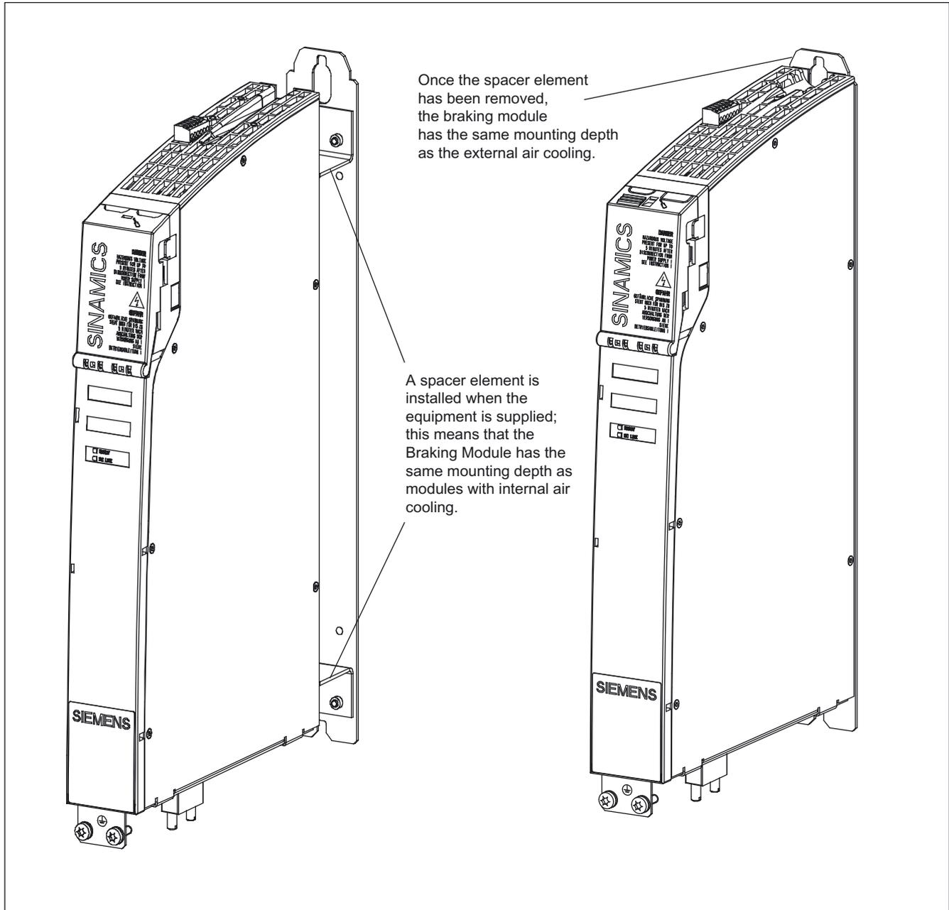
Figure 11-4 Methods of installing Braking Modules with/without spacer elements
