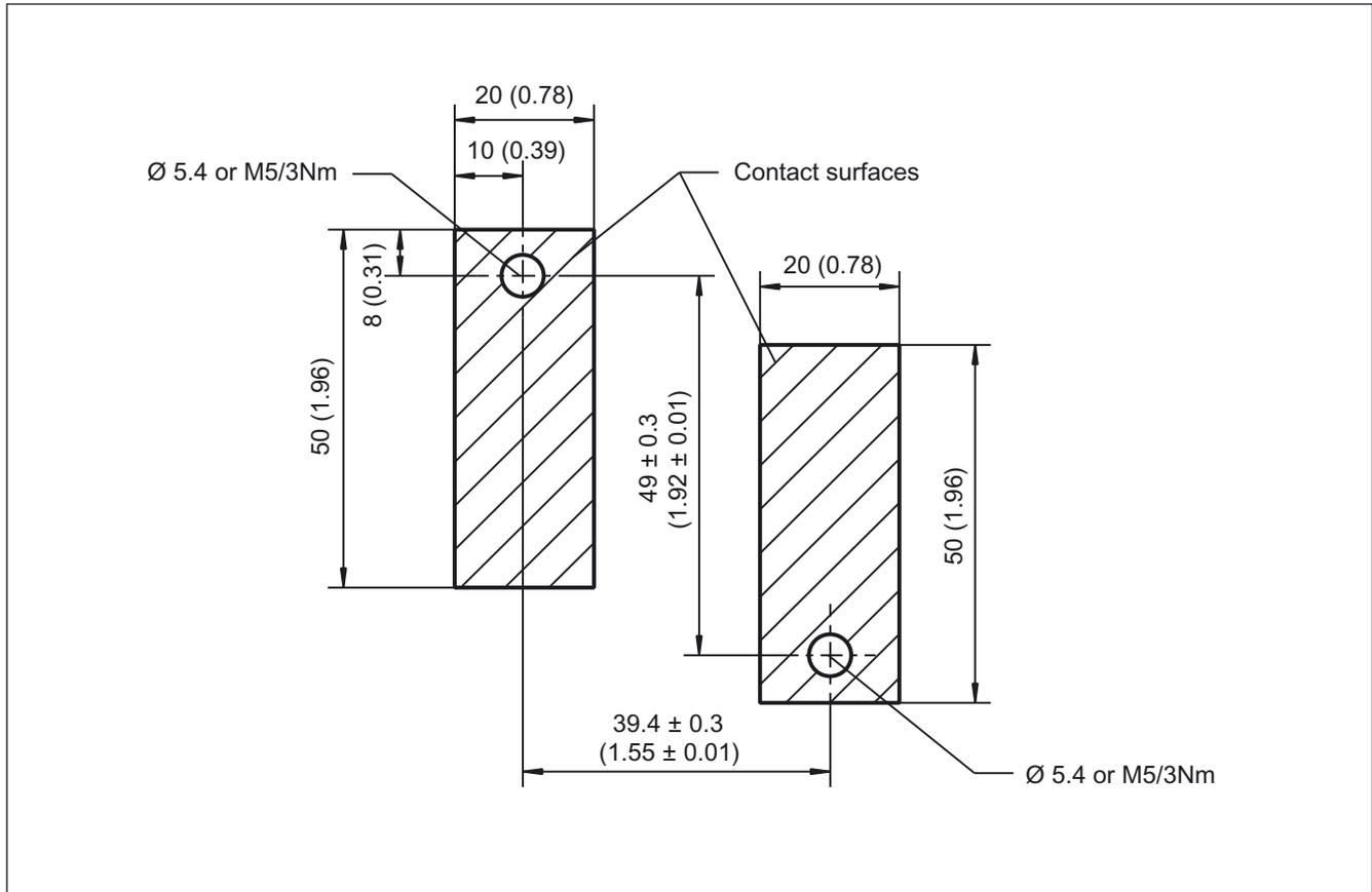
Figure 13-16 Hole drilling template for installation
