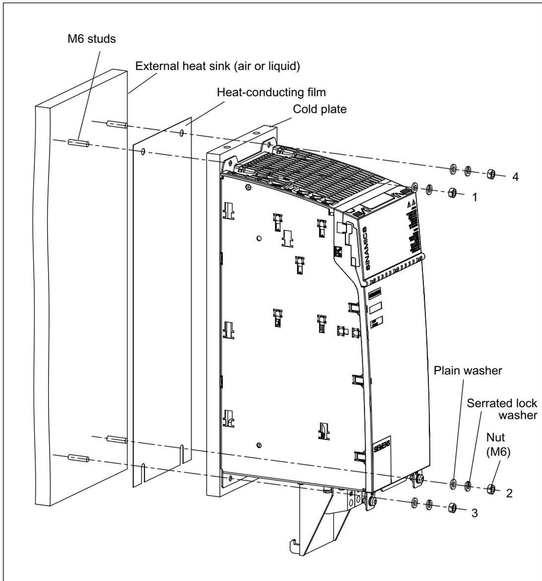
Figure 6-9 Installation of Basic Line Module 40 kW with external heat sink and heat-conducting film
