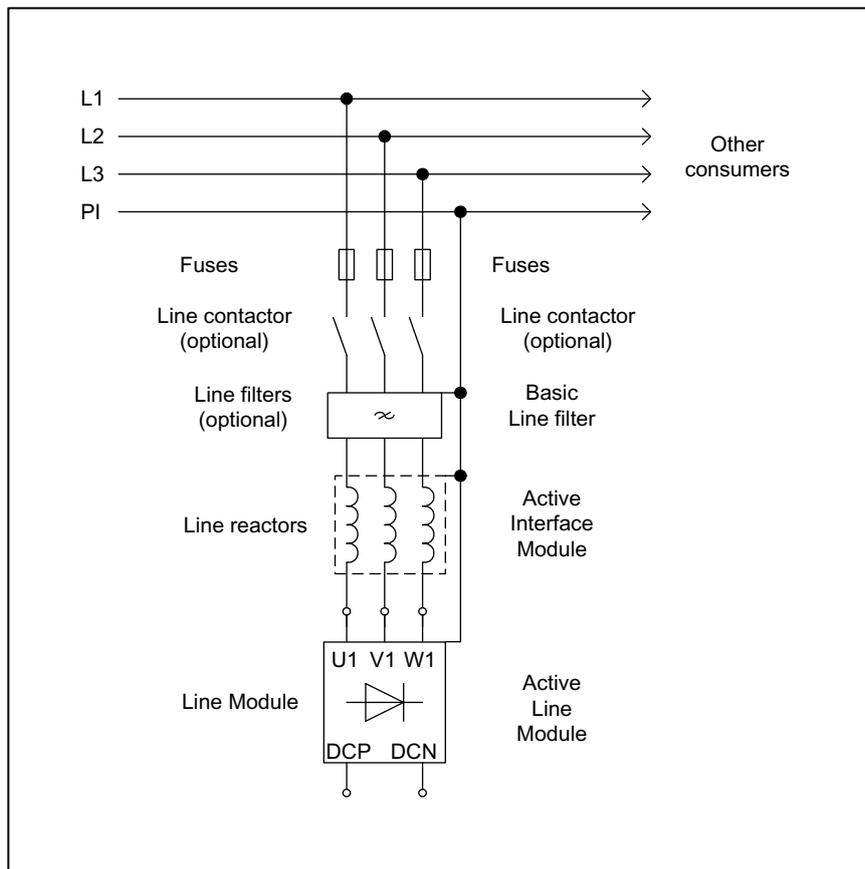
Figure 4-41 Direct operation on the line supply
