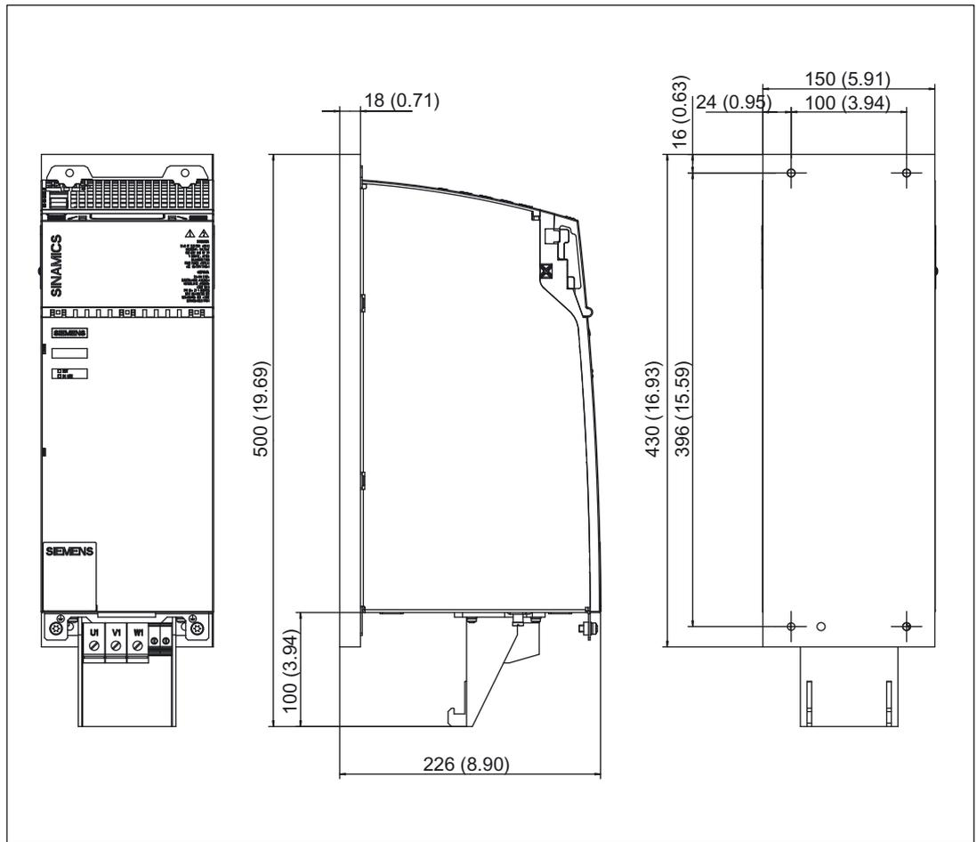
Figure 6-7 Dimension drawing: Basic Line Module with cold plate 40 kW
