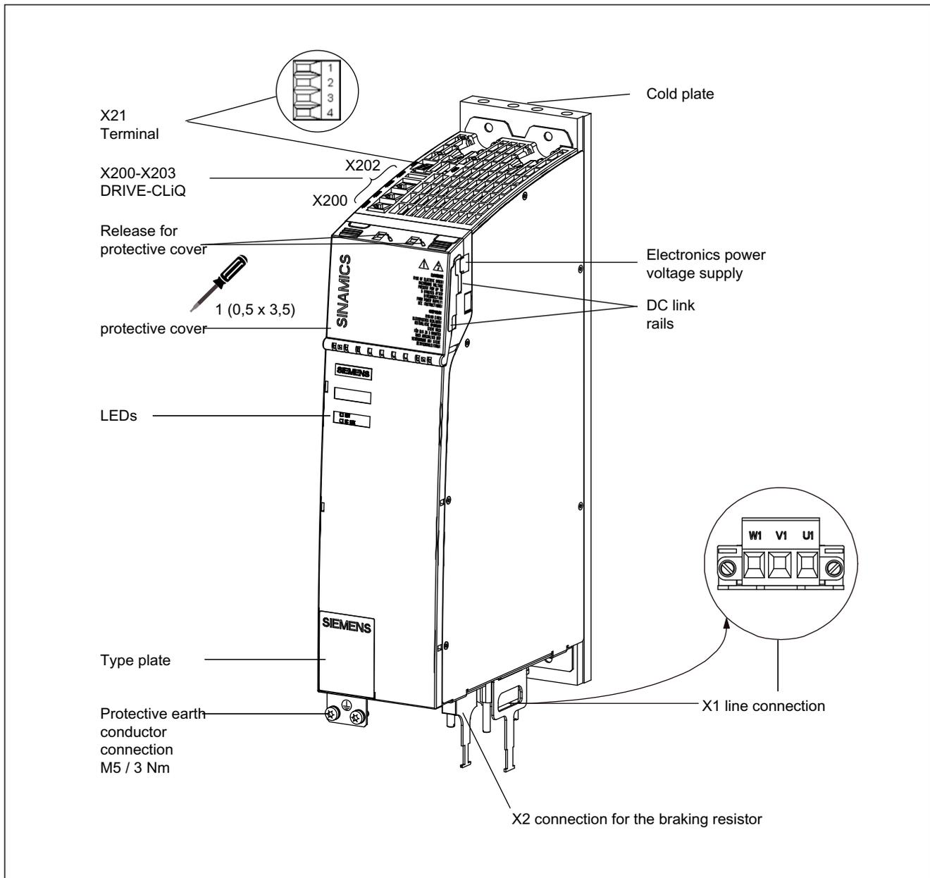
Figure 6-1 Interface description: Basic Line Module with cold-plate cooling (20 kW)
