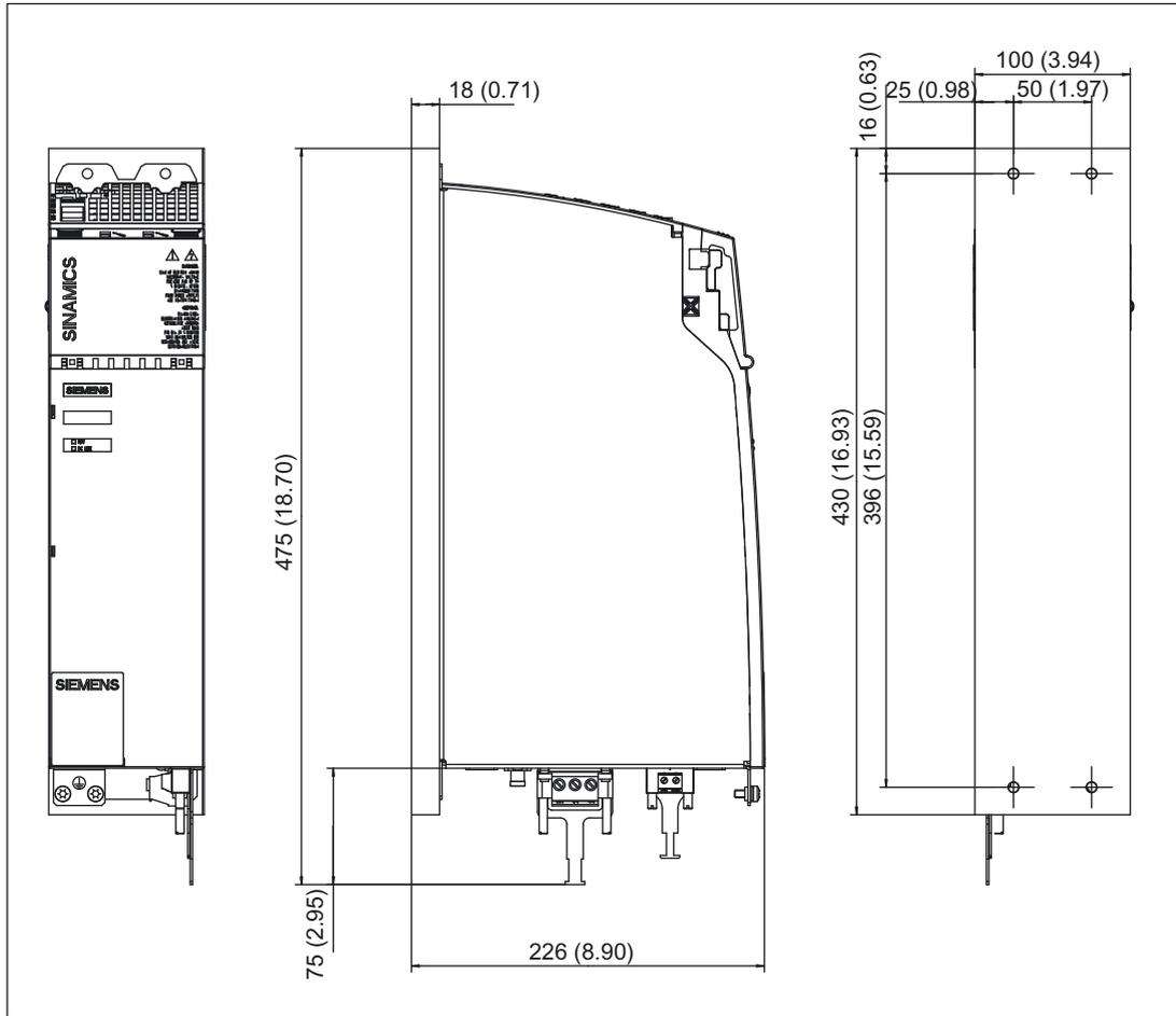
Figure 6-6 Dimension drawing: Basic Line Module with cold plate 20 kW
