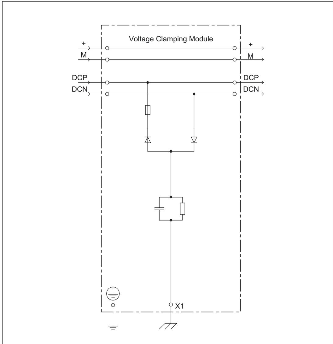
Figure 11-15 Circuit diagram: Voltage Clamping Module
