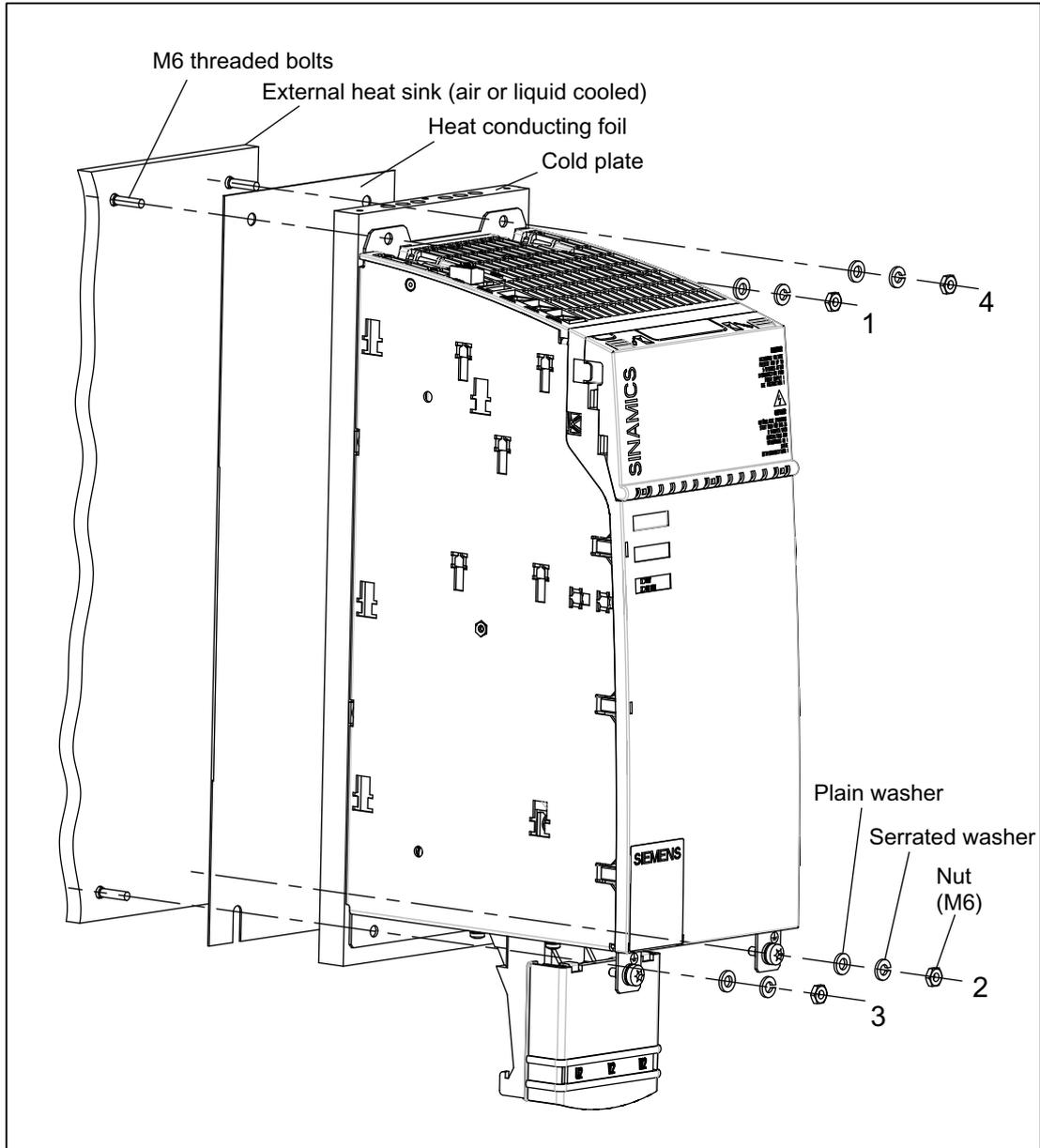
Figure 5-5 Installing a cold-plate power section with an external heat sink and heat-conducting film
