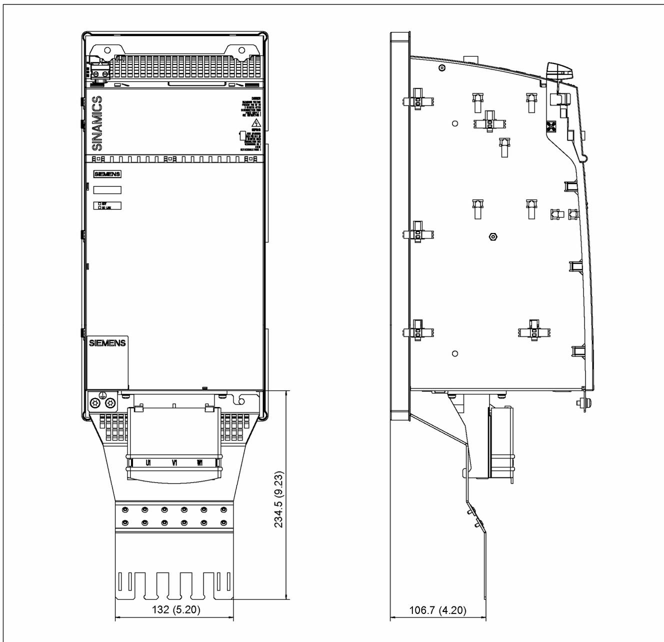
Figure 13-4 Dimension drawing, shield connecting plate on a 200 mm component with cold plate
