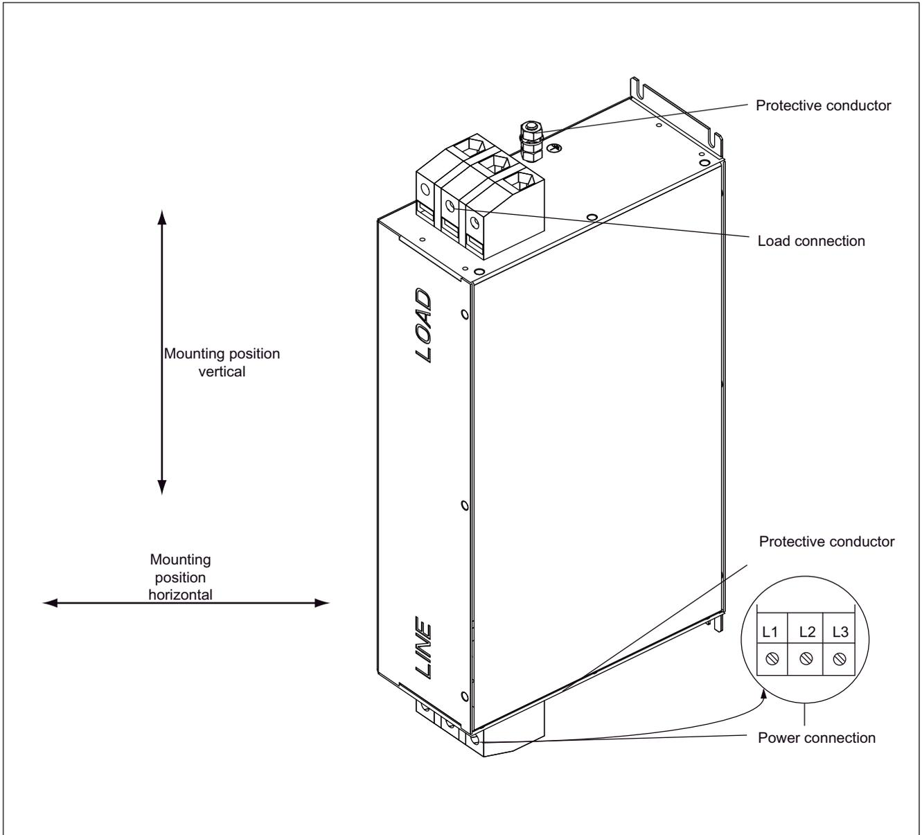
Figure 4-6 Interface description: Basic Line Filter 55 kW
