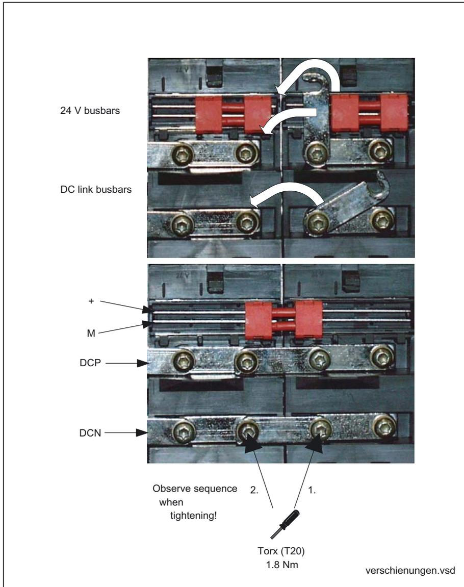
Figure 6-11 Busbar connections for booksize components
