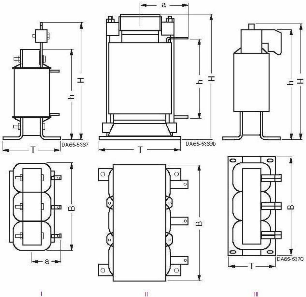
Figure 12-1 Dimension drawings: Motor reactors
