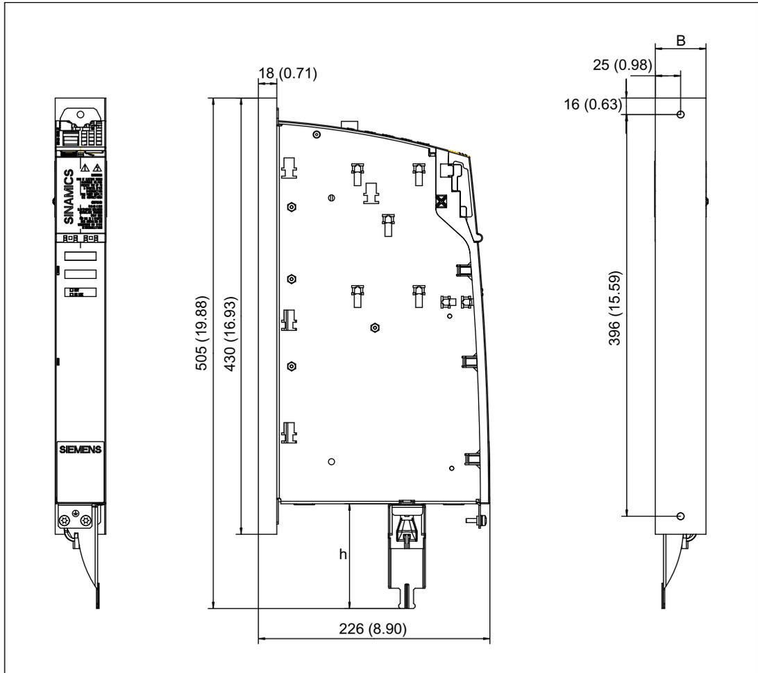
Figure 8-4 Dimension drawing of Motor Module with cold plate 3 A to 18 A and 2 x 3 A to 2 x 9 A
