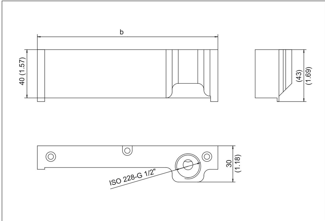
Figure 9-1 Dimension drawing of connection adapter
