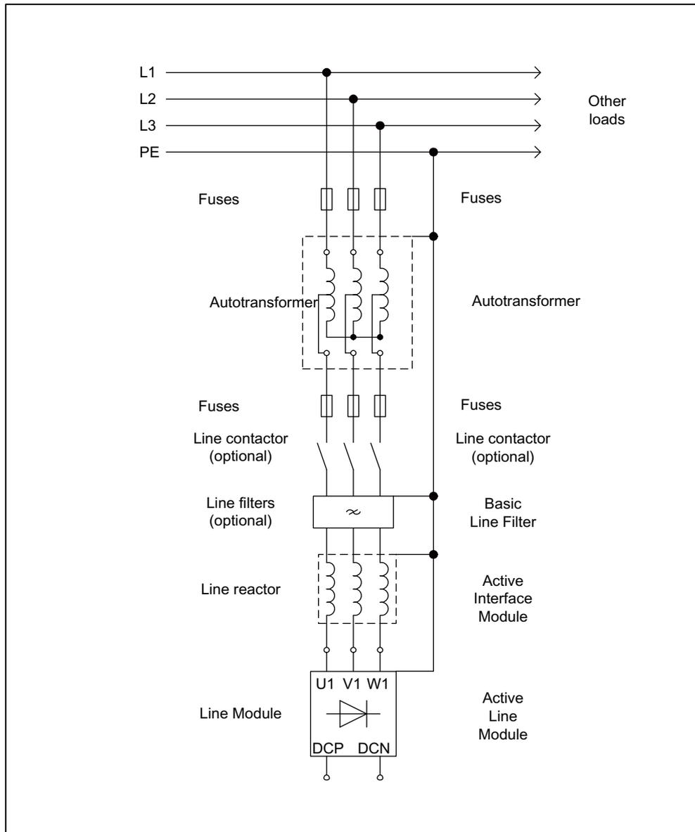
Figure 4-42 Autotransformer
