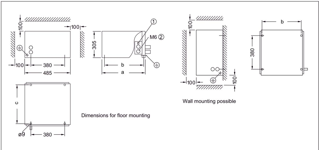
Figure 6-20 Dimension drawing: Braking resistor 30 kW and 75 kW
