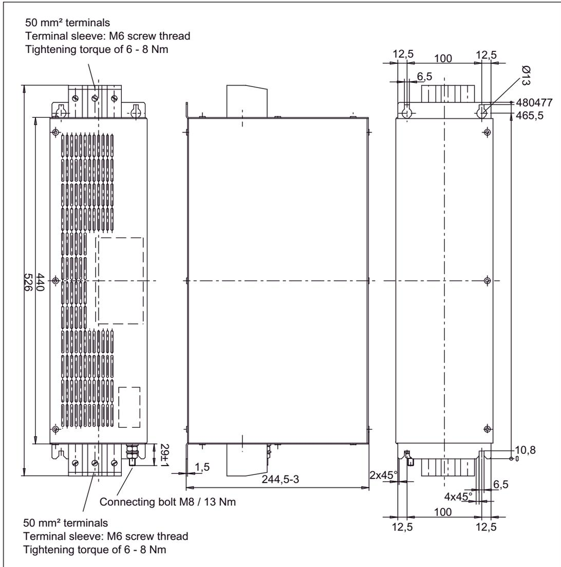
Figure 4-12 Dimension drawing: 36 kW Wideband Line Filter for Active Line Modules
