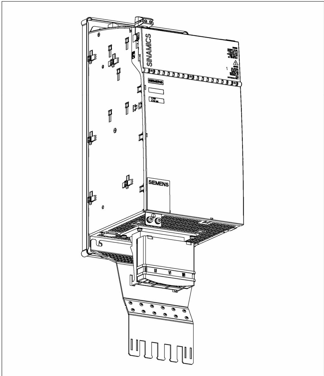
Figure 13-1 Shield connecting plate for a 200 mm module with with a cold plate
