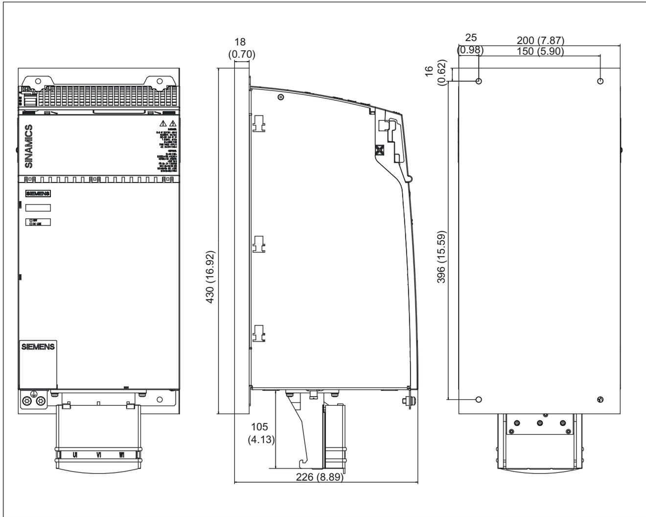
Figure 6-8 Dimension drawing: Basic Line Module with cold plate 100 kW
