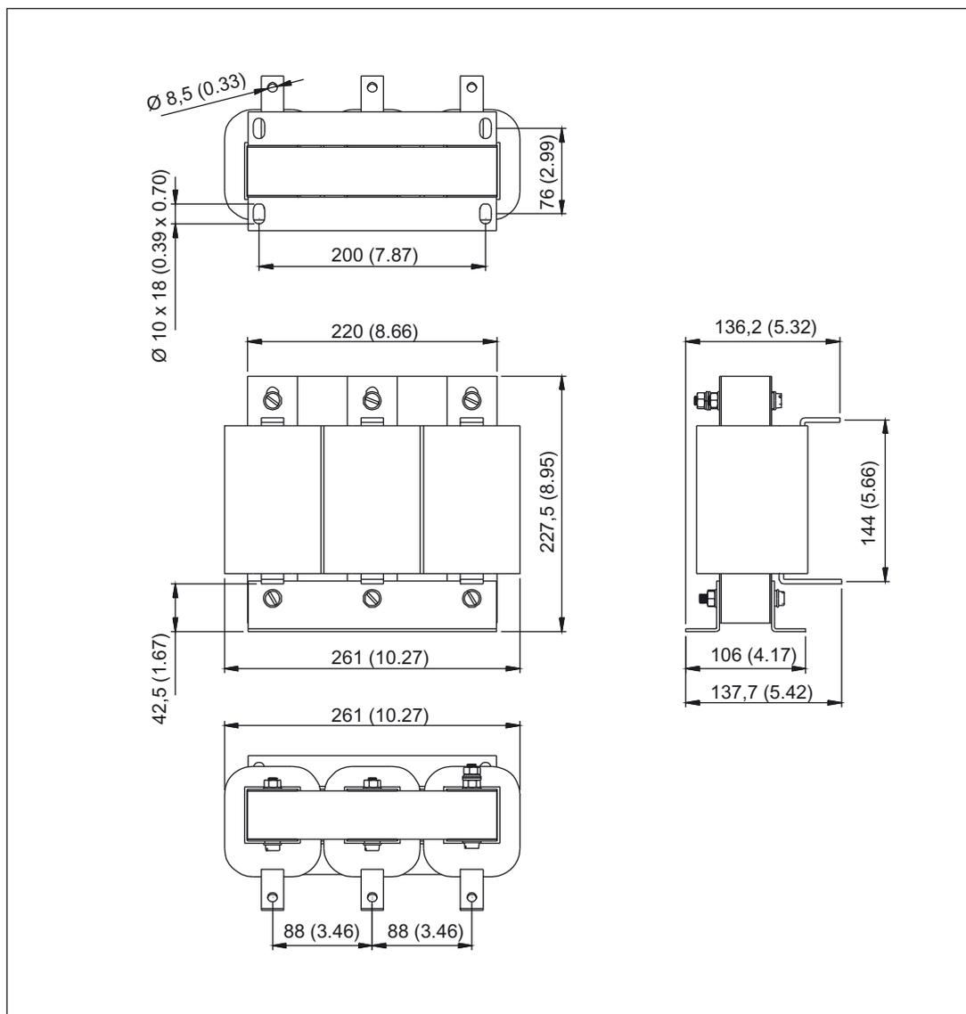
Figure 4-39 Dimension drawing: Line reactor for Basic Line Module (100 kW)
