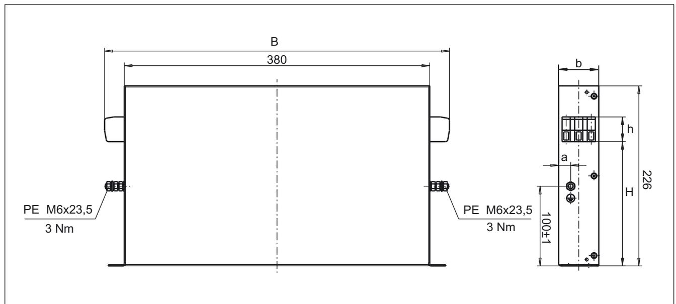
Figure 4-8 Dimension drawing: Basic Line Filter 55 kW
