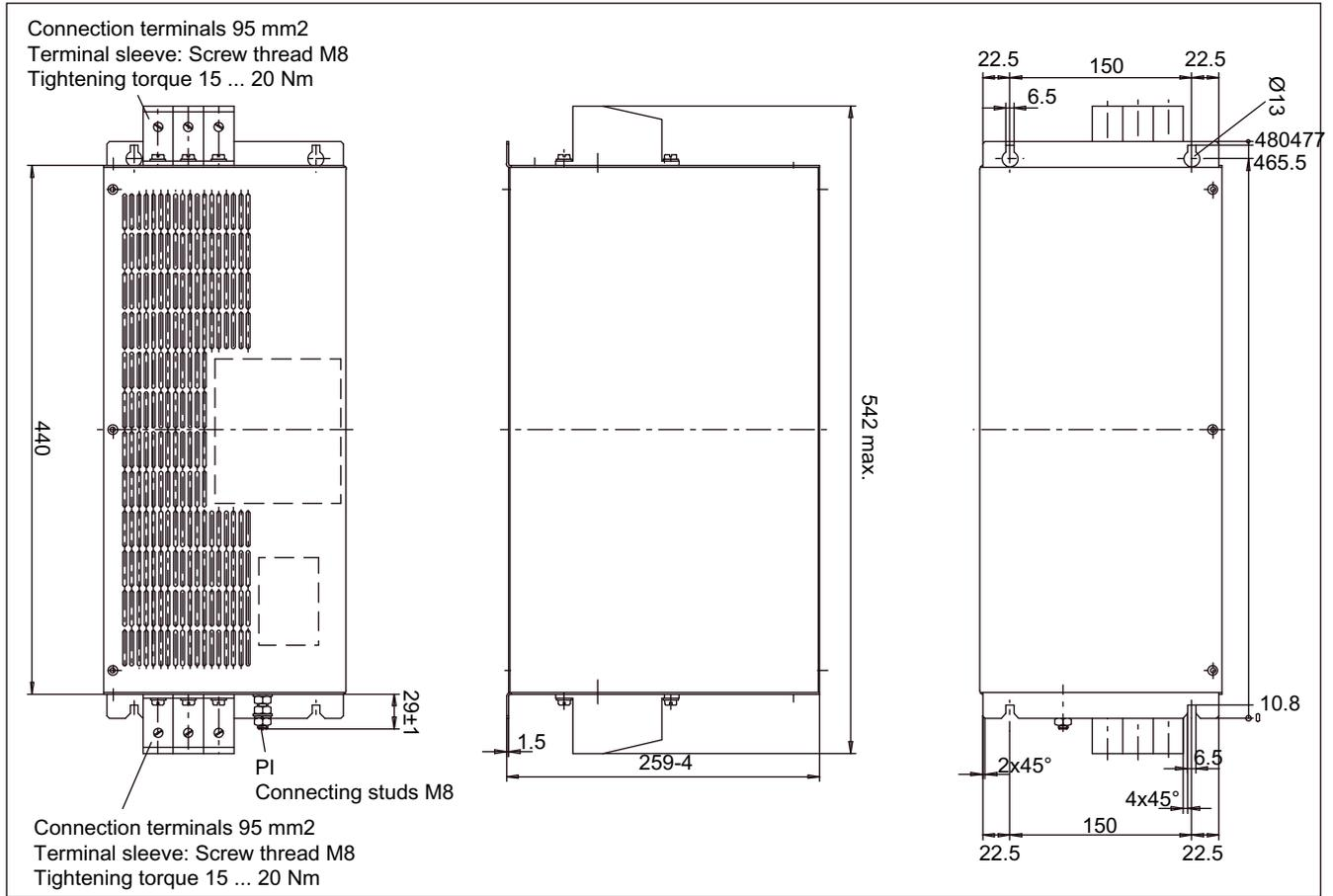
Figure 4-14 Dimension drawing: 80 kW Wideband Line Filter for Active Line Modules
