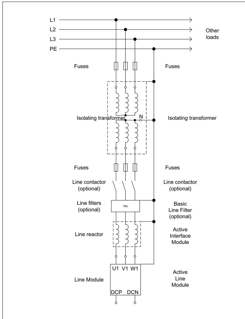
Figure 4-43 Isolating transformer
