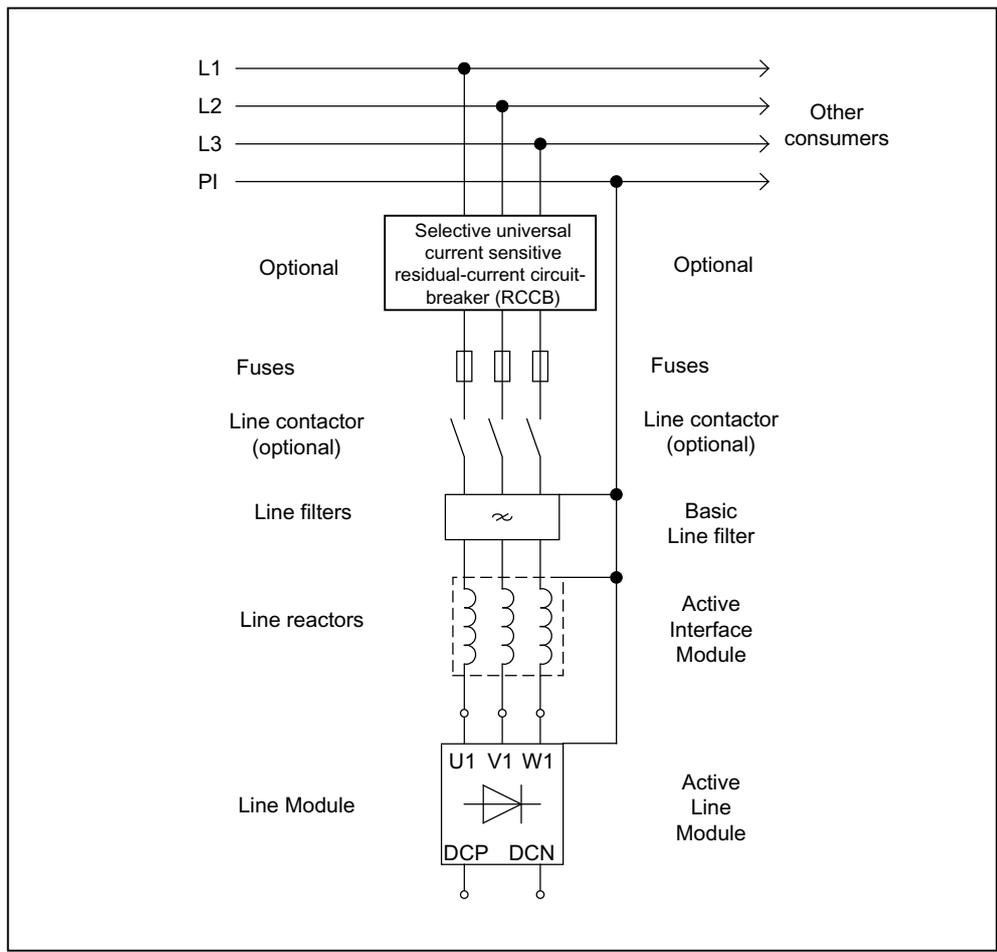
Figure 4-44 Residual-current circuit-breaker (RCCB)
