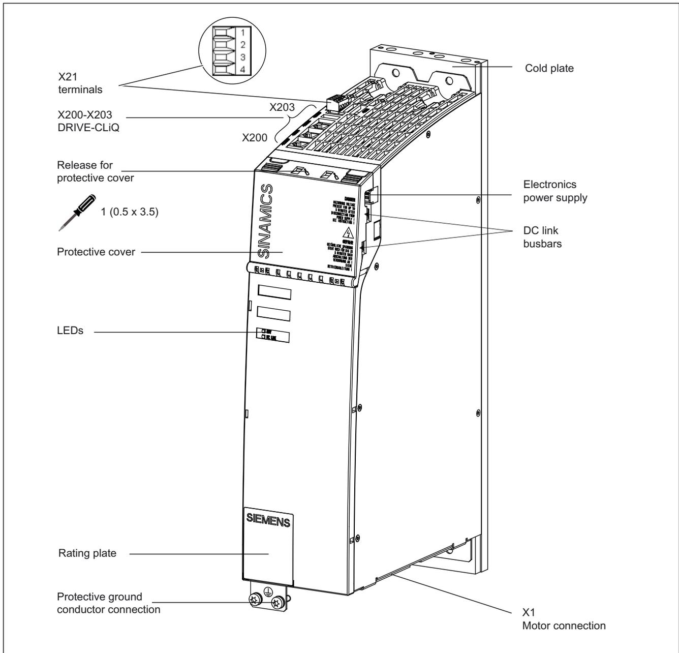
Figure 8-1 Single motor module with cold plate (example 30 A)
