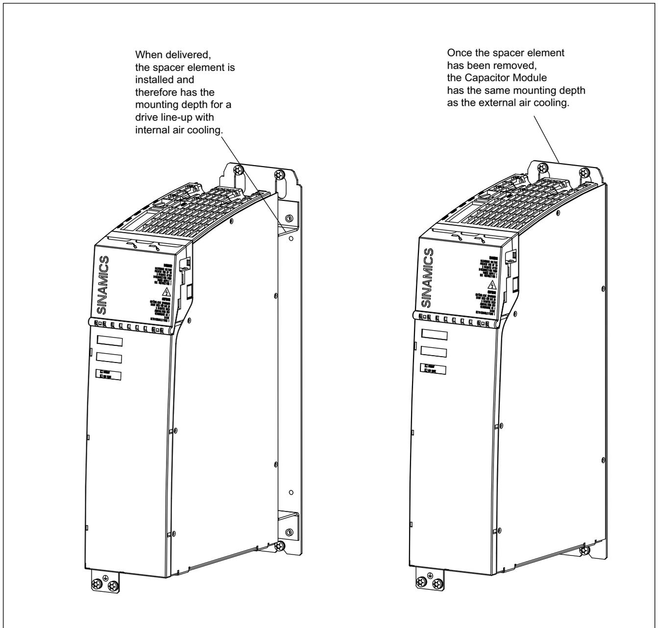
Figure 11-10 Installing a Capacitor Module with/without spacer elements
