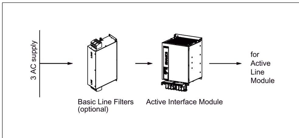
Figure 4-2 Overview: line connection with Active Interface Module
