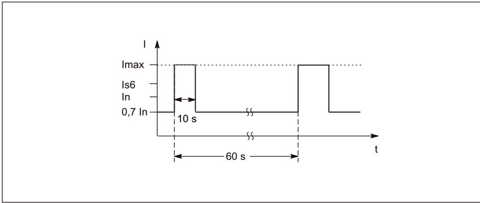
Figure 8-12 S6 peak current duty cycle with prior loading
