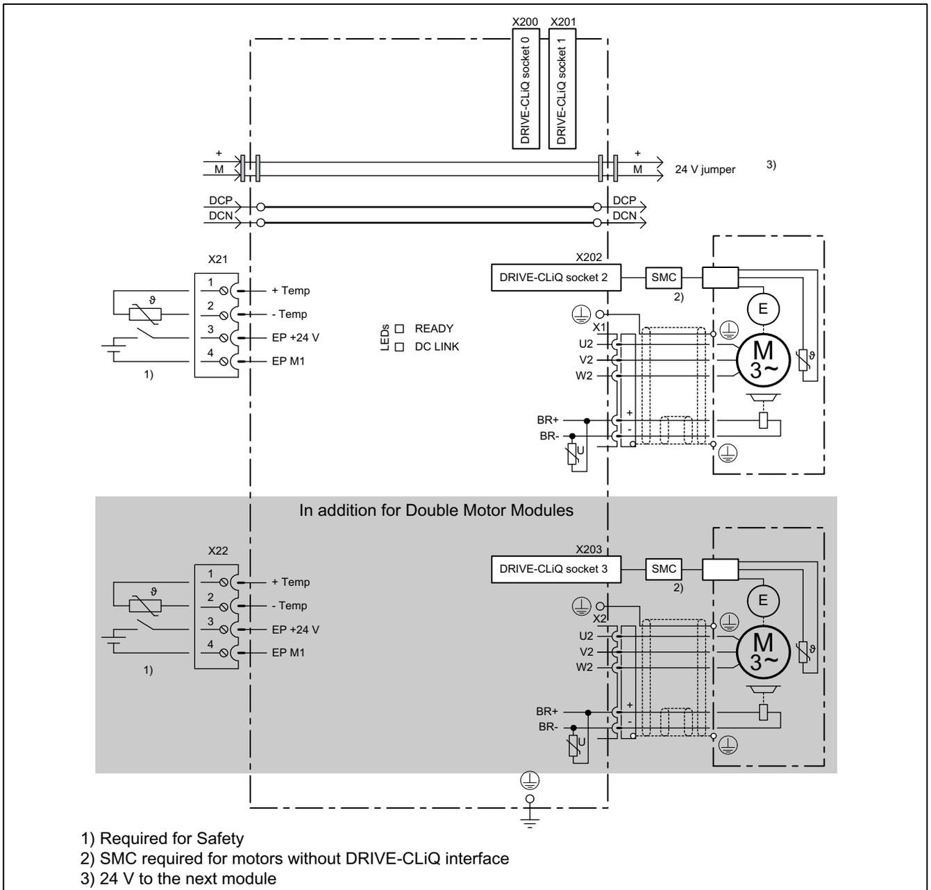
Figure 8-2 Connection example of Motor Modules 3 A to 30 A and Double Motor Modules 3 A to 18 A
