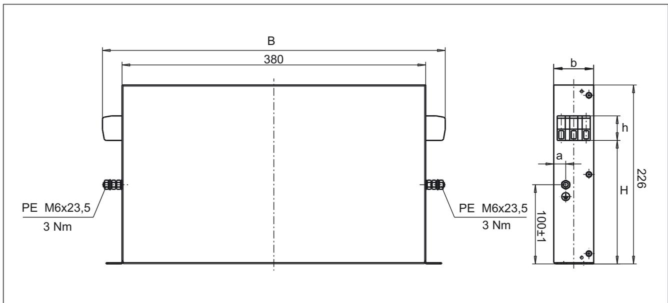
Figure 4-17 Dimension drawing: Basic Line Filter for Basic Line Modules (20 kW and 40 kW)
