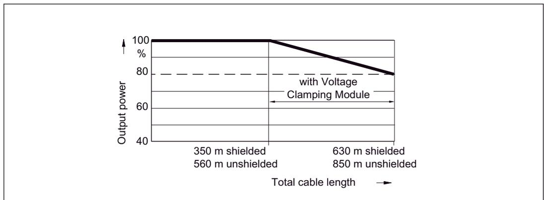
Figure 5-10 Output power as a function of total cable length
