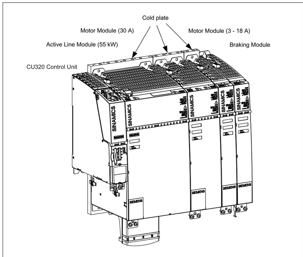
Figure 14-2 Example of a drive line-up
