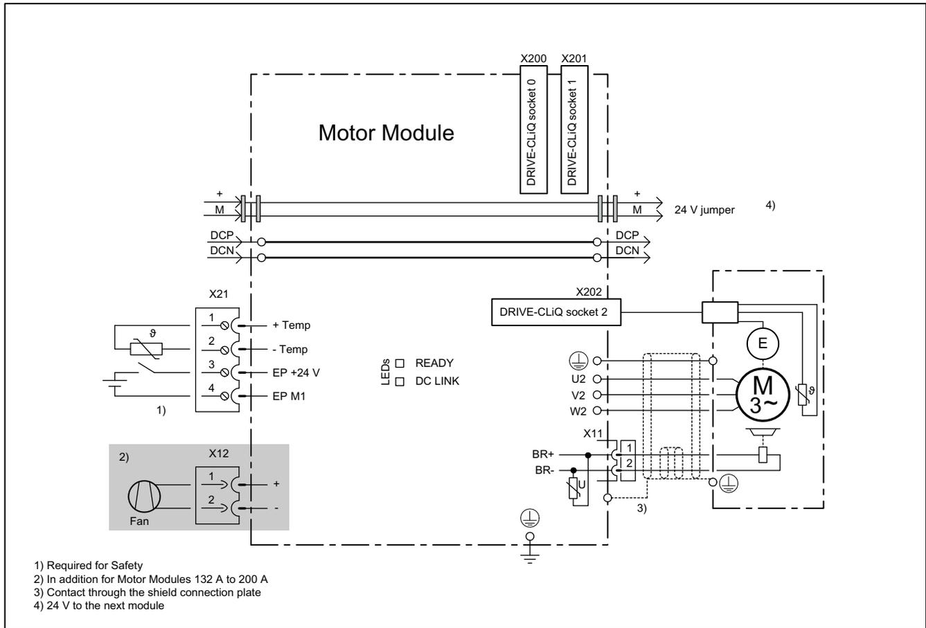
Figure 8-3 Example connection of Single Motor Modules 45 A to 200 A
