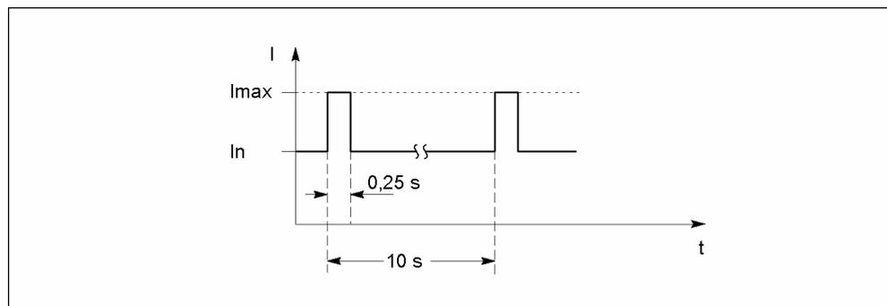
Figure 8-9 Peak current duty cycle with prior loading
