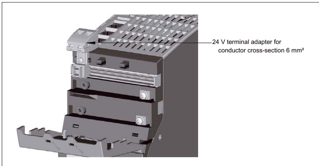
Figure 14-11 24 V terminal adapter
