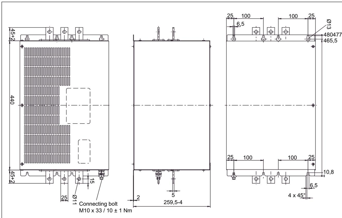
Figure 4-15 Dimension drawing: 120 kW Wideband Line Filter for Active Line Modules
