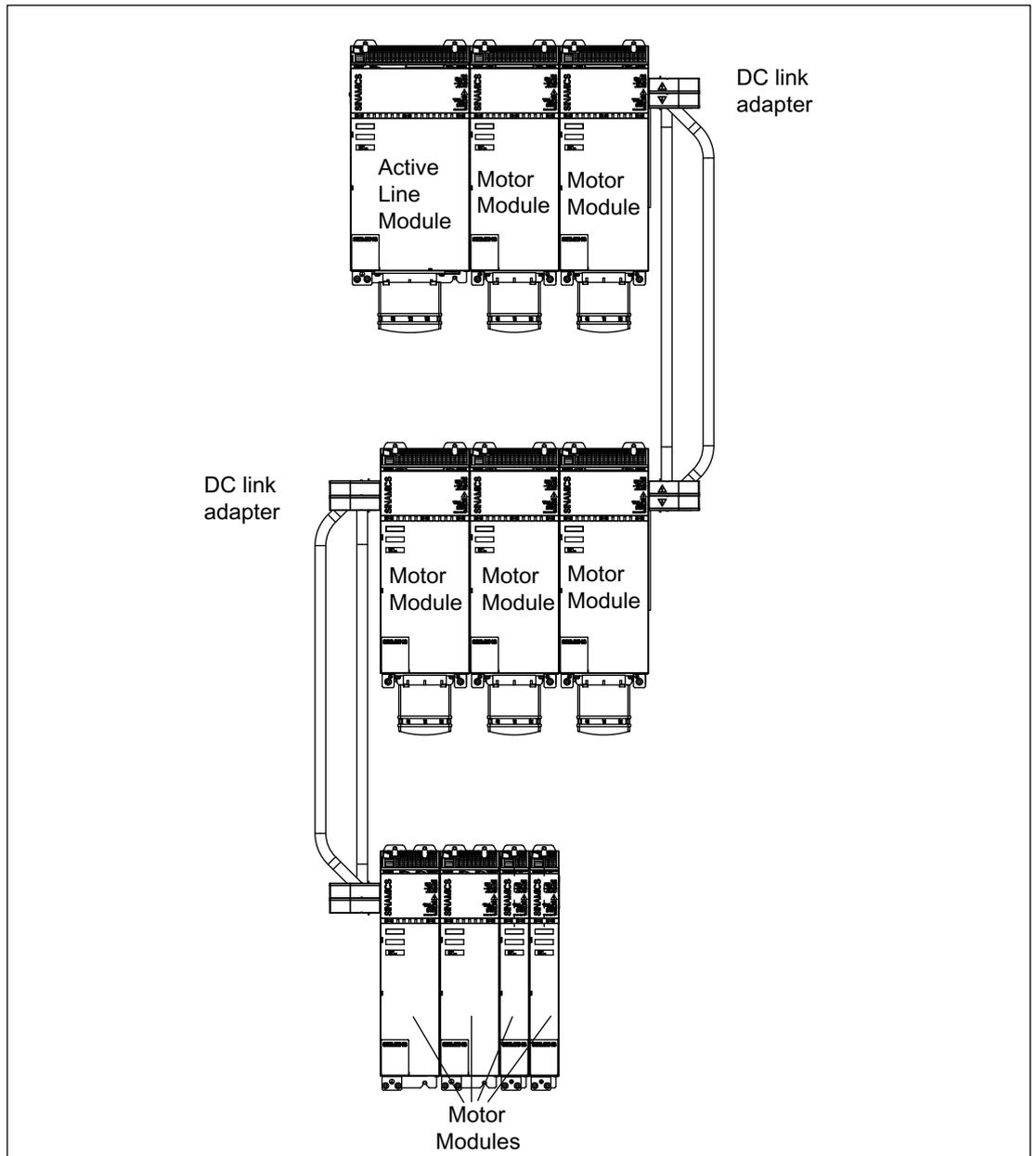
Figure 14-5 Example of a three-tier configuration with components between 50 and 200 mm wide
