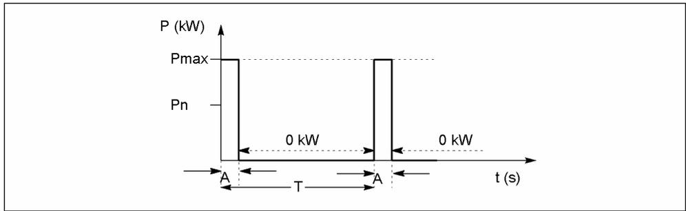
Figure 11-7 Duty cycle for braking resistors
