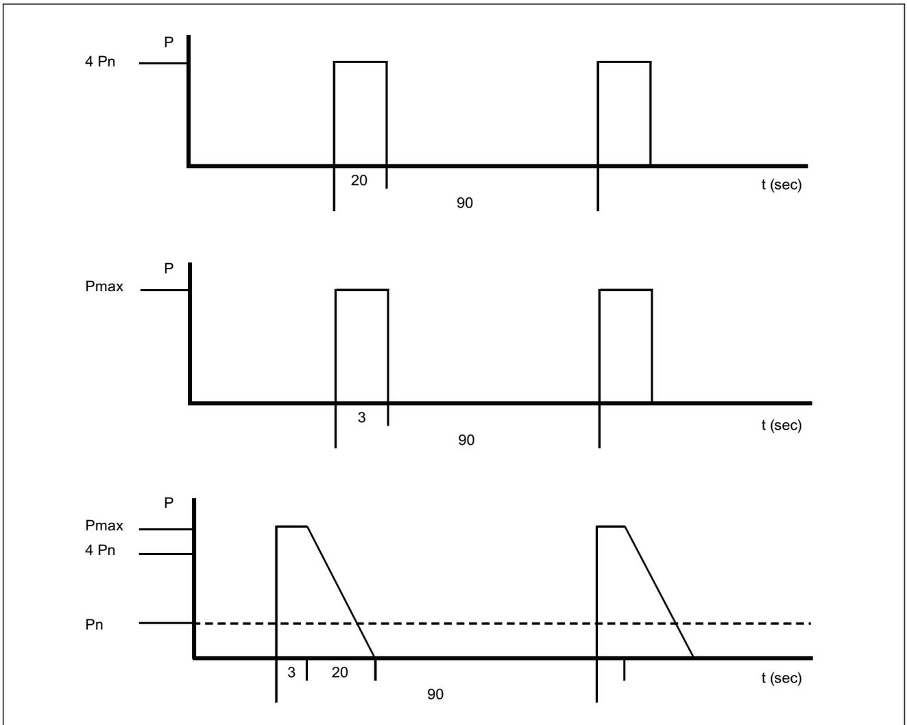
Figure 6-21 Braking duty cycles for braking resistors
