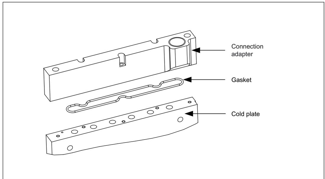
Figure 9-4 Example: connection adapter with seal
