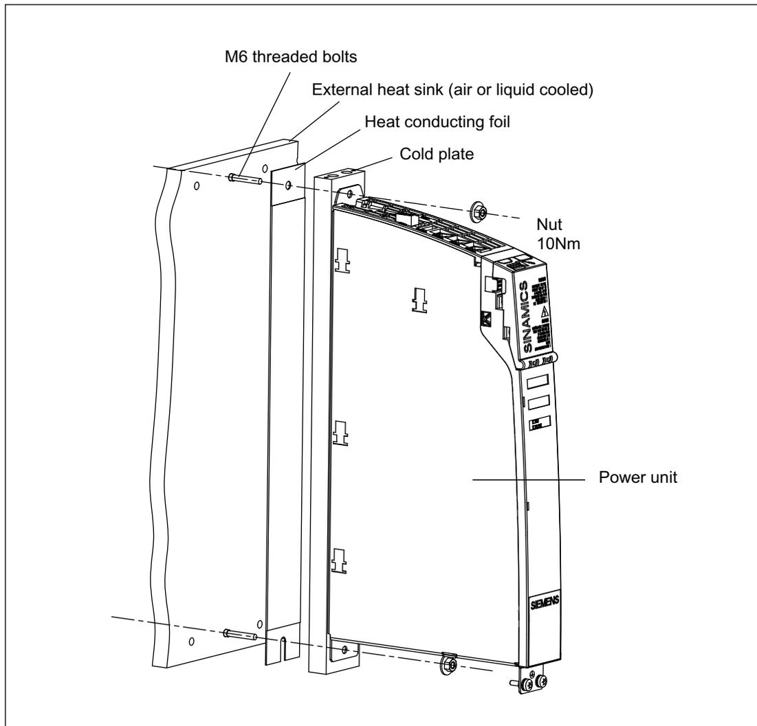
Figure 7-4 Installing a cold-plate power section with an external heat sink
