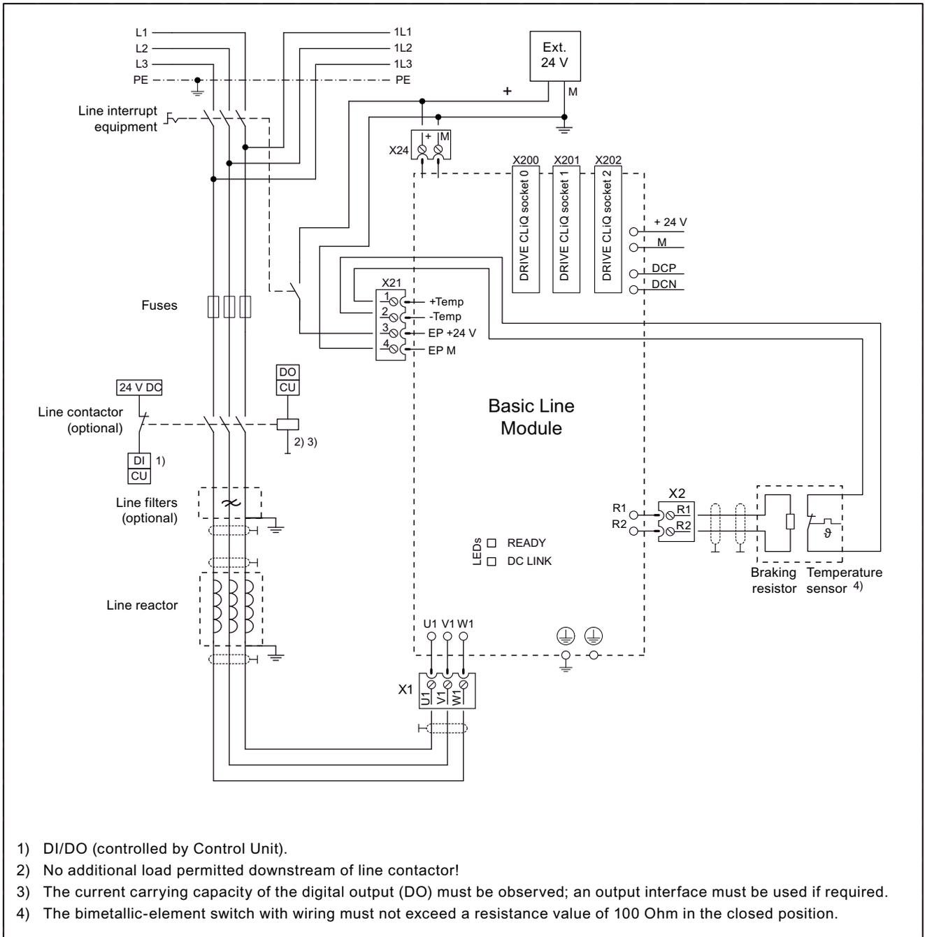
Figure 6-4 Connection example: Basic Line Module (20 kW and 40 kW)
