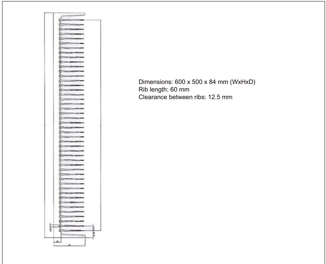
Figure 2-3 Example of an air heat sink
