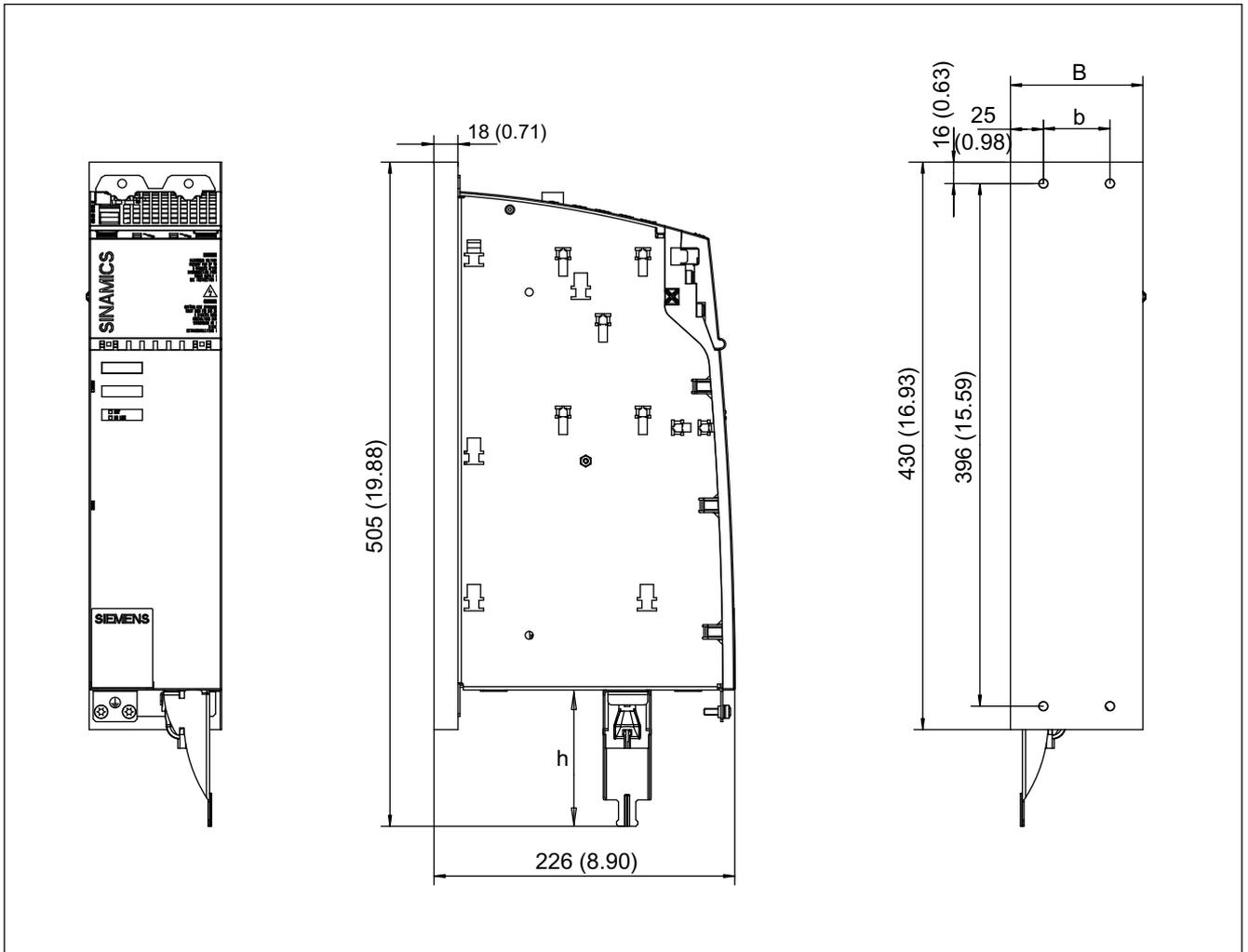
Figure 8-5 Dimension drawing of Motor Module with cold plate 30 A and 2 x 18 A
