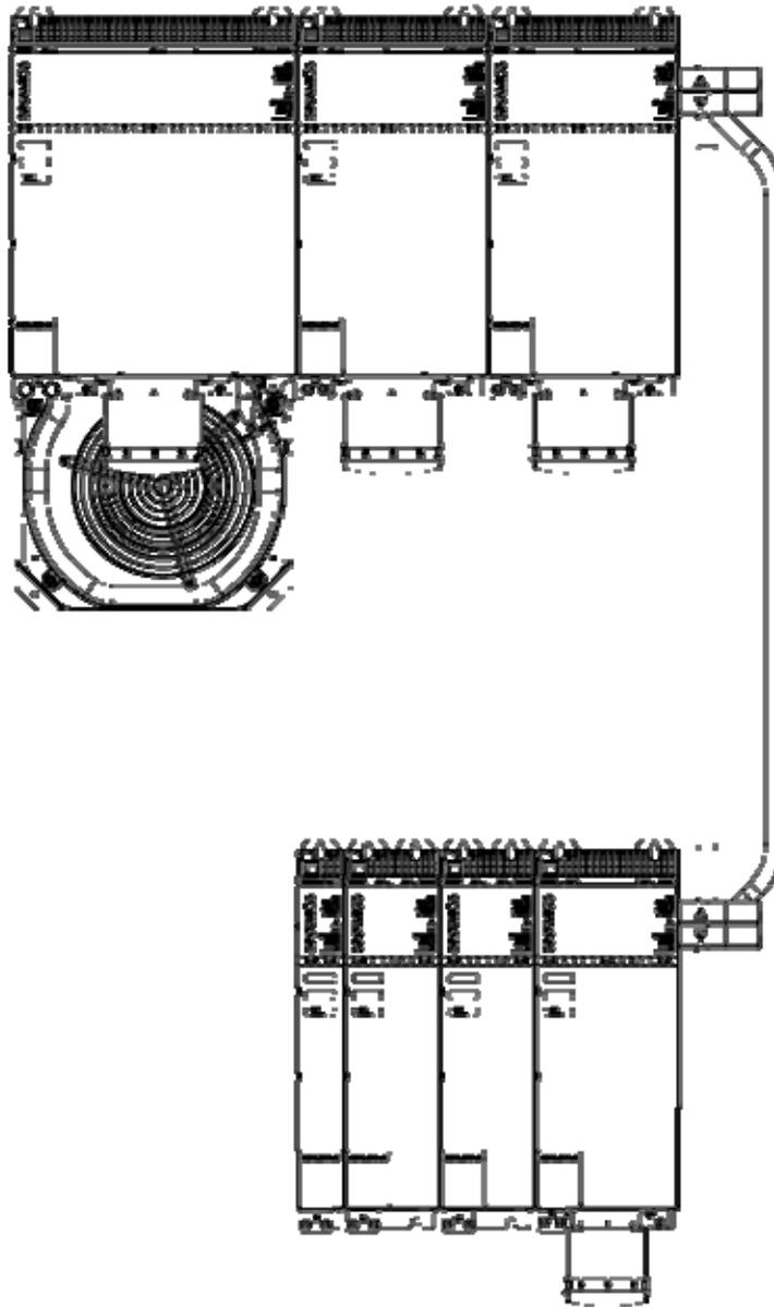
Figure 14-4 Example of a multi-tier configuration with components between 200 and 300 mm wide
