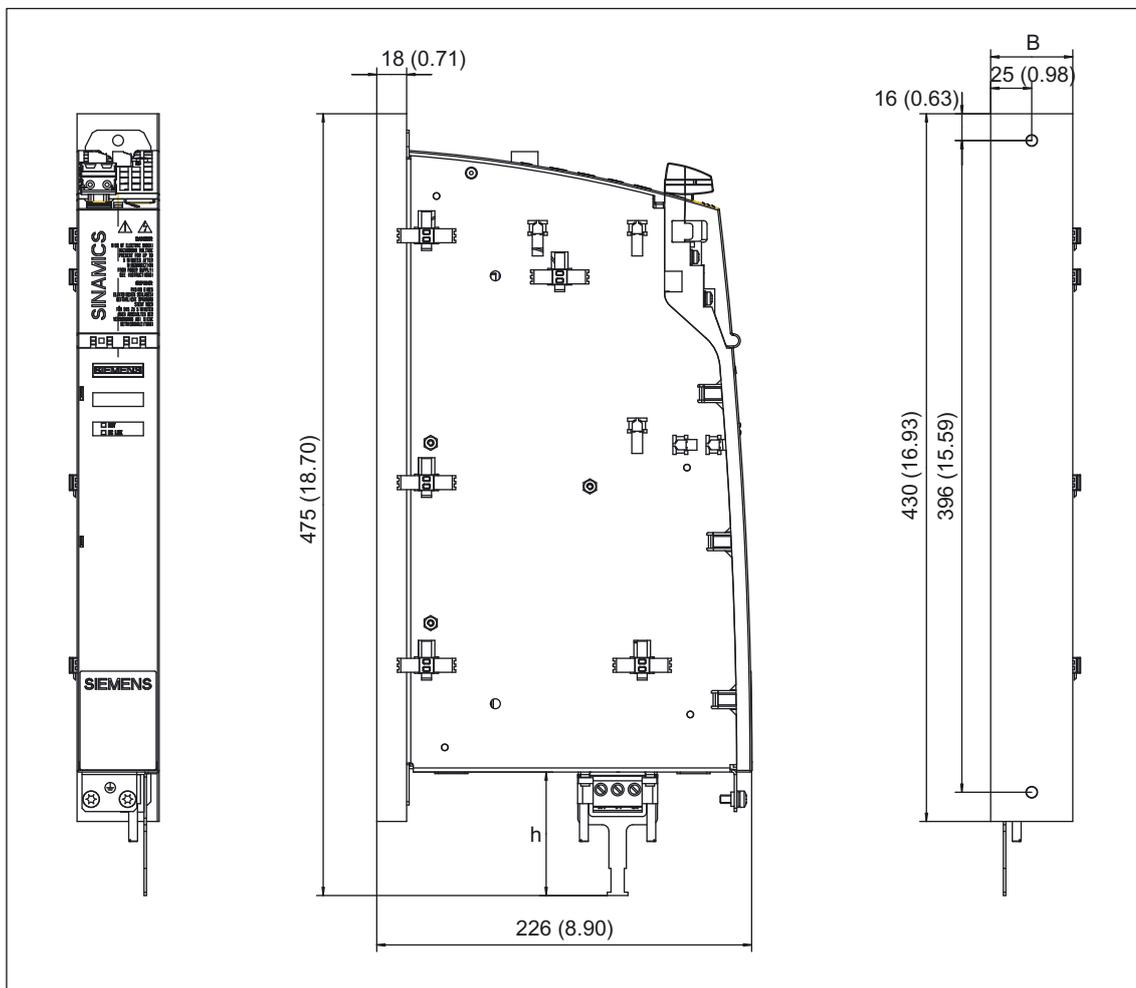
Figure 7-3 Dimension drawing, Smart Line Module with cold plate (5 kW and 10 kW)
