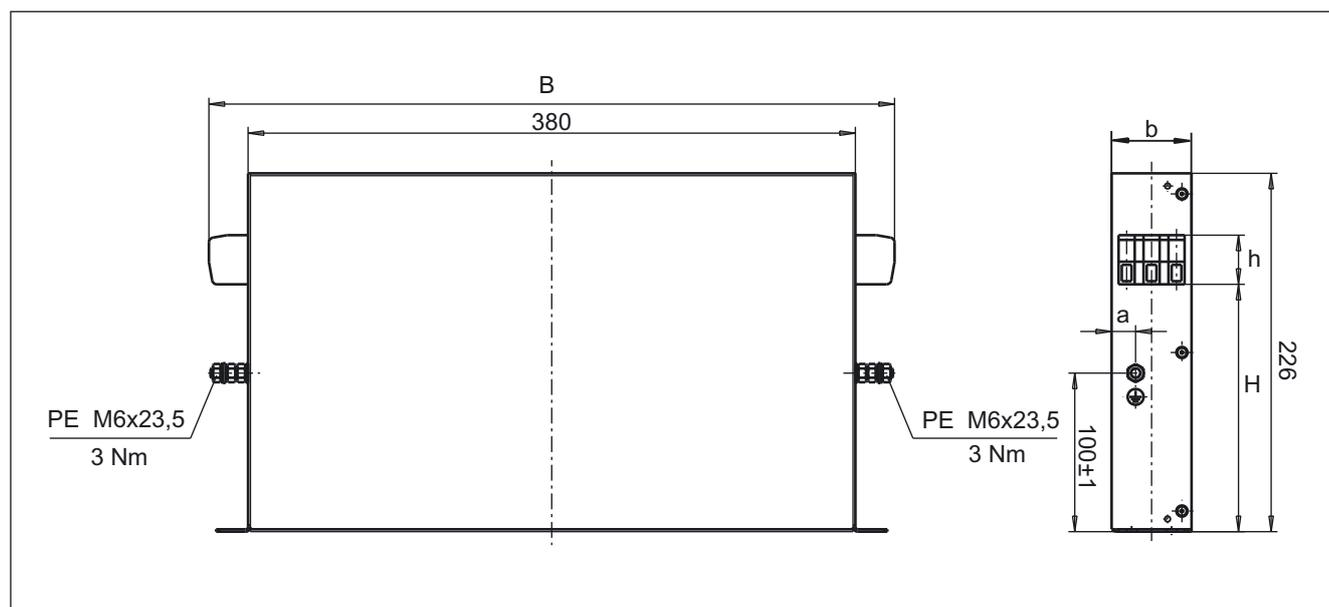
Figure 4-5 Dimension drawing: Basic Line Filter for Active Line Modules (16 kW to 55 kW)
