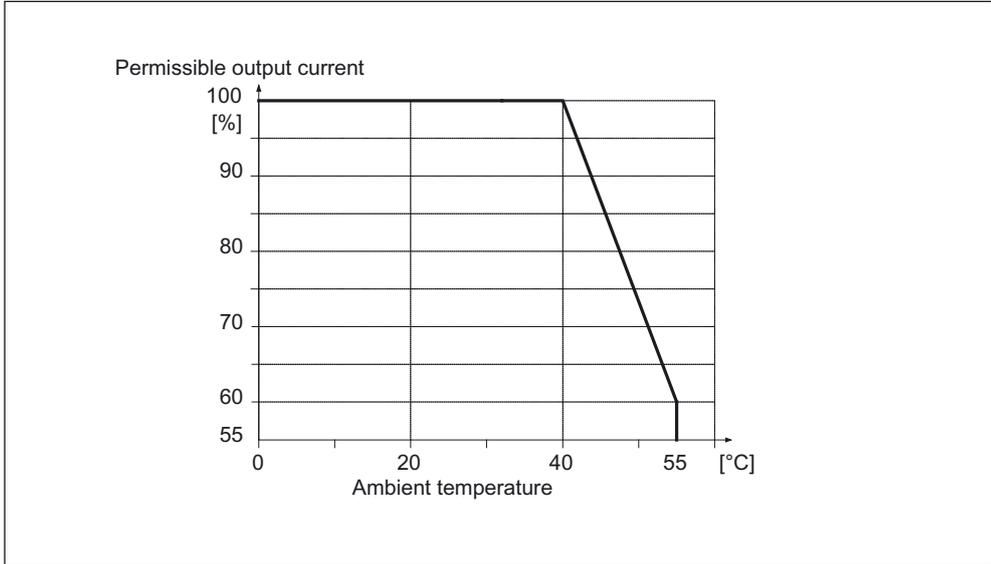
Figure 5-7 Derating as a function of the ambient temperature
