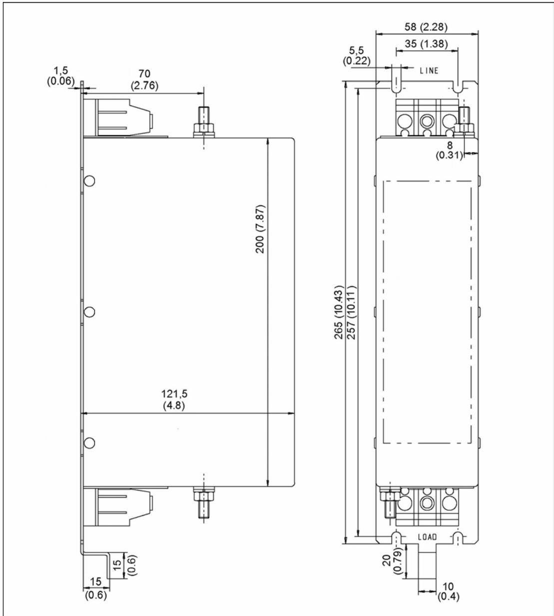
Figure 4-19 Dimension drawing: Basic Line Filter for Smart Line Modules (5 and 10 kW)
