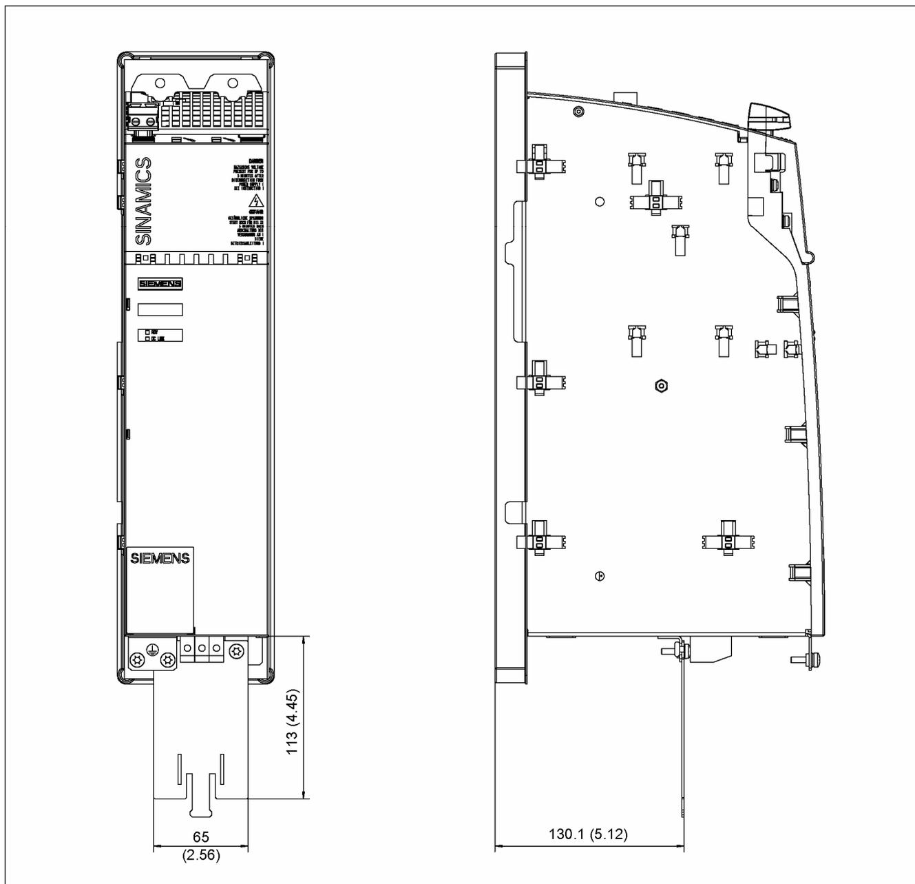
Figure 13-2 Dimension drawing, shield connecting plate on a 100 mm component with cold plate
