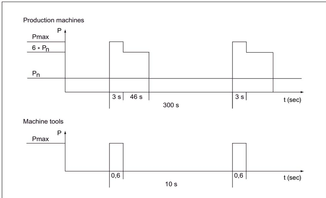
Figure 6-14 Braking duty cycle for 20 kW and 40 kW Basic Line Modules
