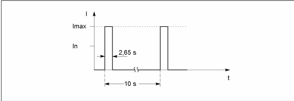
Figure 8-10 Peak current duty cycle without prior loading
