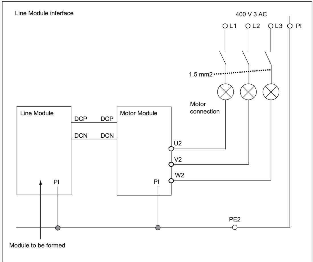
Figure 15-1 Line Module interface
