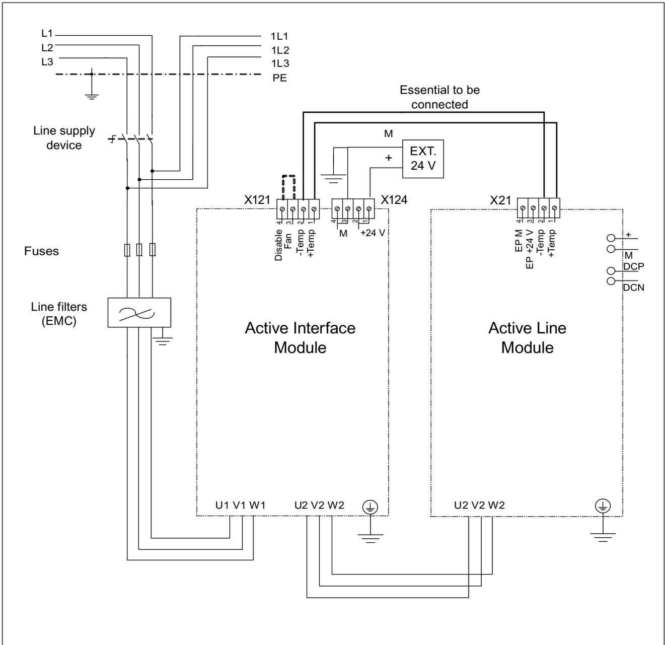
Figure 4-23 Connection example: Active Interface Module
