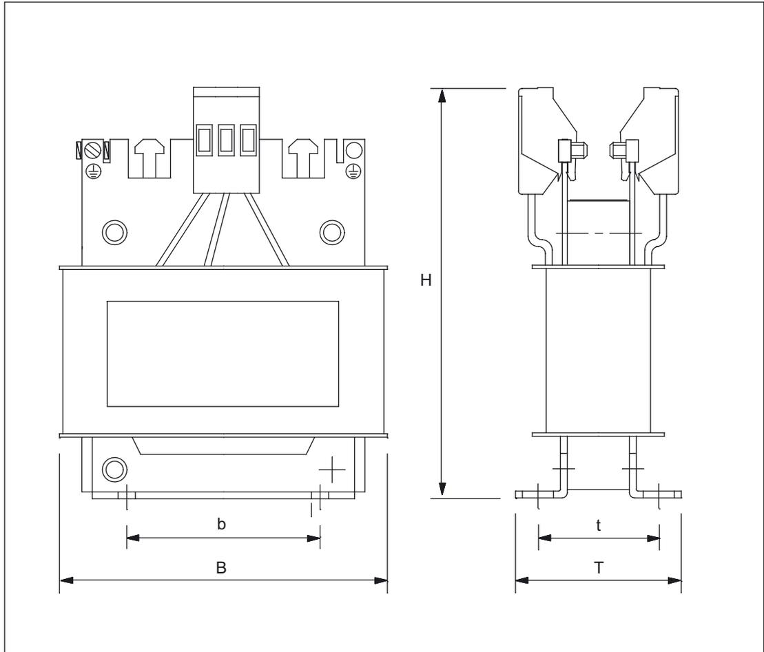
Figure 4-31 Dimension drawing: line reactor for Smart Line Modules (5 and 10 kW)
