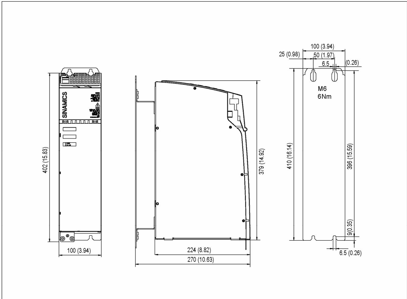
Figure 11-9 Dimension drawing of the capacitor module
