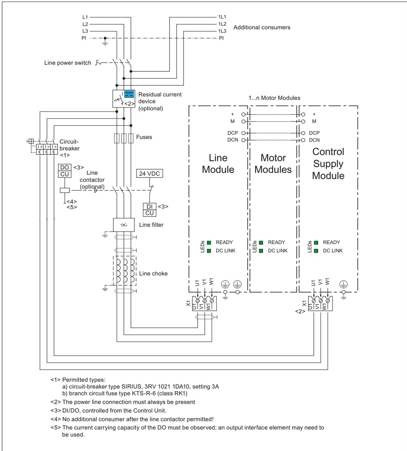
Figure 11-12 Example connection of Control Supply Module
