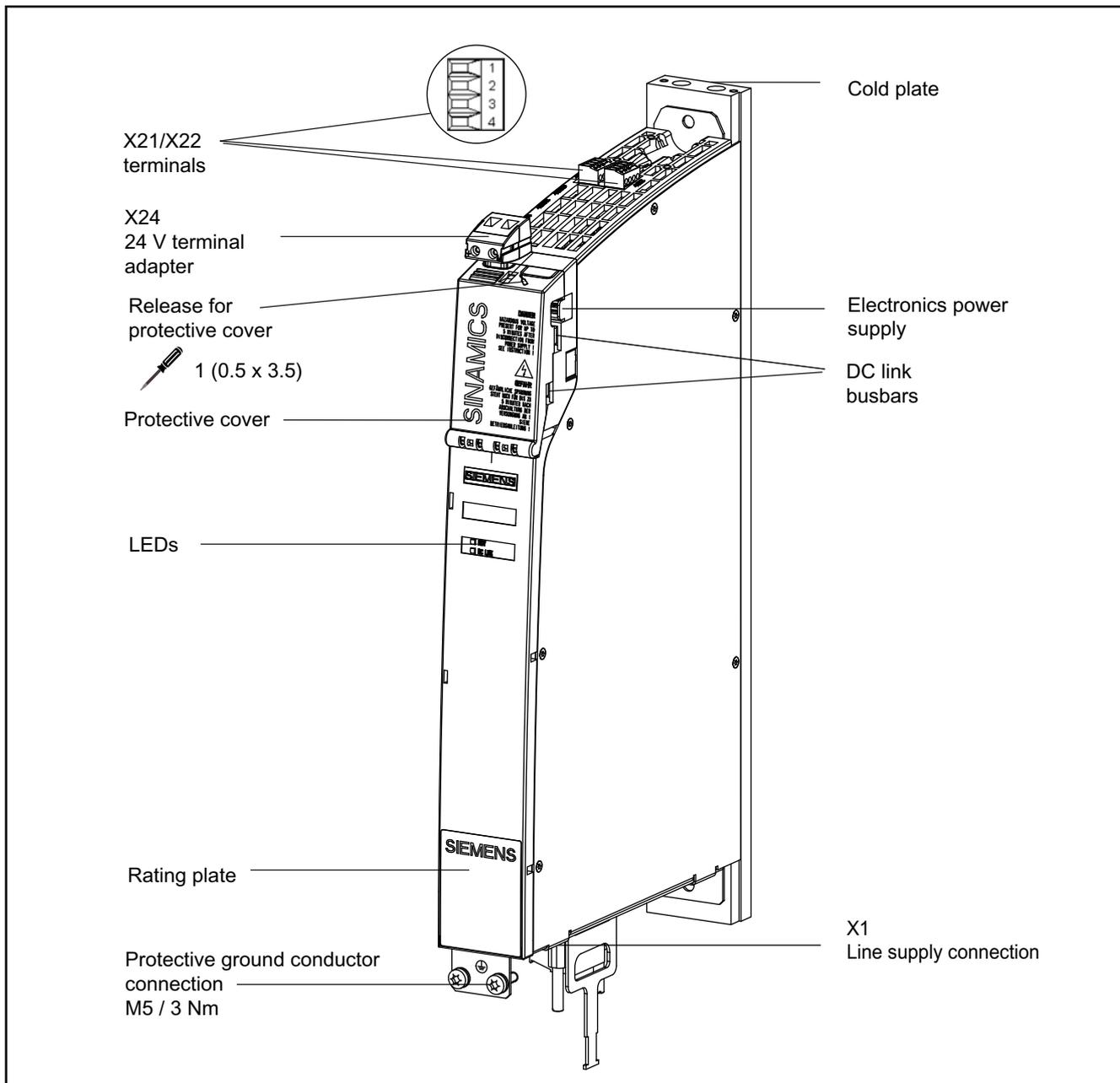
Figure 7-1 Smart line module with cold plate (10 kW)
