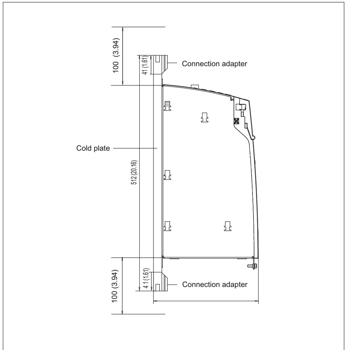
Figure 9-2 Space requirements for connection adapter
