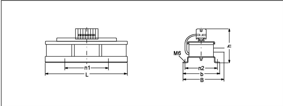
Figure 4-28 Dimension drawing: line reactor for Active Line Modules (up to 55 kW)
