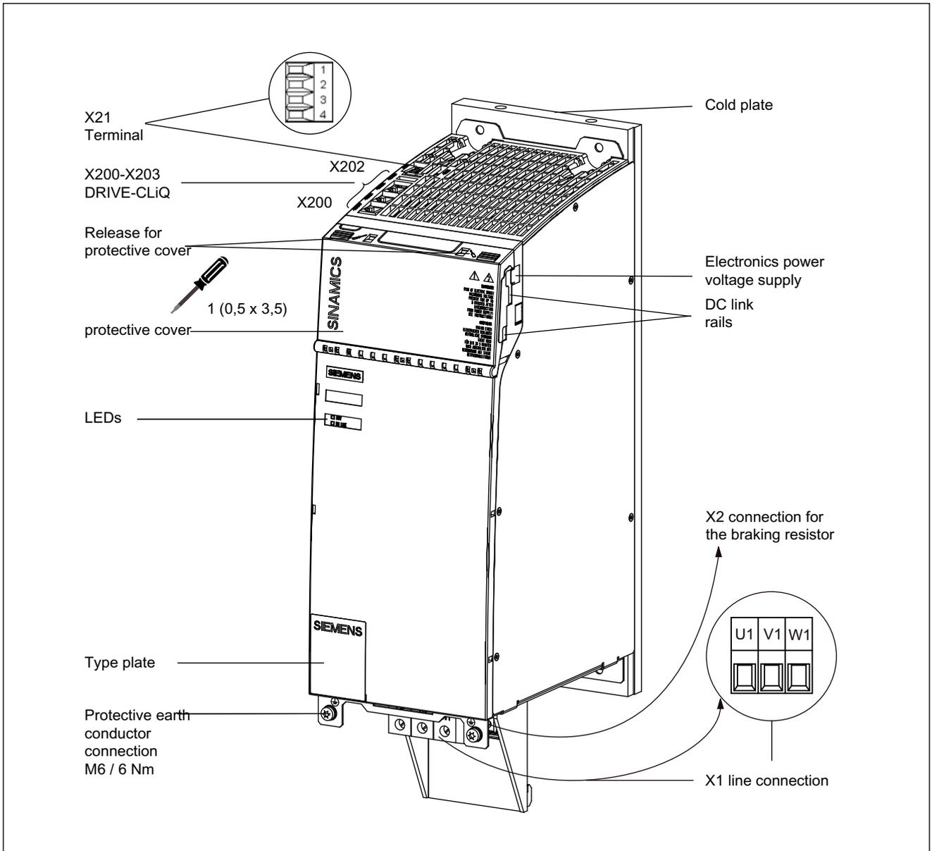
Figure 6-2 Interface description: Basic Line Module with cold-plate cooling (40 kW)
