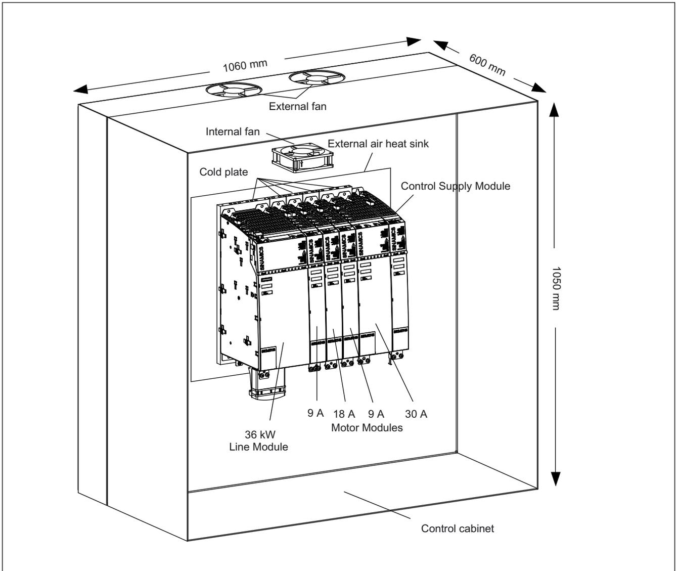
Figure 2-1 Example: cabinet setup with powers actions, cold plate, and external air heat sink
