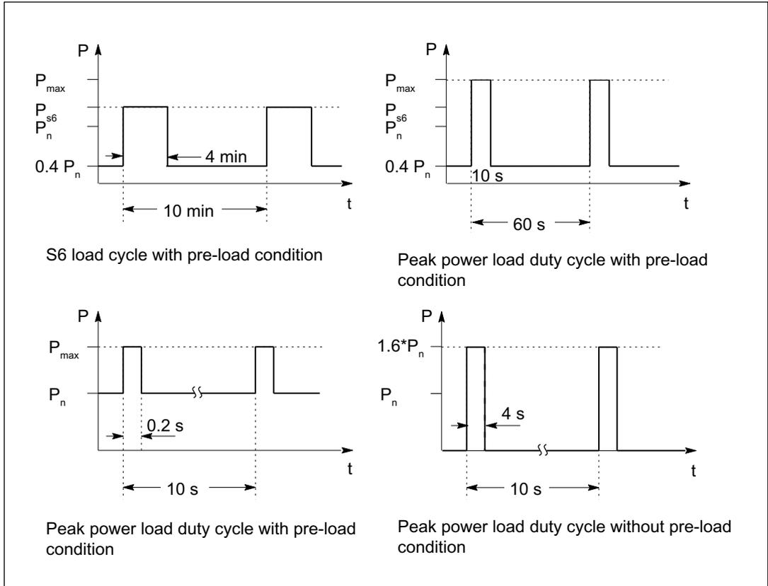
Figure 7-5 Rated duty cycles of Smart Line Modules
