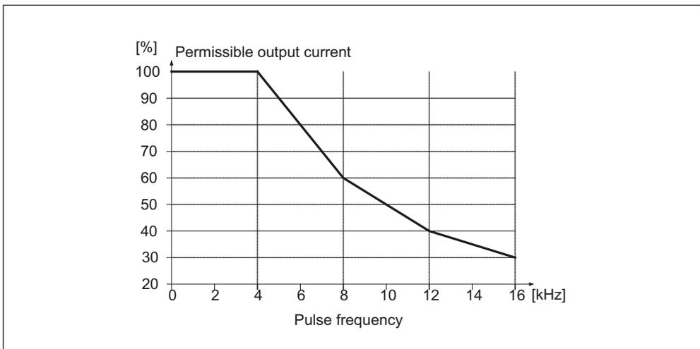
Figure 8-16 Derating as a function of the pulse frequency
