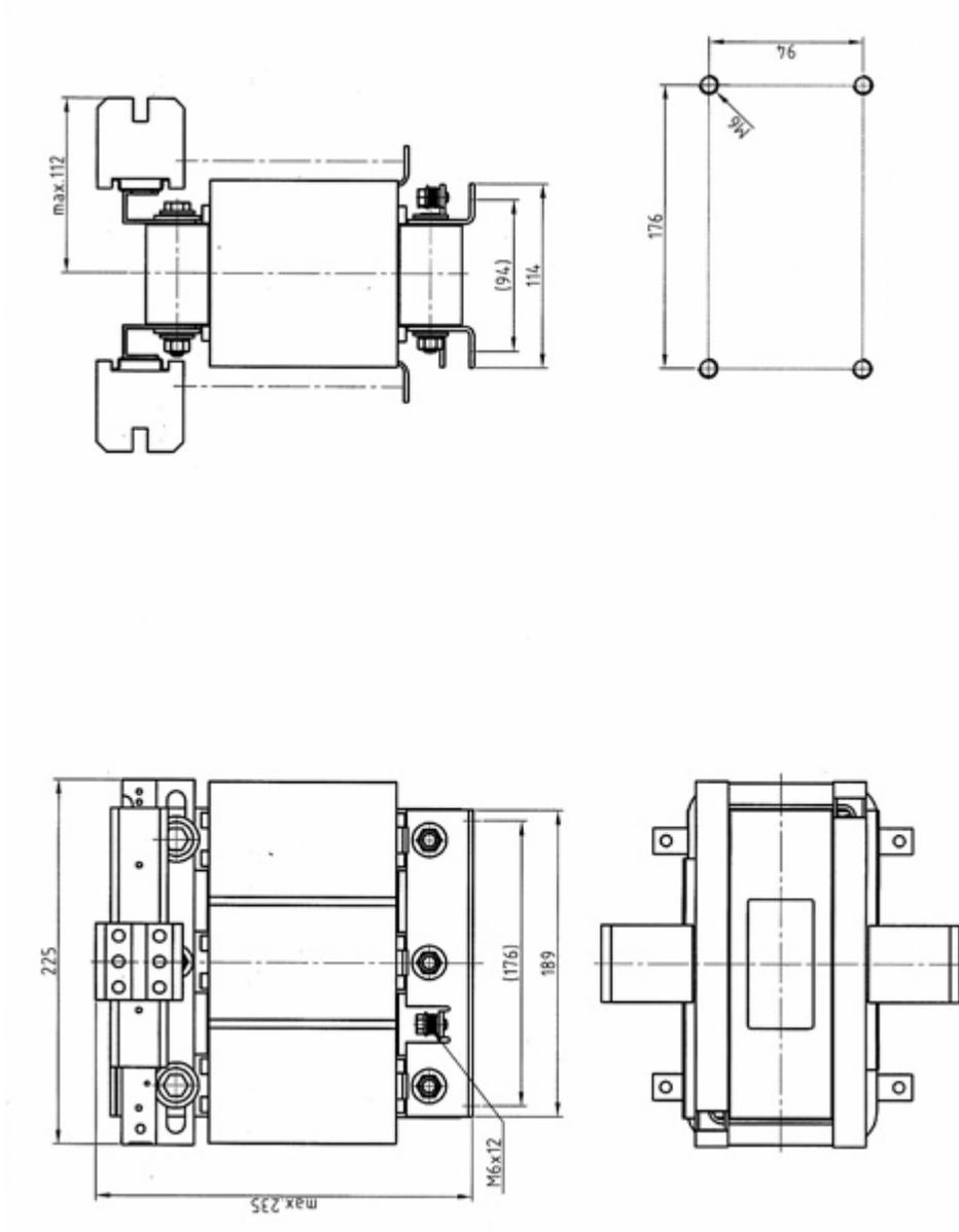
Figure 4-33 Dimension drawing of the line reactor for the Smart Line Module 36 kW
