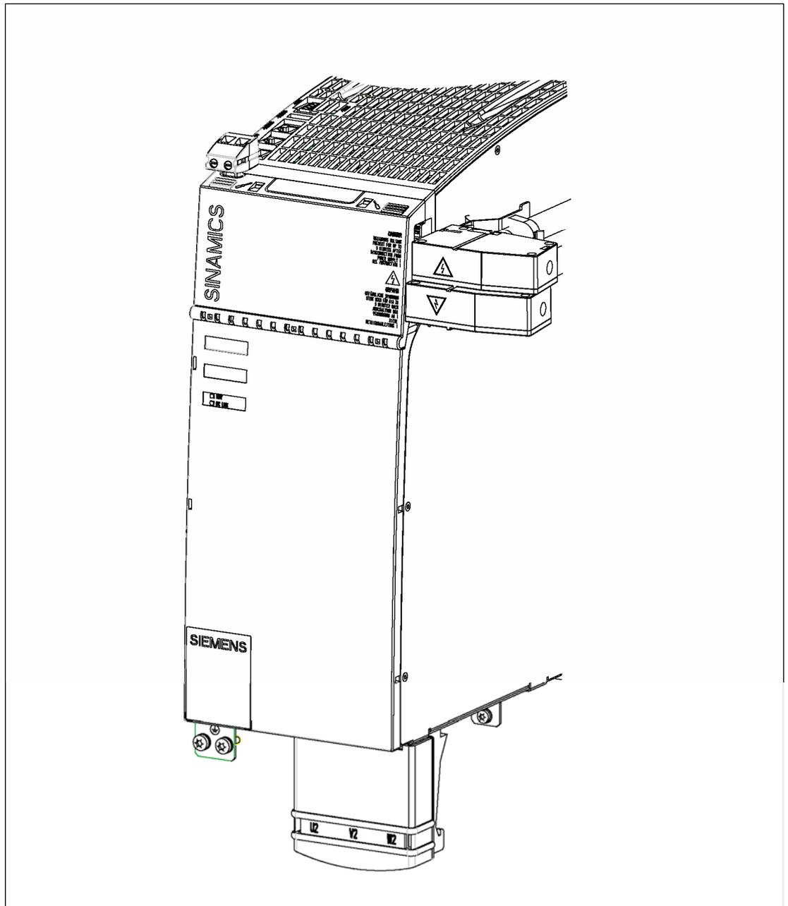
Figure 13-8 150 mm components with DC link adapter for two-row configuration 35 mm<sup>2</sup> to 95 mm<sup>2</sup>
