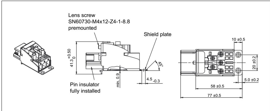
Figure 14-10 Dimensions: Power connector
