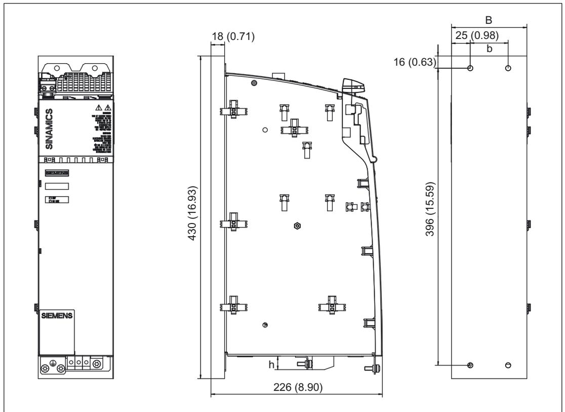
Figure 5-3 Dimension drawing, Active Line Module with cold plate (16 kW)
