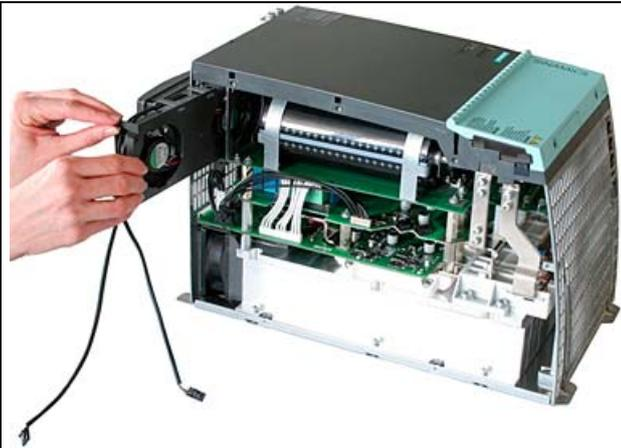
Completely pull out the fan module
