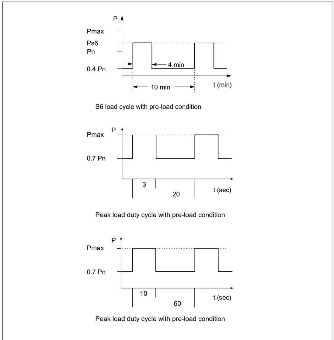
Figure 6-13 Infeed duty cycles for 100 kW Basic Line Module
