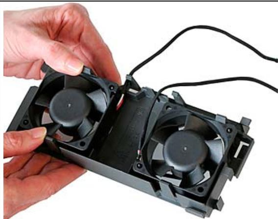
Slightly push the fan holder apart and pull out the fan
