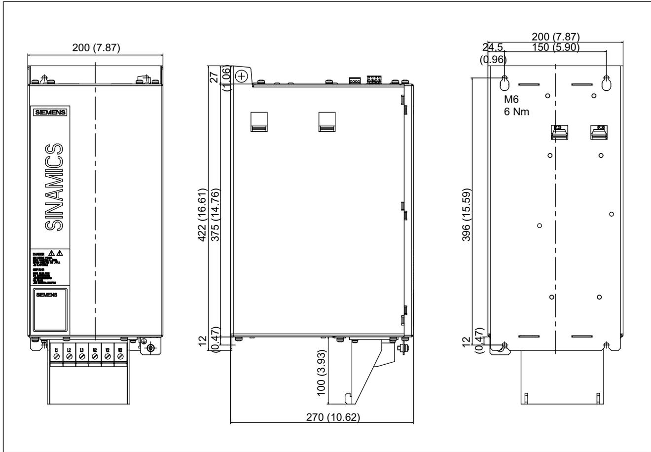
Figure 4-24 Dimension drawing: Active Interface Module 55 kW
