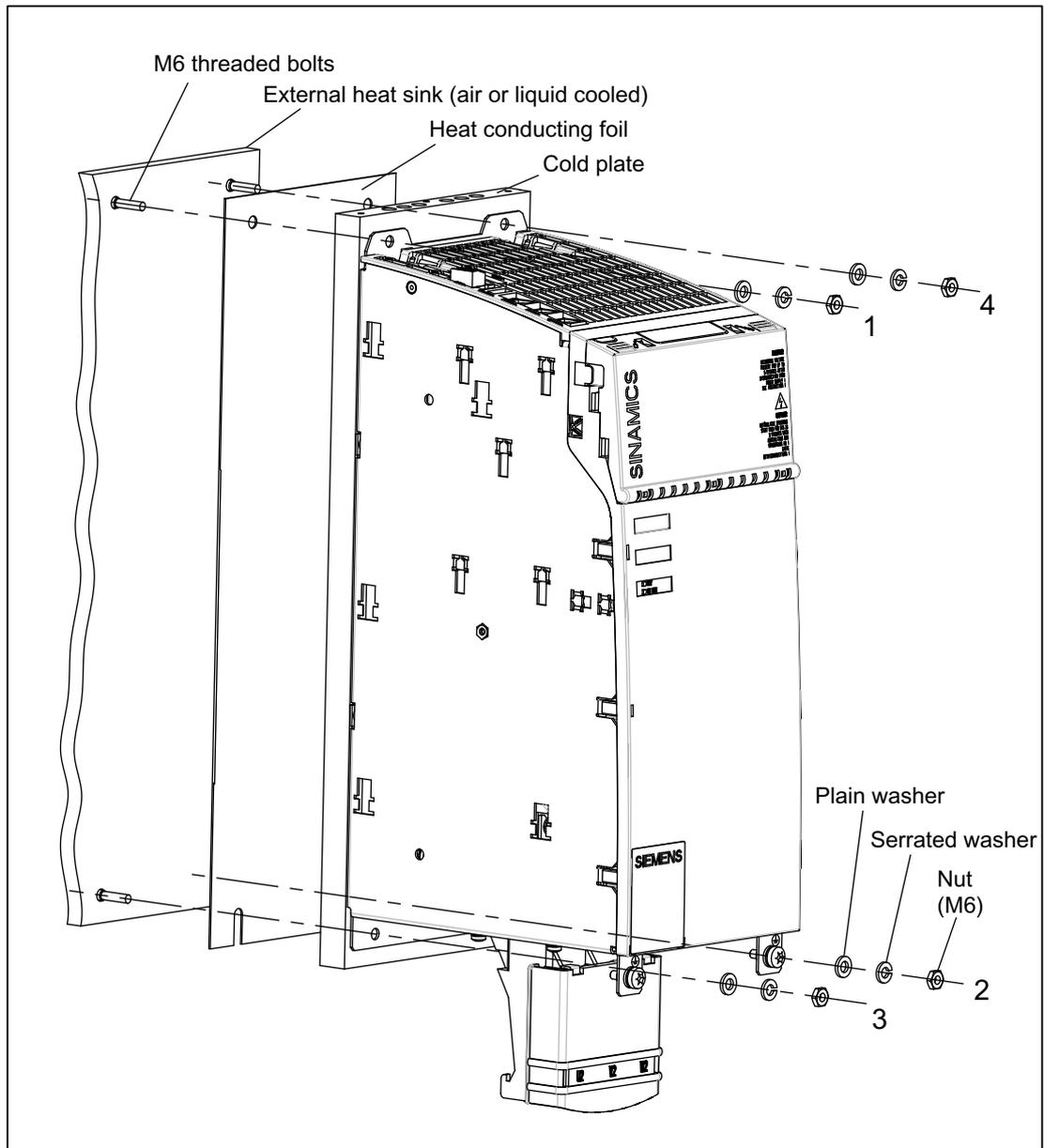
Figure 8-8 Installing a cold-plate power section with an external heat sink and heat-conducting film
