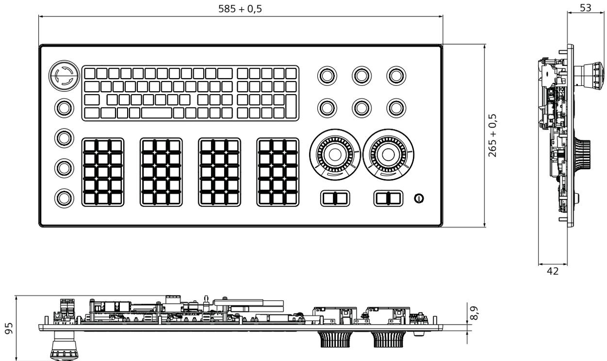
Figure 3-1 Front, rear and side view of MCP 2400 (all specifications in mm)
