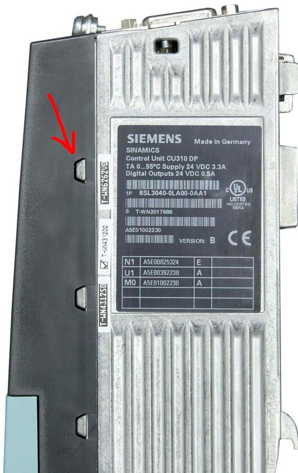
Figure 11-1 Lateral snap hooks on a CU310 DP
