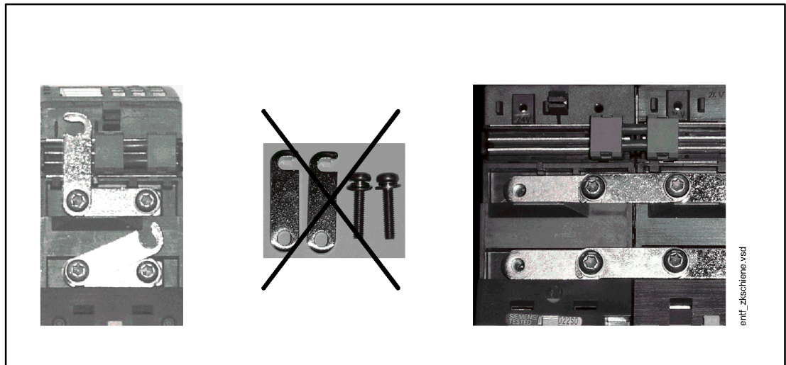
Figure 7-4 Removing the DC link bridges (two-tier arrangement)
