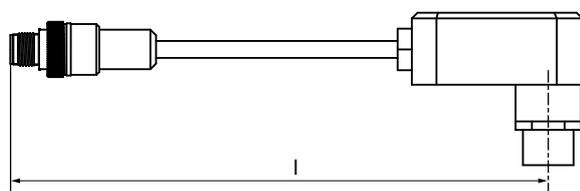
Figure 10-1 M12 connecting cable ↔ reader
