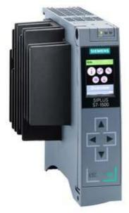
\*\*\*SPARE PART\*\*\* SIPLUS S7-1500 CPU 1511-1 PN -40...+70°C start up -20°C with conformal coating based on 6ES7511-1AK01-0AB0! To the left of the CPU, no module can be inserted! . Central processing unit with Work memory 150 KB for Program and 1 MB for data, 1st interface: PROFINET IRT with 2-port switch, 60 ns bit performance, SIMATIC Memory Card required
