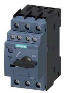
Circuit breaker size S0 for motor protection, CLASS 10 A-release 30...36 A N-release 432 A screw terminal Standard switching capacity with transverse auxiliary switches 1 NO+1 NC Reusable packaging Pack = 43 units
