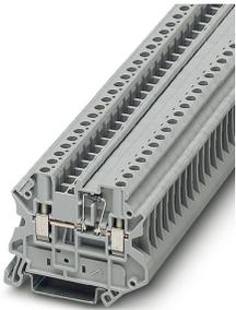
Component terminal block, with integrated diode, The max. current is determined by the diode. Installed: Diode 1N 4007, reverse voltage: 1300 V, maximum continuous current: 0.5 A., nom. voltage: 800 V, nominal current: 0.5 A, connection method: Screw connection, number of connections: 2, cross section: 0.14 mm<sup>2</sup> - 6 mm<sup>2</sup>, AWG: 26 - 10, width: 6.2 mm, color: gray, mounting type: NS 35/7,5, NS 35/15
