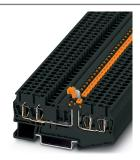
Knife disconnect terminal block, nom. voltage: 400 V, nominal current: 20 A, connection method: Spring-cage connection, cross section: 0.08 mm² - 4 mm², AWG: 28 - 12, length: 84 mm, width: 5.2 mm, color: black, mounting: NS 35/7,5, NS 35/15
