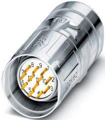
Cable connector, CA, straight, shielded: yes, SPEEDCON locking, M23, No. of pos.: 16, type of contact: Pin, Solder connection, cable diameter range: 4 mm ... 6 mm, coding:N
