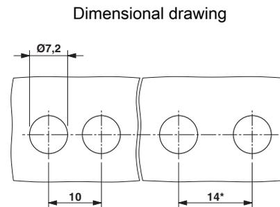
\* Dimensions when using the DP-VDFK 4/4 spacer plate
