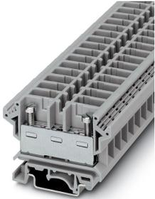
Feed-through terminal block, nom. voltage: 800 V, nominal current: 76 A, connection method: Screw connection, number of connections: 2, cross section: 0.5 mm<sup>2</sup> - 16 mm<sup>2</sup>, AWG: 20 - 6, width: 10.2 mm, color: gray, mounting type: NS 35/7,5, NS 35/15, NS 32
