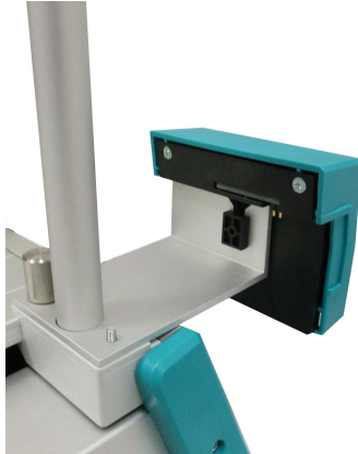
Figure 2-3 Positioning the lowering unit in the mounting bracket
