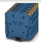
High-current terminal block, nom. voltage: 1000 V AC / 1500 V DC, nominal current: 232 A, connection method: Power-Turn connection, number of connections: 2, number of positions: 1, cross section: 25 mm<sup>2</sup> - 95 mm<sup>2</sup>, AWG: 4 - 4/0, width: 25 mm, color: blue, mounting type: NS 35/15
