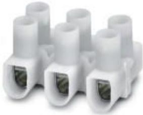
Europe terminal strip consisting of polypropylene, white, to connect solid and stranded conductors with and without ferrules with a cross section from 0.75 to 6 mm<sup>2</sup>, 3-pos.
