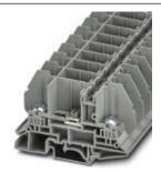
Feed-through terminal block with bolt connection, cross section: 0.1 - 6 mm², AWG: 26 - 10, width 16.3 mm, color: Grav
