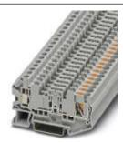
Disconnect terminal block, connection method: Push-in connection, Screw connection, cross section: 0.2 mm<sup>2</sup> - 6 mm<sup>2</sup>, AWG: 24 - 12, width: 6.2 mm, color: gray, mounting: NS 35/7,5, NS 35/15
