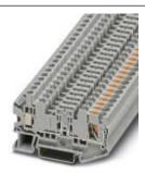
Disconnect terminal block, with test socket screws to accommodate 4 mm test plugs, connection method: Push-in connection, Screw connection, cross section: 0.2 mm² - 6 mm², AWG: 24 - 12, width: 6.2 mm, color: gray, mounting: NS 35/7,5, NS 35/15
