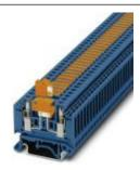
Knife disconnect terminal block, With test socket screws for insertion of test plugs, nom. voltage: 400 V, nominal current: 16 A, connection method: Screw connection, cross section: 0.2 mm² - 4 mm², AWG: 24 - 12, length: 46 mm, width: 5.2 mm, color: blue, mounting: NS 35/7,5, NS 35/15, NS 32
