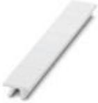
Zack marker strip, Strip, white, unlabeled, can be labeled with: PLOTMARK, CMS-P1-PLOTTER, mounting type: snap into tall marker groove, for terminal block width: 15.2 mm, lettering field size: 10.5 x 15.1 mm, Number of individual labels: 5
