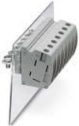
Panel feed-through terminal block, connection method: Screw connection with tension sleeve, Cable lug connection, number of positions: 1, load current: 101 A, cross section: 6 mm<sup>2</sup> - 35 mm<sup>2</sup>, connection direction of the conductor to plug-in direction: 0 °, width: 15.1 mm, color: gray
