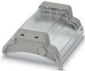
Cover profile, can optionally be sealed, length: 73.4 mm, width: 74.1 mm, height: 32 mm, color: transparent
