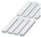
Marker for terminal blocks. Strip, white, labeled, can be labeled with: CMS-P1-PLOTTER, horizontal: L1, L2, L3, N, PE, L1, L2, L3, N, PE, mounting type: snap into tall marker groove, for terminal block width: 8.2 mm, lettering field size: 10.5 x 8.15 mm, Number of individual labels: 10
