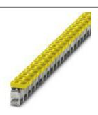
Connection terminal block, connection method: Screw connection, load current: 125 A, cross section: 2.5 mm² - 35 mm², width: 14.3 mm, color: yellow
