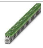
Connection terminal block, connection method: Screw connection, load current: 76 A, cross section: 1.5 mm<sup>2</sup> - 16 mm<sup>2</sup>, width: 9.8 mm, color: green
