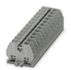
Feed-through terminal block with bolt connection method, cross section: 0.1 - 6 mm², AWG: 26 - 10, width 13 mm, color: gray
