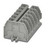
Feed-through terminal block with bolt connection method, cross section: 0.1 - 10 mm², AWG: 26 - 8, width 13 mm, color: gray
