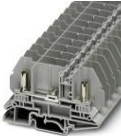
Test disconnect terminal block, cross section: 0.1 - 6 mm 2 , AWG: 26 - 8, width 13 mm, color: gray
