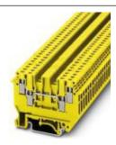
Feed-through terminal block, nom. voltage: 500 V, nominal current: 24 A, connection method: Screw connection, number of connections: 4, cross section: 0.2 mm² - 4 mm², AWG: 24 - 12, width: 5.2 mm, color: yellow, mounting type: NS 35/7,5, NS 35/15, NS 32
