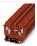
Feed-through terminal block, nom. voltage: 500 V, nominal current: 24 A, connection method: Screw connection, number of connections: 4, cross section: 0.2 mm² - 4 mm², AWG: 24 - 12, width: 5.2 mm, color: red, mounting type: NS 35/7,5, NS 35/15, NS 32
