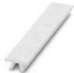
Zack marker strip, can be ordered: Strip, white, labeled according to customer specifications, mounting type: snap into tall marker groove, for terminal block width: 12.2 mm, lettering field size: 10.5 x 12.15 mm, Number of individual labels: 5
