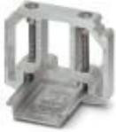
End clamp, for end support of UKH 50 to UKH 240, is pushed onto DIN rail NS 35 and fixed with 2 screws, width: 10 mm, color: aluminum
