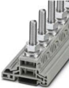
High Current Connectors, nom. voltage: 1000 V, nominal current: 269 A, connection method: Bolt connection, number of connections: 1, width: 32 mm, height: 74.6 mm, color: gray, mounting type: NS 35/7,5, NS 35/15
