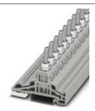
High Current Connectors, nom. voltage: 1000 V, nominal current: 76 A, connection method: Bolt connection, number of connections: 1, width: 13 mm, height: 56.1 mm, color: gray, mounting type: NS 35/7,5, NS 35/15
