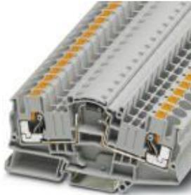
Component terminal block, with integrated BY255 diode, connection method: Push-in connection, cross section: 0.5 mm<sup>2</sup> - 10 mm<sup>2</sup>, AWG: 20 - 10, width: 8.2 mm, color: gray
