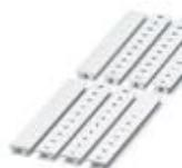
Zack marker strip, Strip, white, labeled, can be labeled with: CMS-P1-PLOTTER, printed horizontally: consecutive numbers 1 ... 10, 11 ... 20, etc. up to 91 ... 100, mounting type: snap into tall marker groove, for terminal block width: 8.2 mm, lettering field size: 10.5 x 8.15 mm, Number of individual labels: 10
