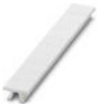
Zack marker strip, Strip, white, unlabeled, can be labeled with: CMS-P1-PLOTTER, PLOTMARK, mounting type: snap into tall marker groove, for terminal block width: 8.2 mm, lettering field size: 10.5 x 8.15 mm, Number of individual labels: 10
