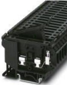
Fuse modular terminal block, fuse type: Glass / ceramics / ..., number of positions: 1, connection method: Screw connection, cross section: 0.2 mm<sup>2</sup>- 4 mm<sup>2</sup>, AWG: 24 - 12, nominal current: 6.3 A, nom. voltage: 800 V, width: 8.2 mm, fuse type: G / 5 x 20 / 5 x 25 / 5 x 30, mounting type: NS 35/7,5, NS 35/15, NS 32, color: black
