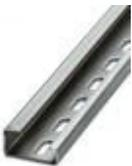
DIN rail perforated, G profile, width: 32 mm, height: 15 mm, acc. to EN 60715, material: Steel, galvanized, passivated with a thick layer, length: 2000 mm, color: silver
