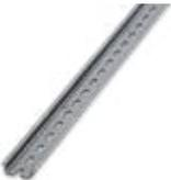
DIN rail perforated, Standard profile, width: 35 mm, height: 7.5 mm, acc. to EN 60715, material: Steel, Galvanized, white passivated, length: 2000 mm, color: silver
