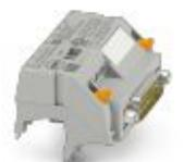
V8 adapter for 8 x PLC-INTERFACE (6.2 mm), controller: PLC system cabling of output cards, connection 1: Screw connection 1x, connection 2: D-SUB pin strip 1x 15-position, connection 3: Plug connection (Can be snapped onto 8x PLC-INTERFACE terminals), number of channels: 8, control logic: positive switching
