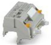
V8 adapter for 8 x PLC-INTERFACE (6.2 mm), controller: PLC system cabling of output cards, connection 1: Screw connection 1x, connection 2: IDC/FLK pin strip 1x 14-position, connection 3: Plug connection (Can be snapped onto 8x PLC-INTERFACE terminals), number of channels: 8, control logic: positive switching
