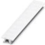
Zack marker strip, can be ordered: Strip, white, labeled according to customer specifications, mounting type: snap into tall marker groove, for terminal block width: 6.2 mm, lettering field size: 6.15 x 10.5 mm, Number of individual labels: 10
