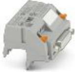
V8 adapter for 8 x PLC-INTERFACE (6.2 mm), controller: PLC system cabling of output cards, connection 1: Screw connection 1x, connection 2: D-SUB socket strip 1x 15-position, connection 3: Plug connection (Can be snapped onto 8x PLC-INTERFACE terminals), number of channels: 8, control logic: positive switching
