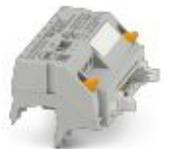
V8 adapter for 8 x PLC-INTERFACE (6.2 mm), controller: PLC system cabling of output cards, connection 1: Screw connection 1x, connection 2: IDC/FLK pin strip 1x 14-position, connection 3: Plug connection (Can be snapped onto 8x PLC-INTERFACE terminals), number of channels: 8, control logic: negative switching
