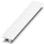
Zack marker strip, Strip, white, unlabeled, can be labeled with: PLOTMARK, CMS-P1-PLOTTER, mounting type: snap into tall marker groove, for terminal block width: 6.2 mm, lettering field size: 6.15 x 10.5 mm, Number of individual labels: 10
