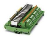
16-channel relay module for Honeywell C300 output modules. The module is controlled by the control system via 37-pos. D-SUB or 50-pos. FLK. A screw connection with knife disconnection is available in the field. Module width: 227 mm
