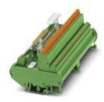
16-channel module for Honeywell C300 modules. The module is controlled by the control system via 37-pos. D-SUB or 50-pos. FLK. A spring-cage connection (1+, 1-,...16+,16-) with knife disconnection is provided in the field. Module width: 254 mm
