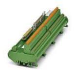
16-channel module for Honeywell C300 modules. On the control side, the module is controlled via D-SUB 37-pos. or FLK 50-pos. A screw connection (1+, 1C, 1-,...16+, 16C, 16-) with knife disconnection is available on the field side. Module width: 258.5 mm
