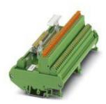
16-channel module with LED for Honeywell C300 modules. The module is controlled by the control system via 37-pos. D-SUB or 50-pos. FLK. A spring-cage connection (1+, 1-,...16+,16-) with knife disconnection is provided in the field. Module width: 170 mm
