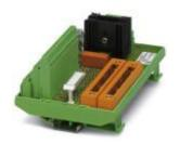
16-channel digital input module with screw connection and redundant voltage supply. Suitable for Yokogawa SDV 144 card
