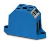
Device terminal block, nom. voltage: 1000 V, nominal current: 57 A, connection method: Screw connection, number of connections: 4, number of positions: 1, cross section: 0.5 mm² - 16 mm², AWG: 20 - 6, width: 71.3 mm, height: 40 mm, color: blue, mounting type: direct screw connection
