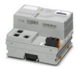
Axiocontrol for the direct control of Axioline F I/Os. With 3 Ethernet interfaces for the additional connection of distributed I/Os via PROFINET, Modbus TCP or TCP/IP. Programming according to IEC 61131-3. Includes connector plug and marking field.
