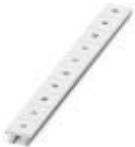
Marker for terminal blocks, Strip, white, labeled, can be labeled with: CMS-P1-PLOTTER, horizontal: U, V, W, N, GND, U, V, W, N, GND, mounting type: snap into tall marker groove, for terminal block width: 10.2 mm, lettering field size: 10.15 x 10.5 mm, Number of individual labels: 10
