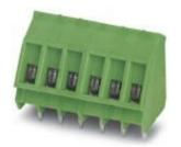
PCB terminal block, nominal current: 24 A, rated voltage (III/2): 400 V, nominal cross section: 2.5 mm², pitch: 5 mm, number of positions: 15, connection method: Screw connection with tension sleeve, mounting: Wave soldering, conductor/PCB connection direction: 55 °, color: green, Pin layout: Linear pinning, Solder pin [P]: 4.5 mm
