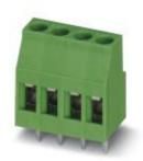
PCB terminal block, nominal current: 24 A, rated voltage (III/2): 400 V, nominal cross section: 2.5 mm², pitch: 5 mm, number of positions: 4, connection method: Screw connection with tension sleeve, mounting: Wave soldering, conductor/PCB connection direction: 0 °, color: green, Pin layout: Linear pinning, Solder pin [P]: 3.6 mm. The article can be aligned to create different nos. of positions!
