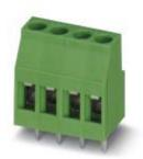
PCB terminal block, nominal current: 24 A, rated voltage (III/2): 400 V, nominal cross section: 2.5 mm², pitch: 5 mm, number of positions: 3, connection method: Screw connection with tension sleeve, mounting: Wave soldering, conductor/PCB connection direction: 0 °, color: green, Pin layout: Linear pinning, Solder pin [P]: 3.6 mm. The article can be aligned to create different nos. of positions!
