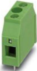
PCB terminal block, nominal current: 41 A, rated voltage (III/2): 320 V, nominal cross section: 4 mm<sup>2</sup>, pitch: 7.5 mm, number of positions: 1, connection method: Screw connection with tension sleeve, mounting: Wave soldering, conductor/PCB connection direction: 0 °, color: green, Pin layout: Linear pinning, Solder pin [P]: 5 mm
